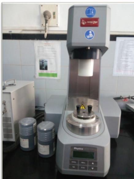
**Fig. 7.4** Controlled-Stress Rheometer
