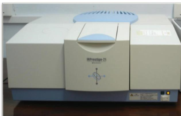
**Fig. 8.4** Fourier-transform infrared spectroscope
