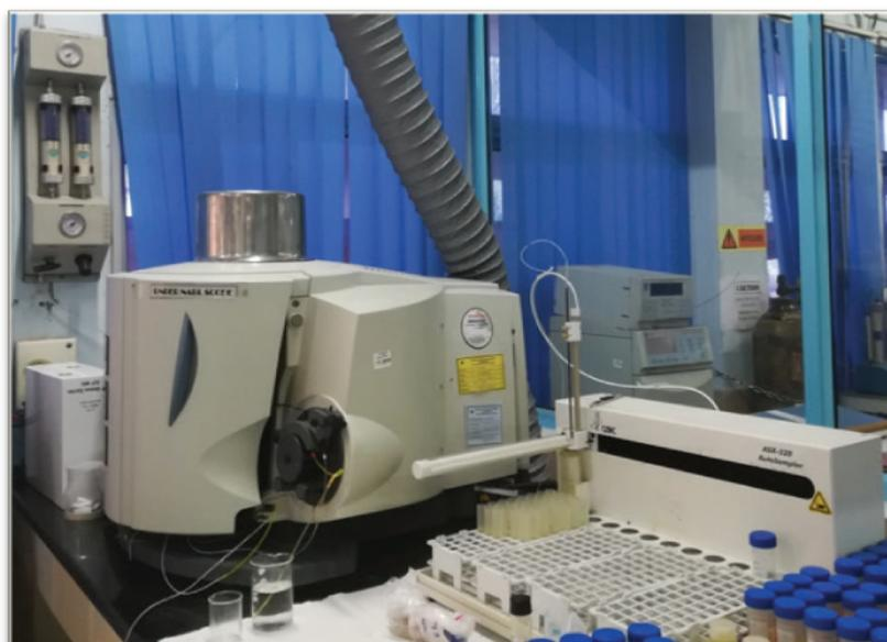
**Fig. 6.3** Inductivity Coupled Plasma–Optical Emission Spectrometer
