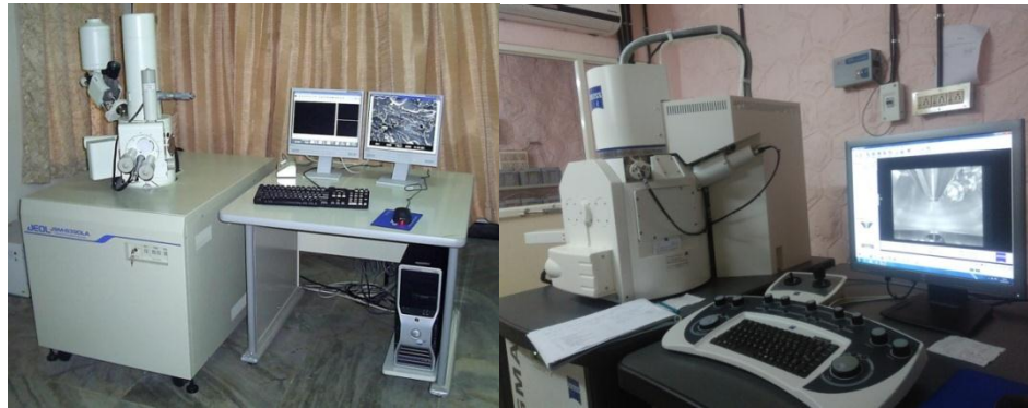
Fig.2.4 JEOL JSM-6390 LV Model Scanning Electron Microscope (SEM) and Carl Zeiss, sigma HV model Field emission scanning electron microscopy (FE-SEM) used for sample analysis
