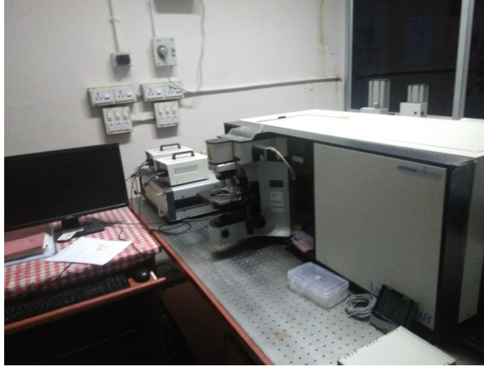
Fig.2.3 Horiba Jobin Yuon LabRAM HR system with a resolution in the order of 3\text{ cm}^{-1} equipped with He-Ne laser (632.8 nm)
