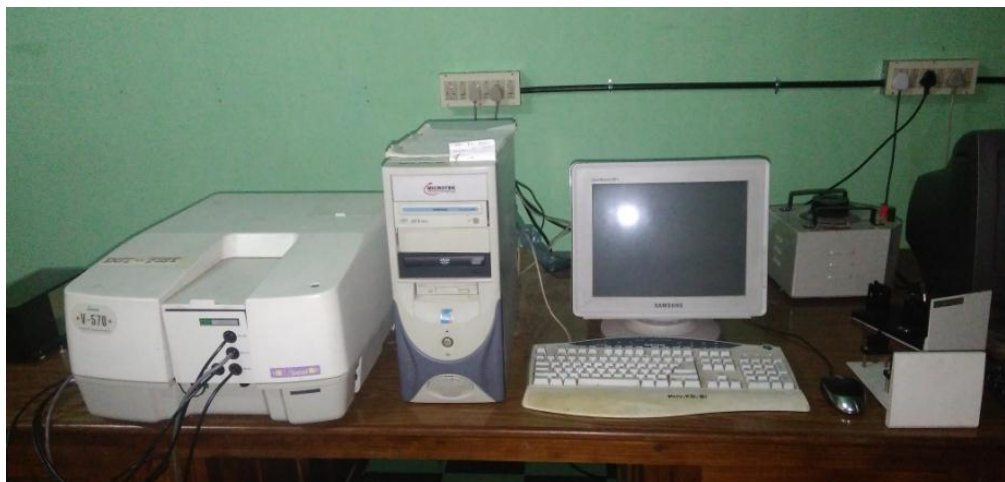
Fig.2.6 JASCO V 570 UV-Vis NIR spectrometer used for sample analysis
