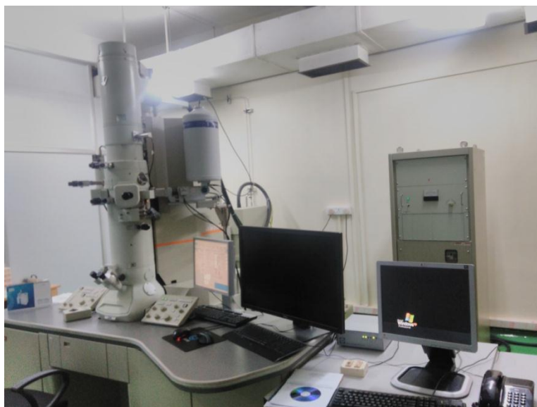
Fig.2.5 A JEOL JEM 2100 model advanced analytical High Resolution Transmission Electron Microscope (HRTEM) operated at 200 KeV attached with EDAX set up used for sample analysis in the present study.
