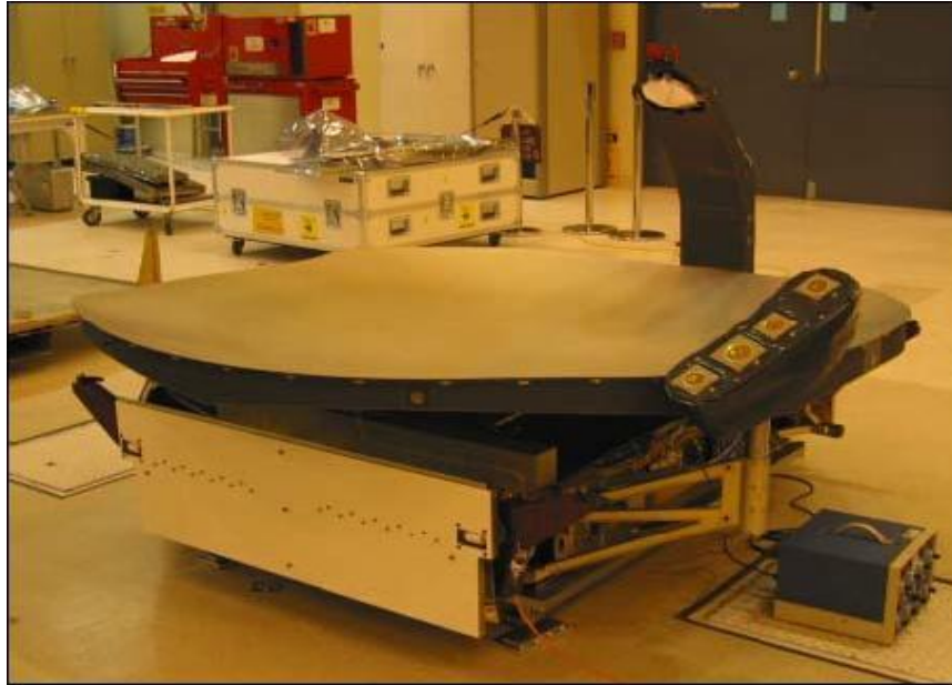
Figure 2.4: CPR Antenna Subsystem flight model (Adapted from Im et al. , 2005).
