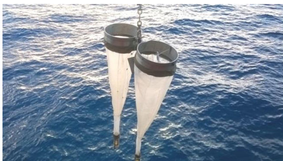
Figure 15. Operation of Bongo net onboard FORV Sagar Sampada during April 2015
