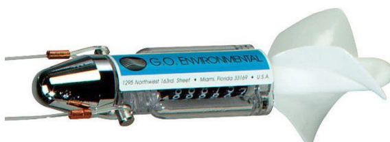
Figure 14. Flowmeter used for the study (General Oceanics 2030R with a standard rotor).
