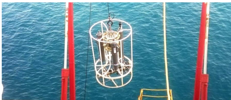
Figure 12. Operation of CTD, Sea-Bird Electronics Model 911 series onboard FORV Sagar Sampada .
