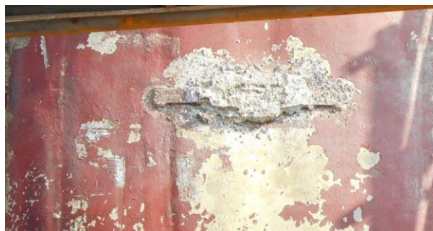
f) Fully consumed sacrificial anode on a ship's hull
