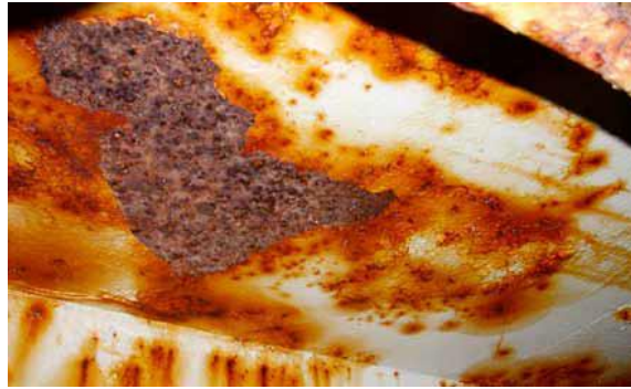
a) Corrosion of outer hull
