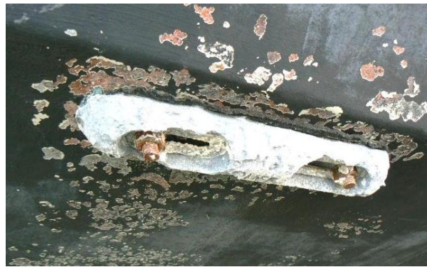
e) Ineffective sacrificial anode on a ship's hull
