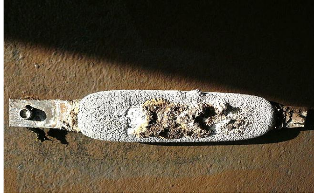
d) Sacrificial anodes on a ship's hull being consumed ( https://en.wikipedia.org )
