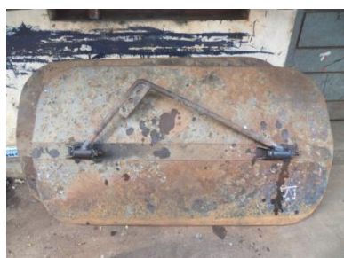
View of dorsal side of steel otterboard
