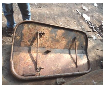
View of ventral side of steel otterboard
