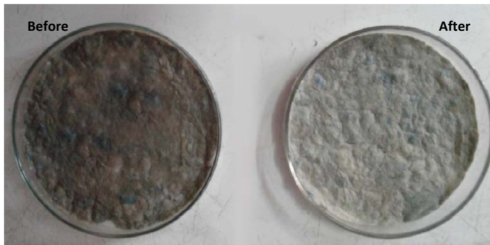
Fig 5.13. Manually pressed pulp before and after treatment with xylanase
