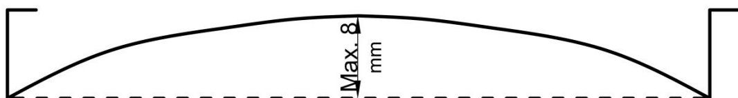
Fig. 3.5. Buckling Shaped Deflection of Plate between Stiffeners (Source: IACS (2013))
