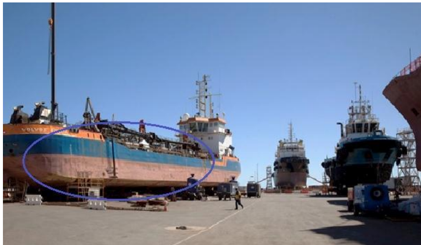
Fig. 3.2: HHD on the Port Side Shell Plating
