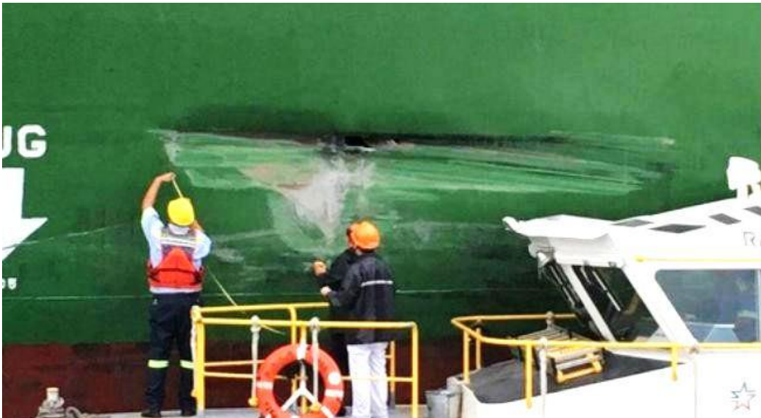
Fig. 2.5: Allision Casualty of Containership Xin Fei Zhou with the Wall of a New Dock Agua Clara on the Atlantic Side of the Panama Canal (Source: https://www.fleetmon.com/media/maritimeneews/xinfei.jpg accessed on 10 December 2017)
