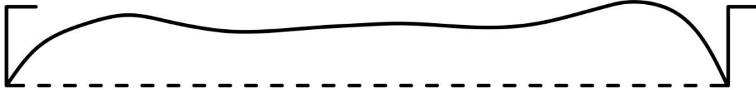
Fig. 3.3: Schematic Representation of Hungry Horse Shape Deflection (Source: Jiang and Soares 2013)
