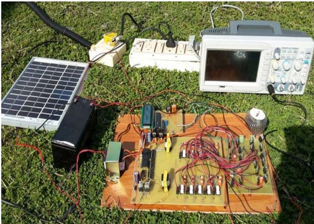
Figure 6.18: Hardware Set Up of the Proposed Converter for Harnessing Solar Energy
