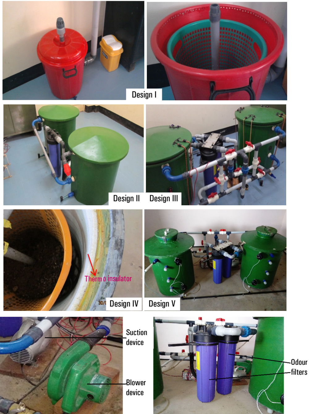
Figure 2.1: Photograph of sequence of developments of novel in-vessel composter
