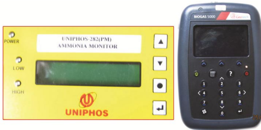
Figure 3.1: Photograph of 1) UNIPHOS 282-PM ammonia detector and 2) BIOGAS 5000
