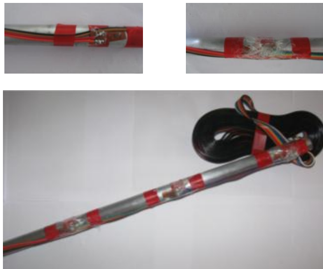
Fig. 3.8 Model Pile instrumented with Strain Gauge
