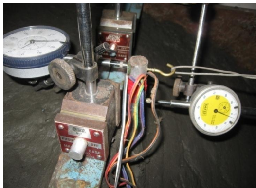
Fig. 3.15 Dial Gauges fixed at top of the pile and at the ground level
