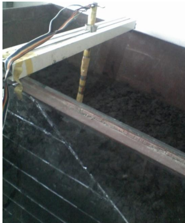
Fig. 3.13 Packing of soil in 10 cm layers
