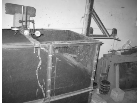
Fig. 3.14 Soil Packed in the Tank
