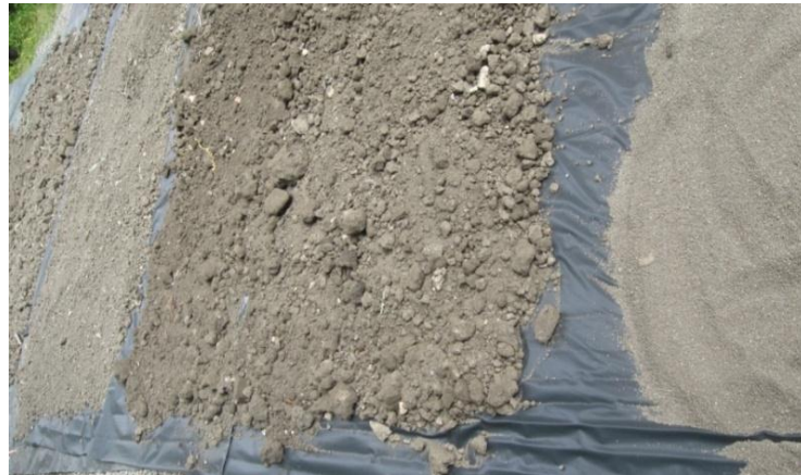
Fig. 3.4 Sundrying and powdering of soil sample
