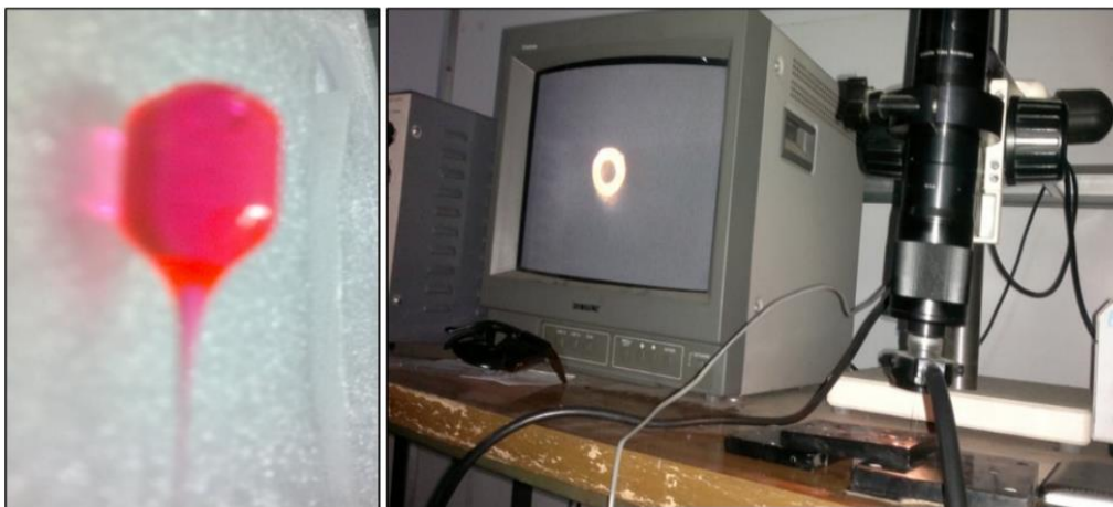
Figure 3.12 Dye doped PMMA preform after the fiber is drawn and enlarged cross sectional view of Rh6G-hollow POF using a CCD camera
