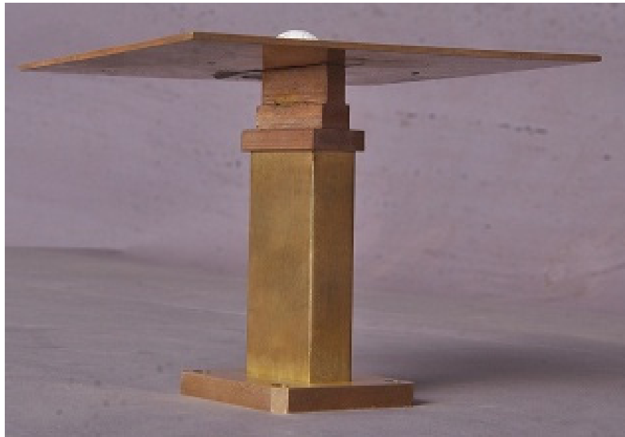
Fig. 3.16 Photograph of the fabricated double step junction coupled waveguide fed HDRA with 2t1 = 4.0 mm, 2t2 = 8.0 mm, 2t3 = 1.3 mm, 2W1 = 6.5 mm, 2W2 = 3.4 mm, 2W3 = 1.0 mm, 2L3 = 9.5 mm, x_{w3} = y_{w3} = 0 mm, a_{dr} = 7.5 mm, and \epsilon_r = 9.8 .
