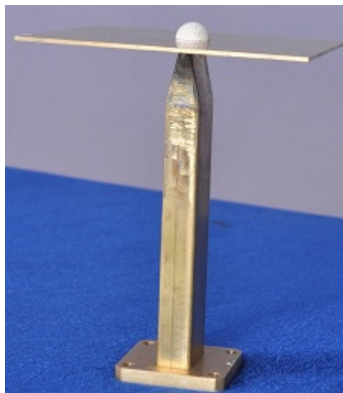
Fig. 4.9 Photograph of the rectangular waveguide fed HDRA using tapered waveguide section with sl = 9.0 mm, sw = 0.7 mm, tp = 21.0 mm, \theta = 13^\circ , a_{dr} = 6.27 mm and \epsilon_r = 9.8 .
