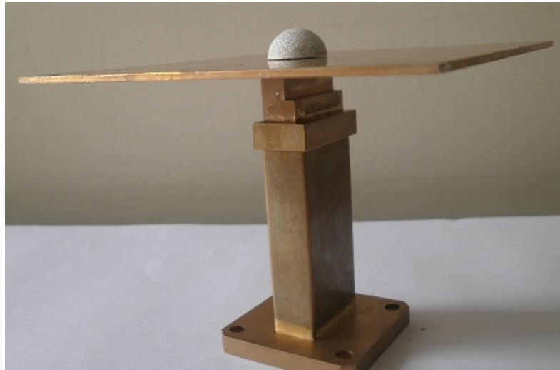
Fig. 5.15 Photograph of the fabricated stair shaped waveguide fed DRA with sl = 10.1 mm, sw = 0.8 mm, st = 1.3 mm, x_w = 0.0 mm, w_l = 7.0 mm, t_l = 5.5 mm, w_2 = 4.3 mm and t_2 = 9.2 mm.
