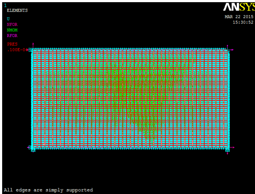
Figure 4.3. Model of plate used for laminate bending (CFRP-VE) in which all the edges are simply supported(AE-SS)
