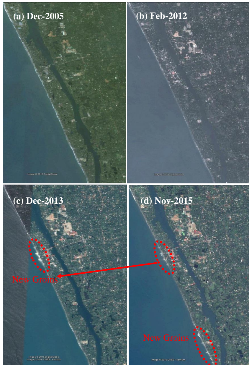
Fig. 6.24 Google images of the north central sector of Chavara coast: (a) 2005, no groins are available; (b) 2012, no groins are available; (c) 2013, a groin field of 4 nos. is seen and (d) 2015, another groin field consisting of 7groins is added
