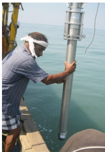
Fig. 3.17 Piston Corer being lowered for collection of sediment core from offshore of Chavara coast
