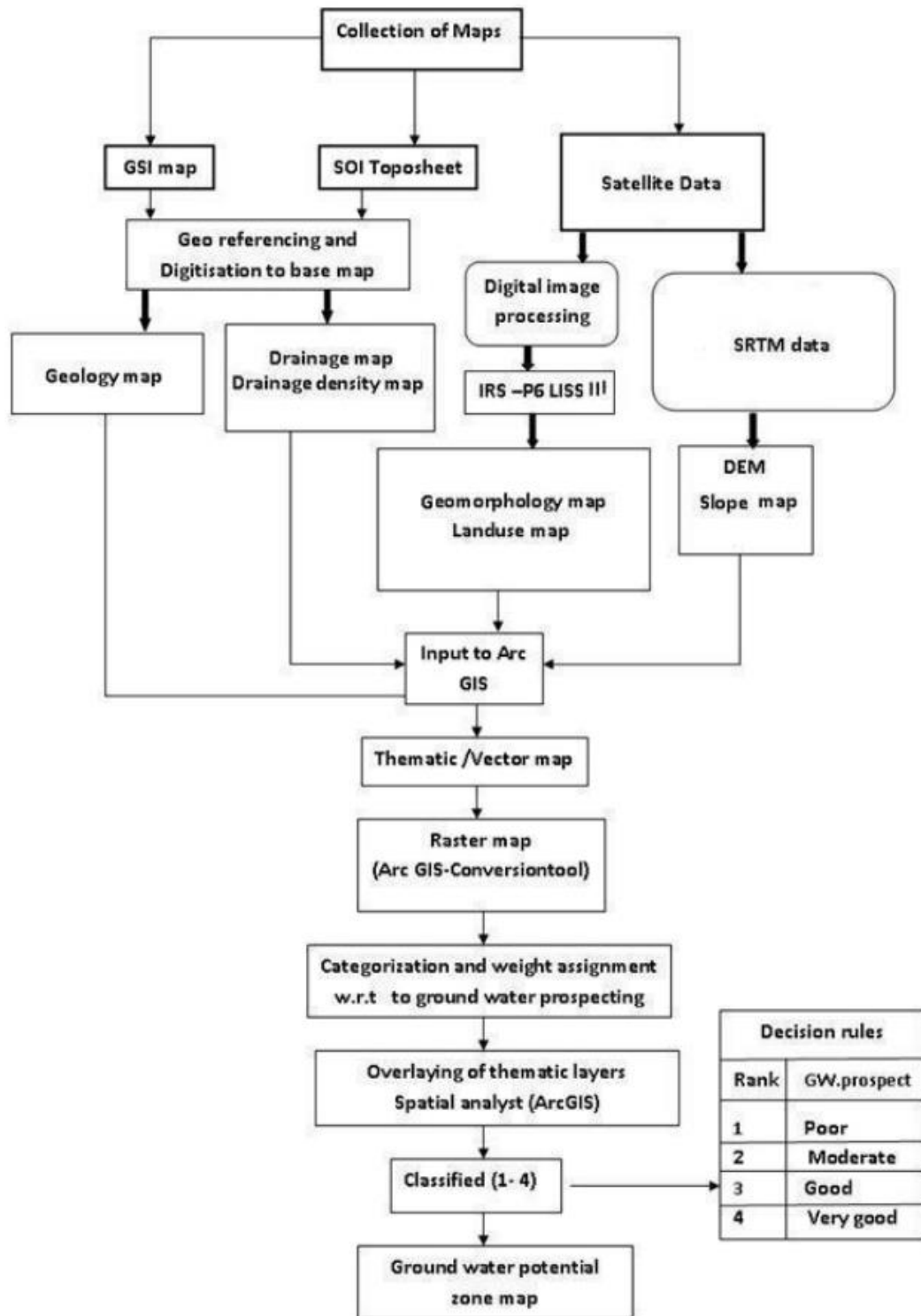
Fig. 3.12 Flow chart showing the methodology for groundwater prospect zone delineation.
