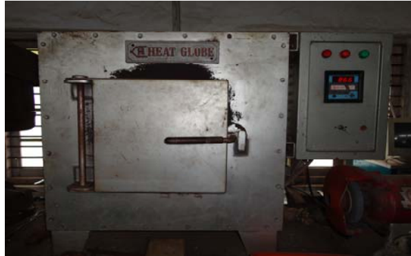
Figure 2.1: Furnace used for melt quenching
