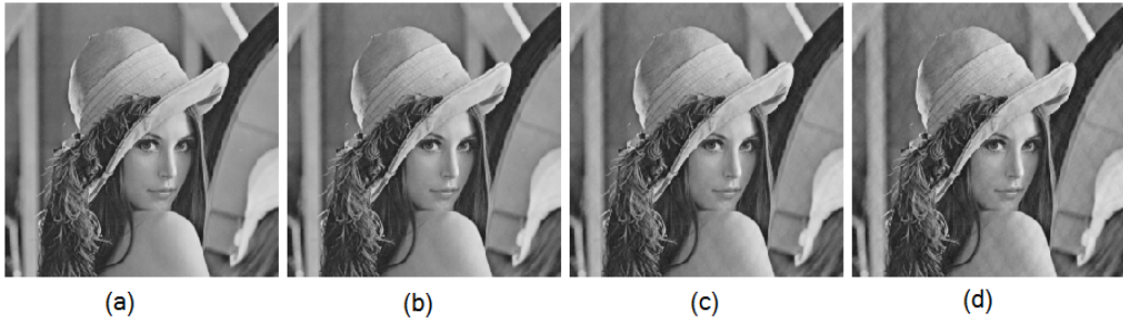
Fig. 5.7: (a)Original lena image (b) Reconstructed image by scaling uniformly c_1, c_2 \geq 16 by a factor (b) 1.5 (c) 2 (d) 2.5
