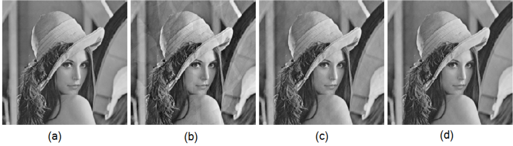
Fig. 5.6: (a)Original lena image, reconstructed image by scaling uniformly (b) c_1, c_2 \geq 4 (c) c_1, c_2 \geq 8 (d) c_1, c_2 \geq 16 by a factor 1.5
