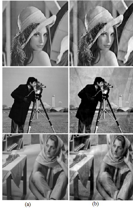
Fig. 5.5: (a)Original images (b)Reconstructed images by scaling uniformly all diagonal blocks having same row column sequency by a factor 1.5
