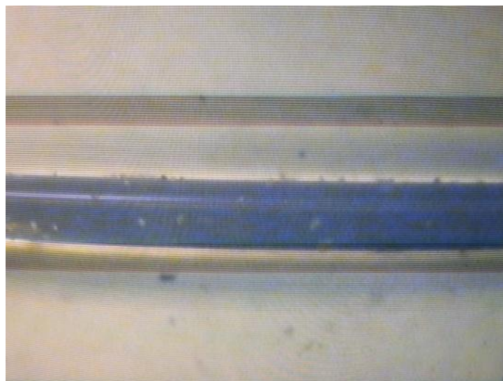
Figure 4.15: Photograph of Au nanoparticles doped hollow fiber under a CCD camera. Violet colour is the characteristics of Au nanoparticles in MMA environment.
