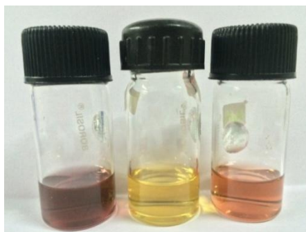
Figure 6.7: Image showing the colour of (left) Au nanoparticles (middle) Ag nanoparticles and (right) alloy of Au-Ag in PVP solvent.
