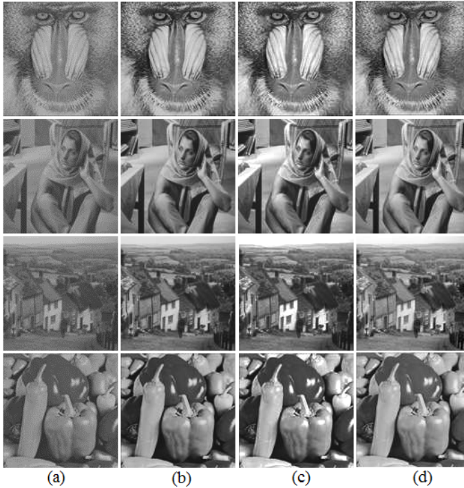
Fig. 6.8: (a) Original images, Enhanced images using (b) FIOP, (c) FIOS, (d) FRBS methods
