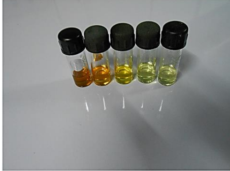
FIG. 2. Photograph of C1, C2, C3, C4, and C5 nanocolloids showing quantum size effect.
