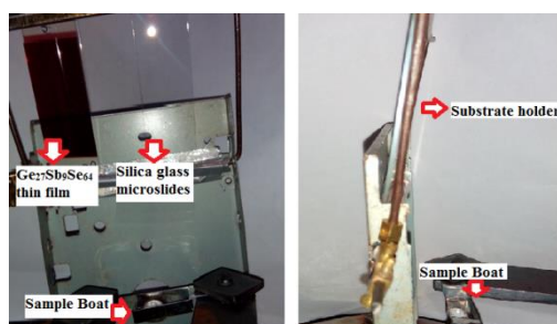
Figure 6.4: The front view and side view of OAD substrate holder containing chalcogenide glass thin film as well as silica glass substrate.
