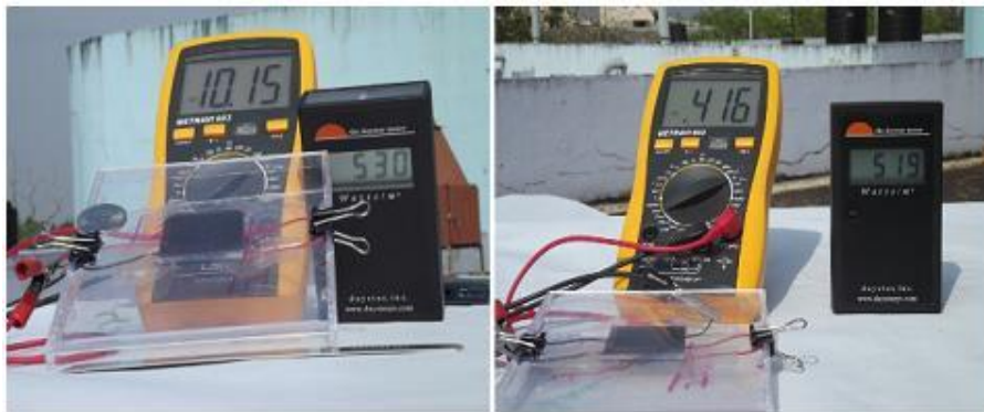
Figure. 3.5 Outdoor measurements of ITO/CuInS 2 /In 2 S 3 /Ag solar cells with an active area of 5cm 2 to study the performance of the device under direct sunlight.
