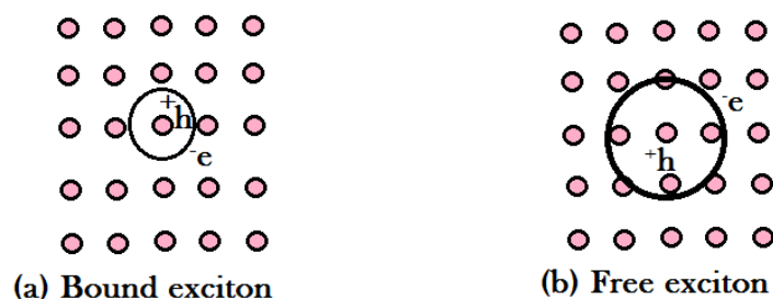
Figure 3.9: (a) Bound excitons: electron is strongly bounded and confined to within a single lattice constant. (b) Free excitons: electron is weakly bounded with an average radius larger than the lattice constant.
