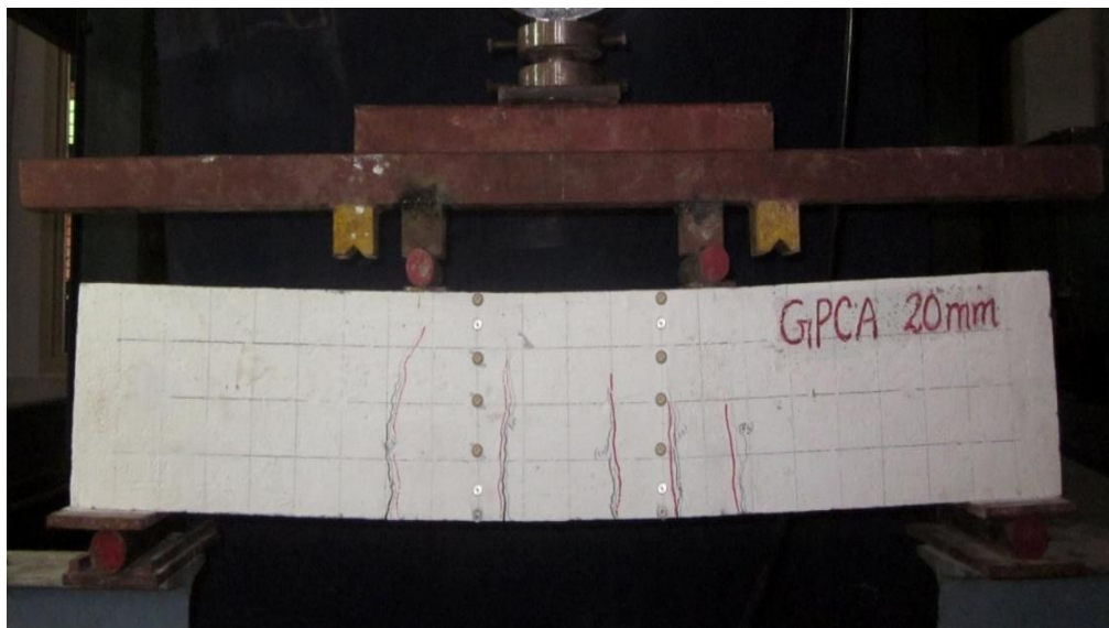
Fig. 6.7. Typical crack pattern of GP concrete beam
