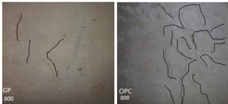
Fig. 5.10. Cracking behaviour of GP and OPC concrete after a temperature exposure of 800 °C
