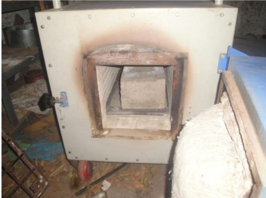
Fig. 3.5. Photograph of electric furnace
