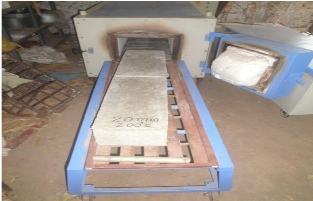
Fig. 3.6. Photograph of heated specimen on bench for air cooling
