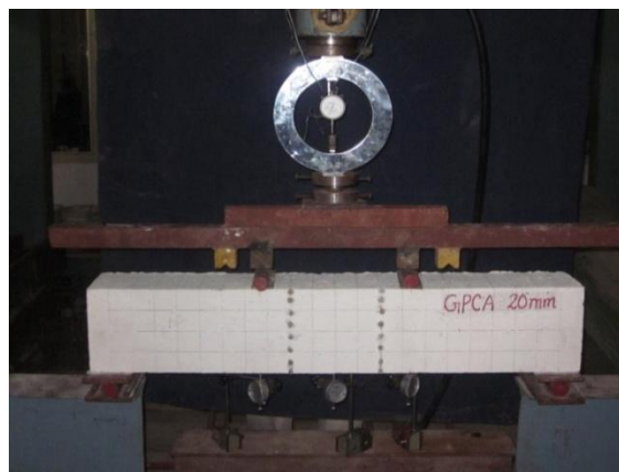
Fig. 6.2. Experimental set up for loading GP concrete beam
