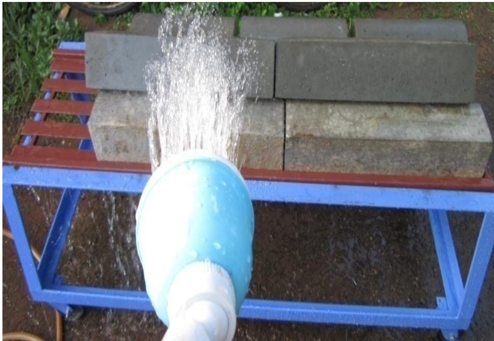
Fig. 3.7. Photograph of water spray cooling of specimen
