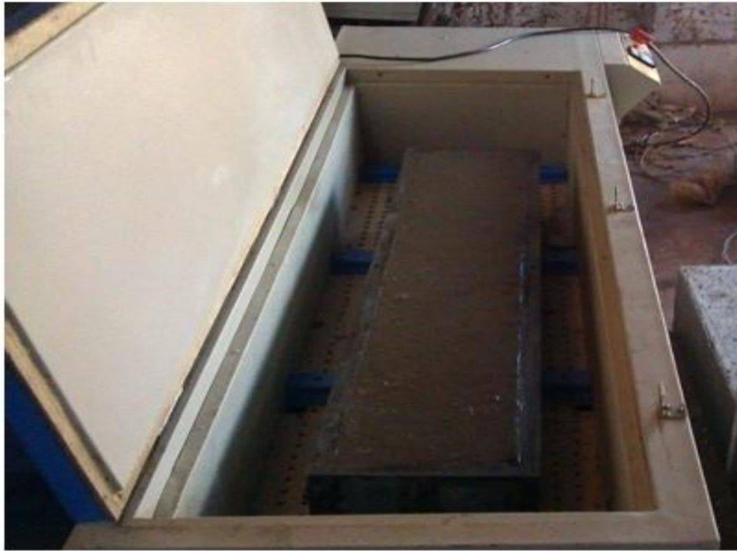
Fig. 3.4. Photograph of electric oven for temperature curing of geopolymer concrete beam
