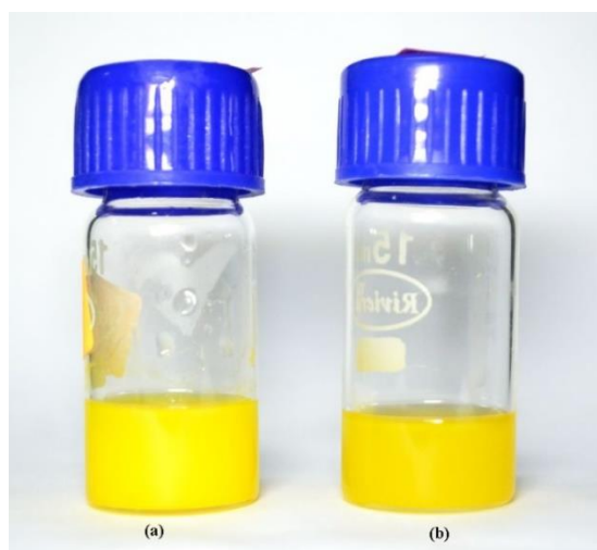
Figure 5.16: Photographs of (a) CdS:TiO 2 PVA and (b) CdS PVA nanocomposites
