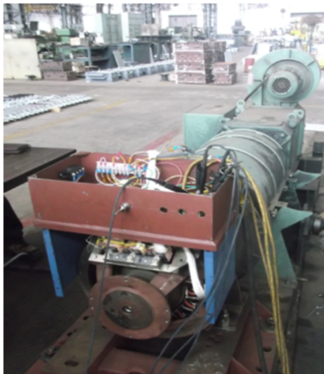
Fig. 5.14: The 45 KVA experimental machine with third harmonic excitation system
