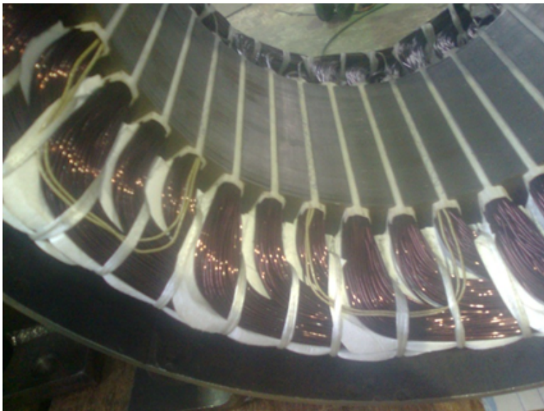
Fig. 5.12: Main and auxiliary windings in the stator
