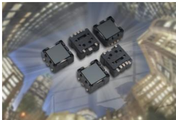
Fig. 1.11 IRS-B series detectors manufactured by Murata Manufacturing Co., Ltd. (Japan)
