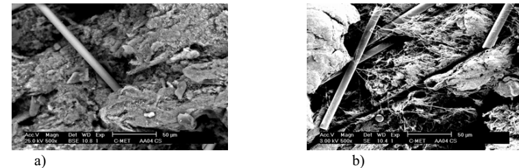
Figure. 1 SEM micrograph of cross section of a) PTFE/fused quartz (silane coated) composite b) PTFE/Fused quartz (uncoated) composite
