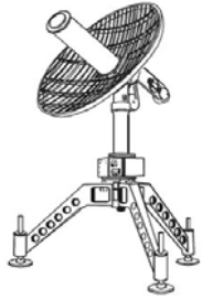
Fig.1 Parabolic reflector tracking antenna in Radio Theodolite system
