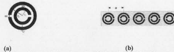
Figure 1(a). Schematic drawing of an SRR unit cell. (b) SRR array with period a
