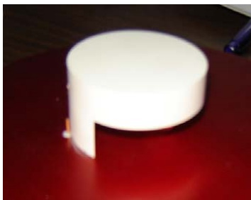
Fig.2. Shaped DRA: DCS-WLAN bands
