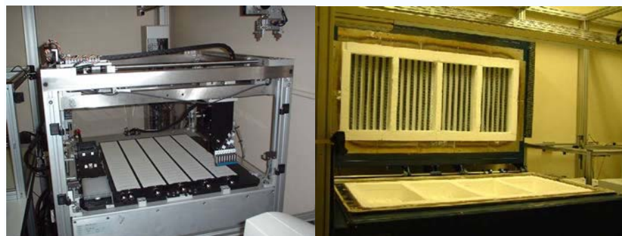
Left: Fig. 1, the printing bed of LUSI. This can hold 100 alumina substrates, each of which can contain 30 or 40 printed dots (1-2 mm diameter), each of a different composition. The inkjet printer can be seen on the right, and a robot arm moves the samples from printer to furnace to measurement table, all under automation.
