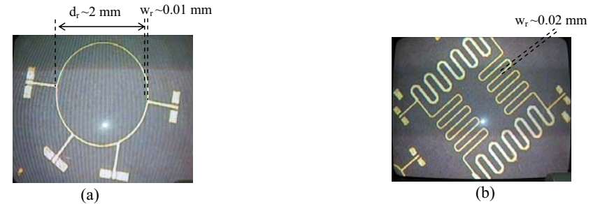
Figure 3 Micro photographs showing the circuits and dimensions of very fine geometries printed using photoimageable thick film techniques
