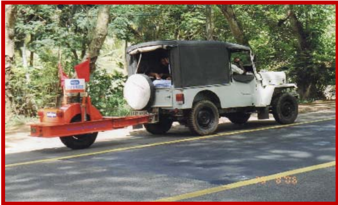
Fig. 3.9 Roughness Survey in Progress
