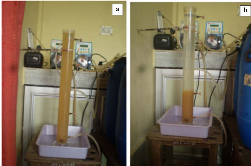
Fig 4.53 Experimental set-up for the treatment of latex processing wastewater (a) during aeration (b) during settling
