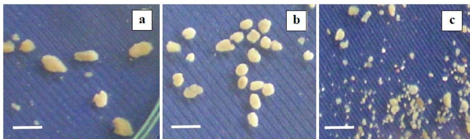
Fig.4.25. Granular sludge formed under various shear forces, on 35 th day (a) trial 4 (b) trial 2 (c) trial 5 (bar = 5 mm)
