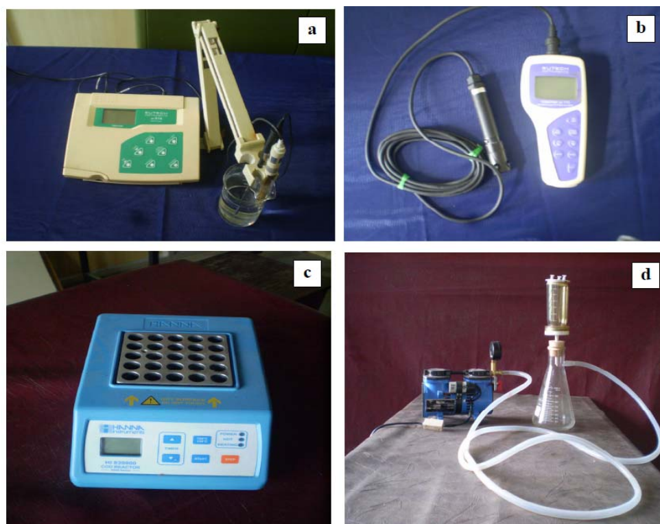
Fig. 3.8 Analytical instruments used for the study (a) pH meter (Cyberscan pH-510) (b) DO meter (Cyberscan DO-110) (c) COD digester (Hanna make, Model HI 83099) (d) vacuum pressure pump assembly for SS determination
