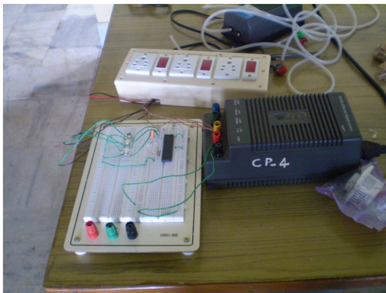
Fig 3.6 Micro-controller AT89C51 assembly for the experimental set-up
