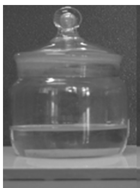
Figure 7.2 Immersion test in diffusion bottles
