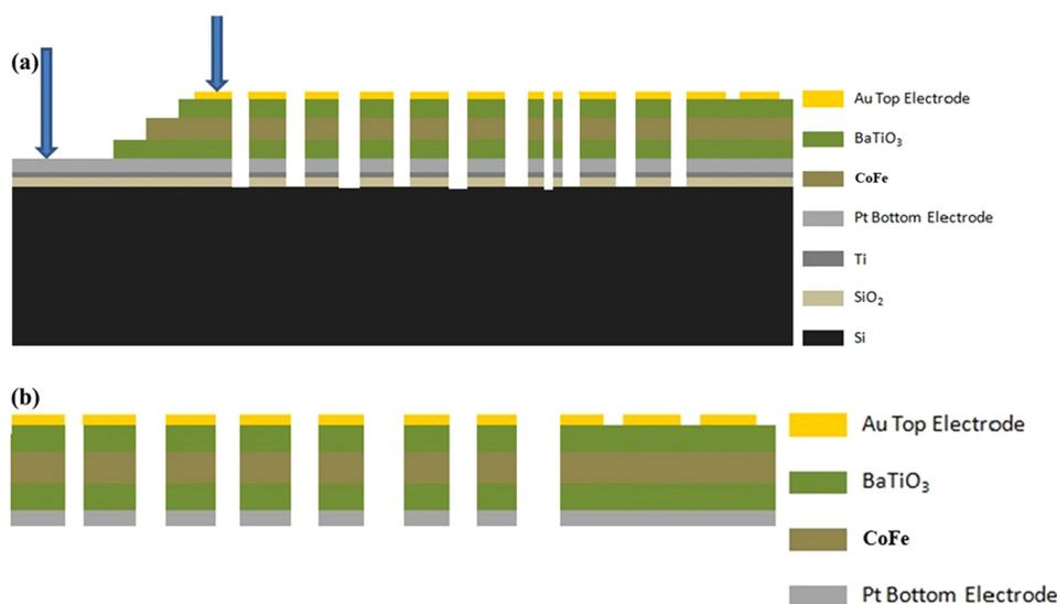
SCHEME 2. Fabrication of magneto-electric cantilevers and microwire sensors through micromachining. (a) Dissolving the thin film and substrates to obtain desired size and shapes (assisted by pre designed masks). (b) Complete dissolution of the substrate to release the micro/nano magneto electric arrays (heterogeneous).
