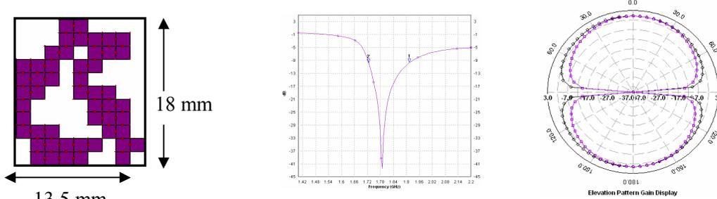
Figure.7 The final Genetic patch with optimized GP, R.L curve and Radiation Pattern
