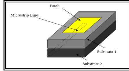
Figure.2. An electromagnetically coupled MSA
