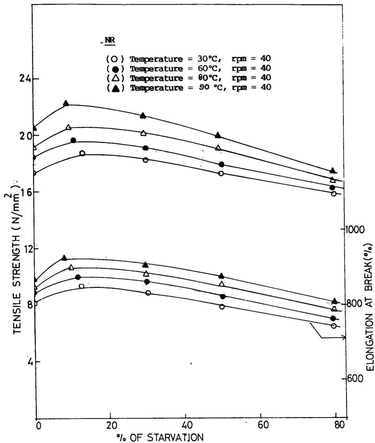
Fig.3.15: Variation of tensile strength and elongation at break of gum NR vulcanizates with percentage starvation at different temperatures.
