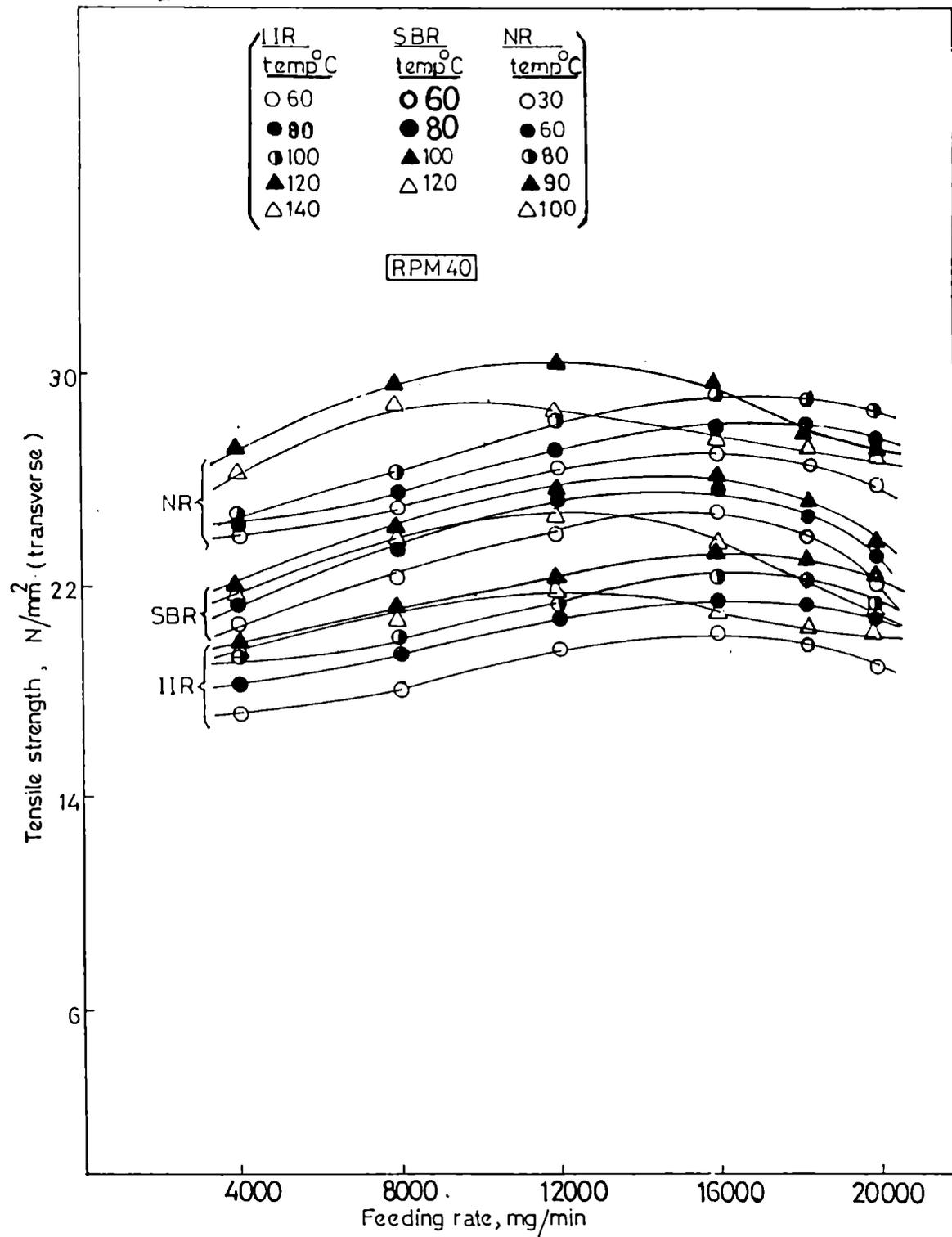
Fig.4.8: Variation of tensile strength of filled NR, SBR and IIR vulcanizates with feeding rate at different temperatures in the transverse direction.
