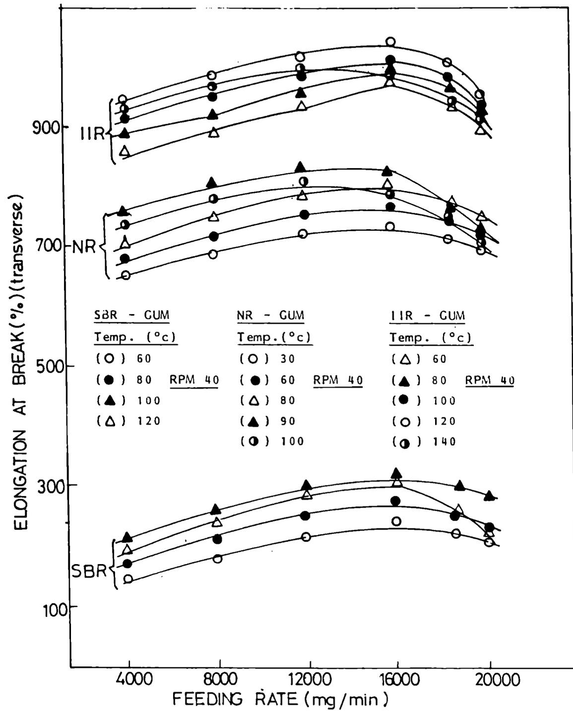
Fig.3.10: Variation of elongation at break of gum NR, SBR and IIR vulcanizates with feeding rate at different temperatures in the transverse direction.
