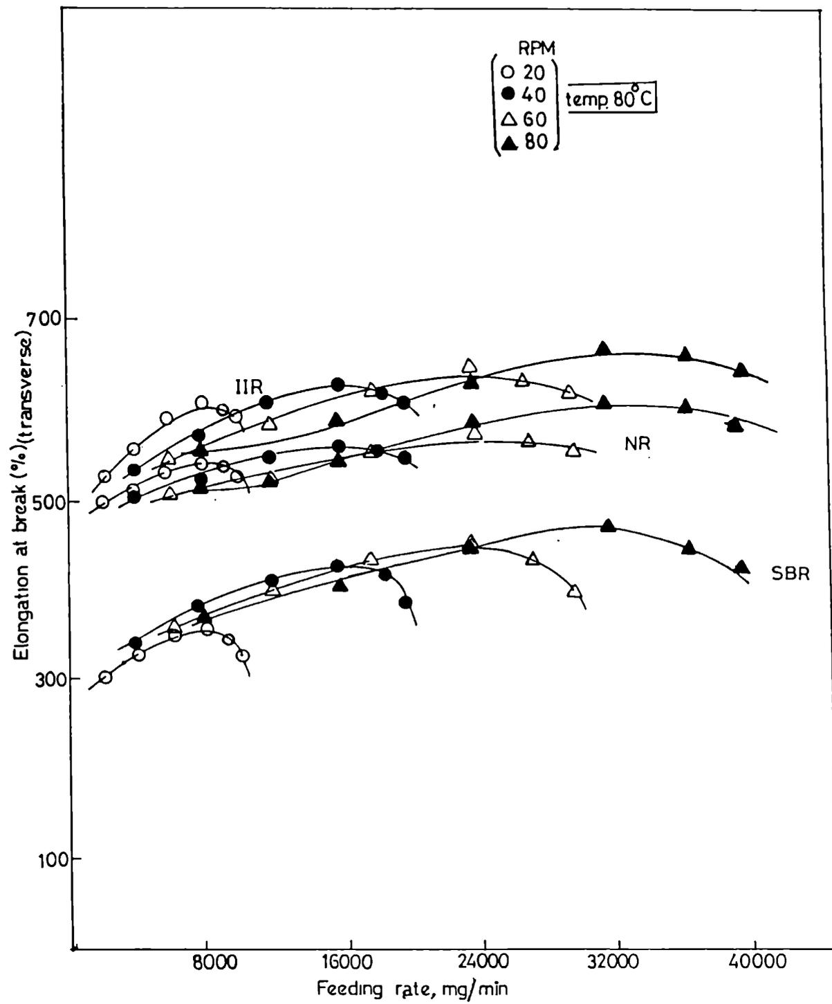
Fig.4.6: Variation of elongation at break of filled NR, SBR and IIR vulcanizates with feeding rate at different rpms in the transverse direction.
