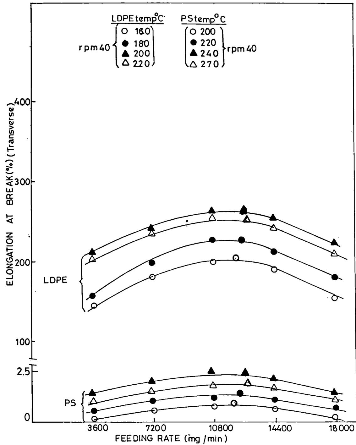
Fig.5.10: Variation of elongation at break of LDPE and PS with feeding rate at different temperatures in the transverse direction.
