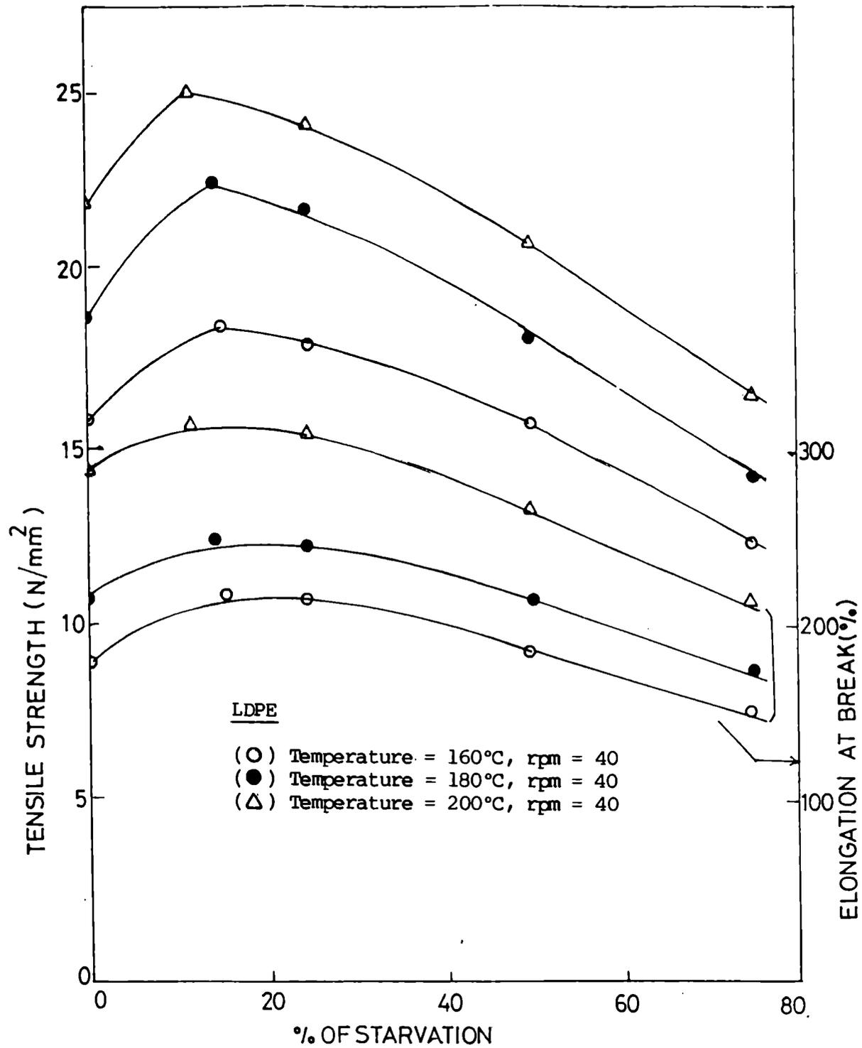
Fig.5.13: Variation of tensile strength and elongation at break of LDPE with percentage of starvation at different temperatures.
