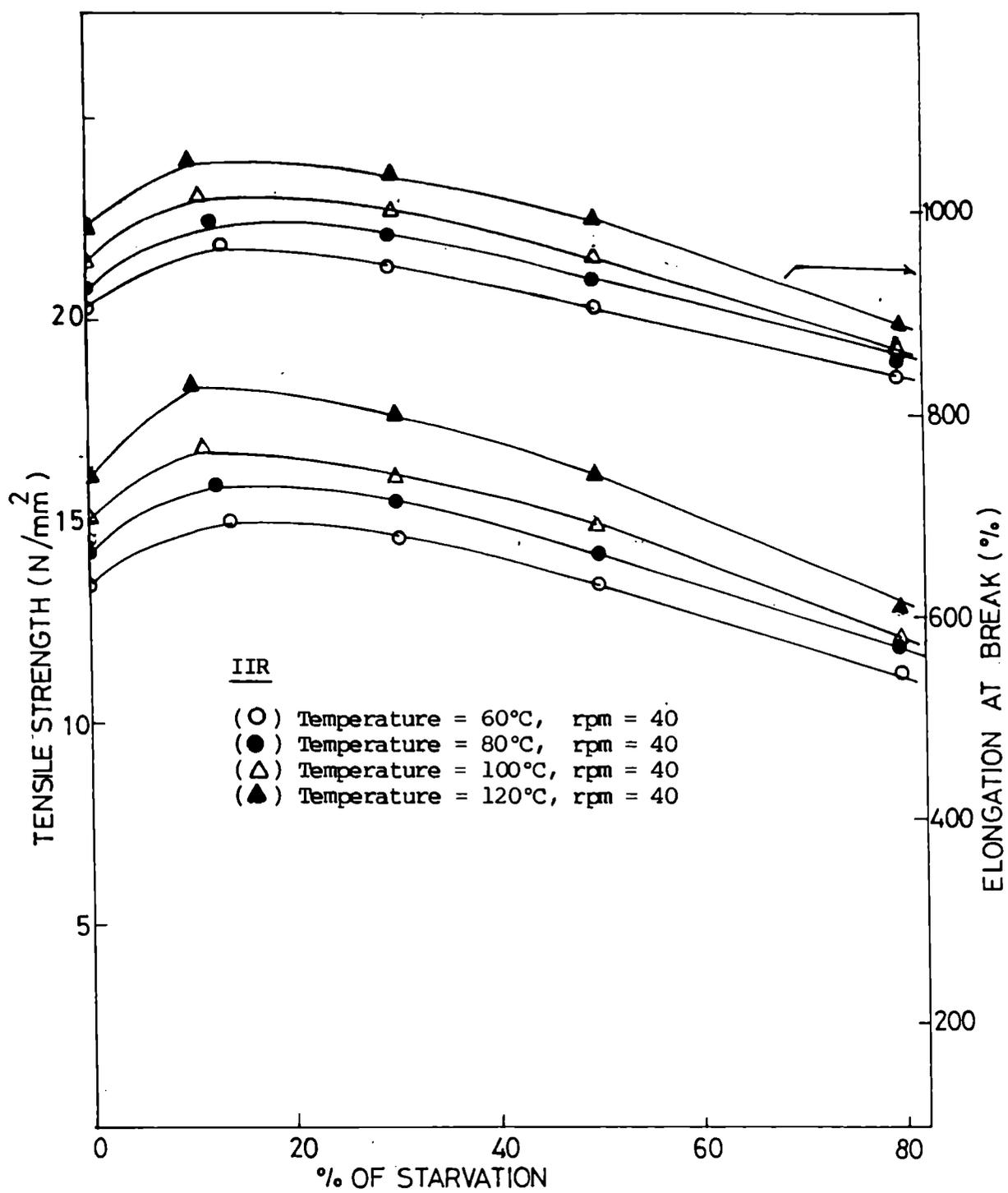
Fig.3.19: Variation of tensile strength and elongation at break of gum IIR vulcanizates with percentage starvation at different temperatures.
