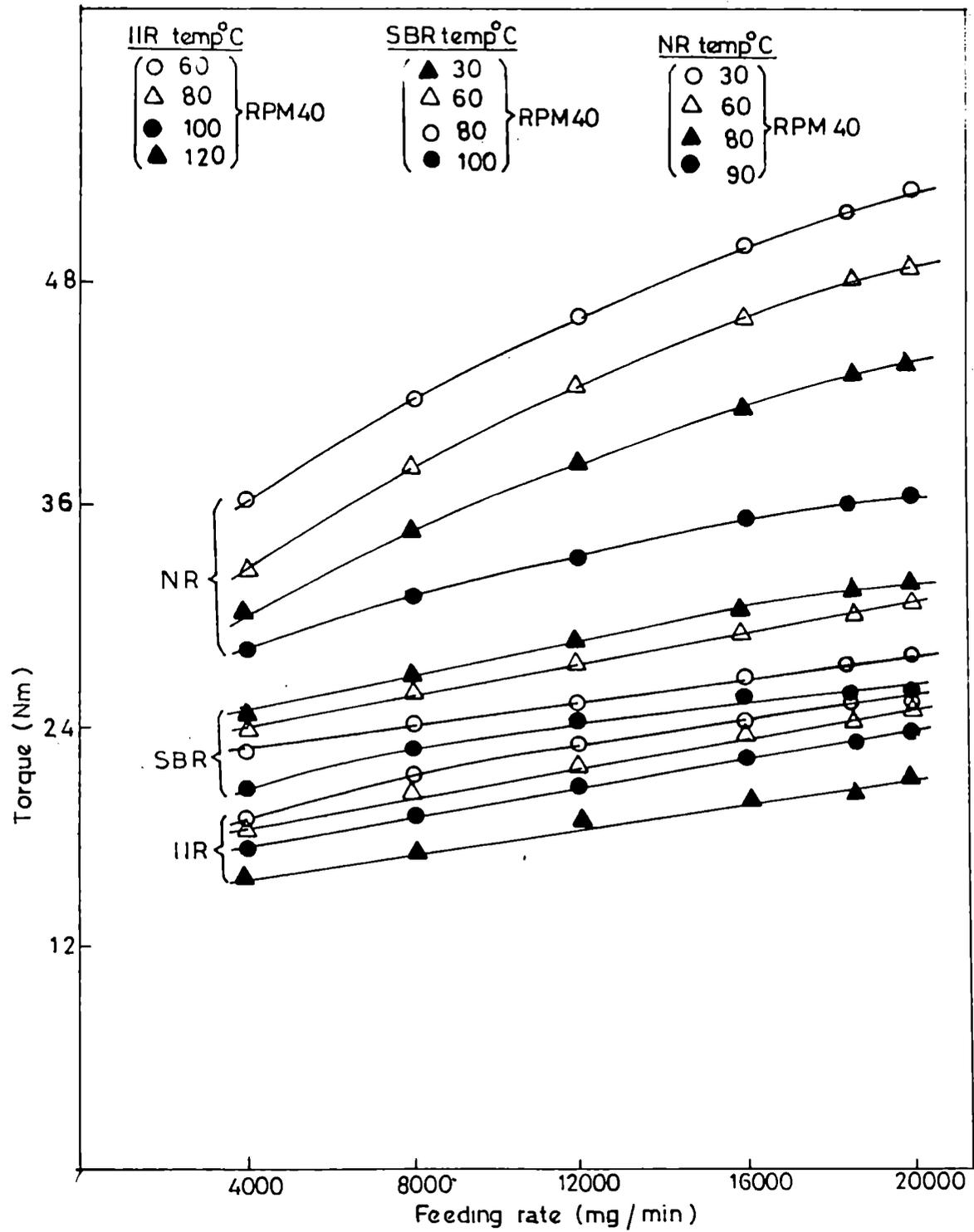
Fig.4.2: Variation of torque in the extrusion of filled NR, SBR and IIR compounds with feeding rate at different temperatures.
