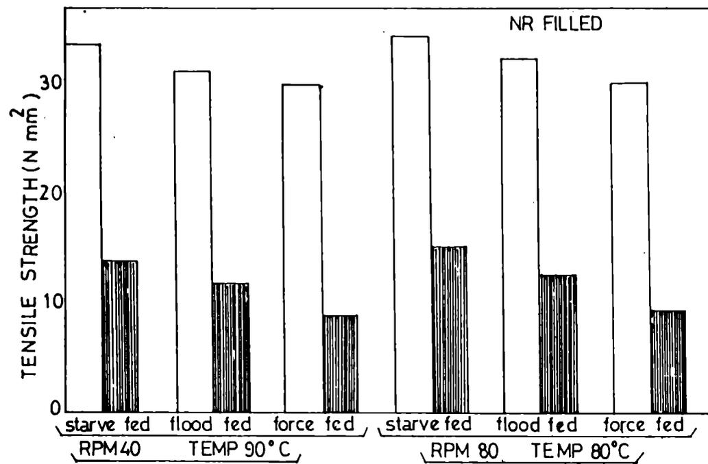
Fig.4.22: Variation of tensile strength and elongation at break of filled NR vulcanizates with different levels of feeding at different rpms and temperatures.
