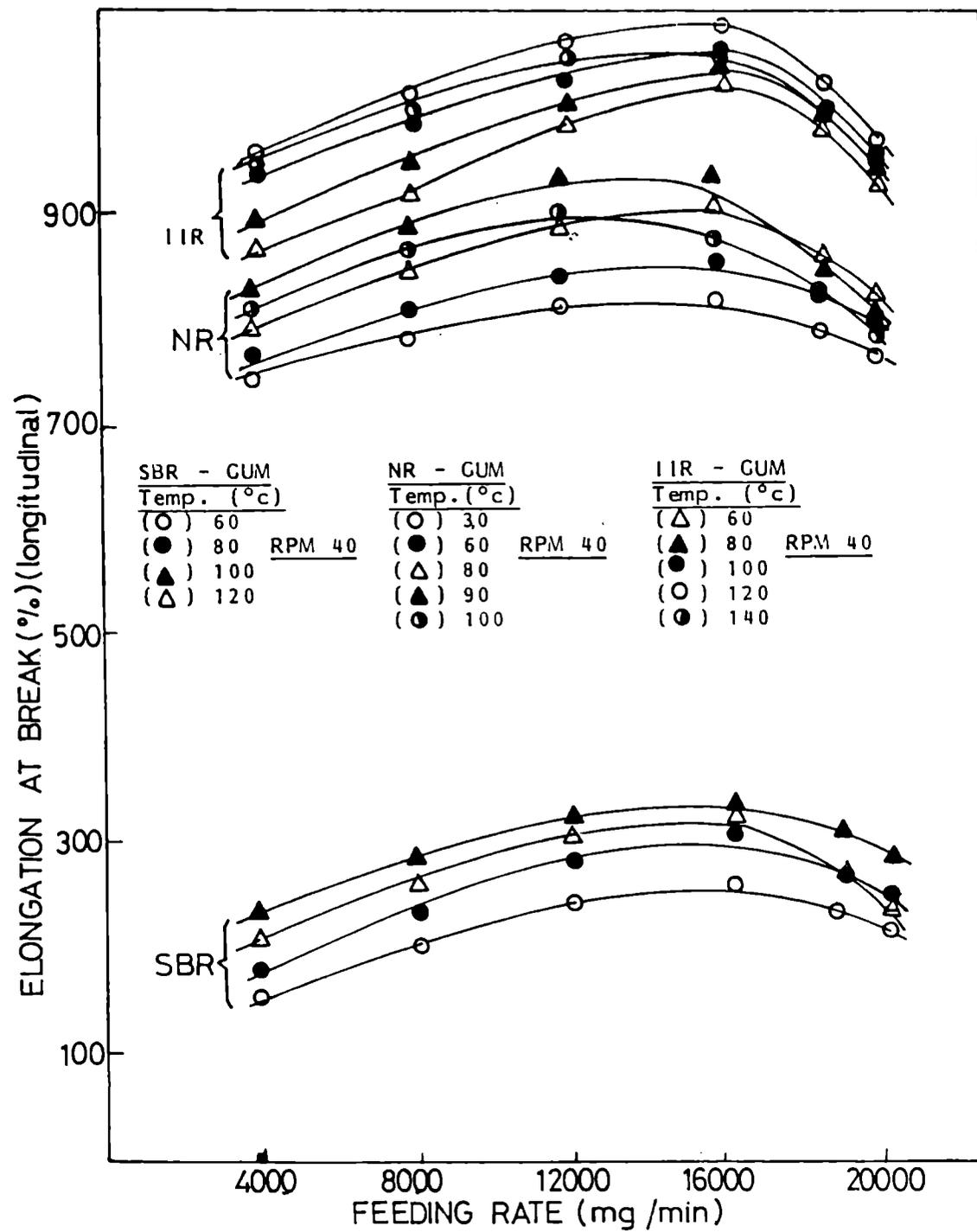
Fig.3.9: Variation of elongation at break of gum NR, SBR and IIR vulcanizates with feeding rate at different temperatures in the milling/extrusion direction.
