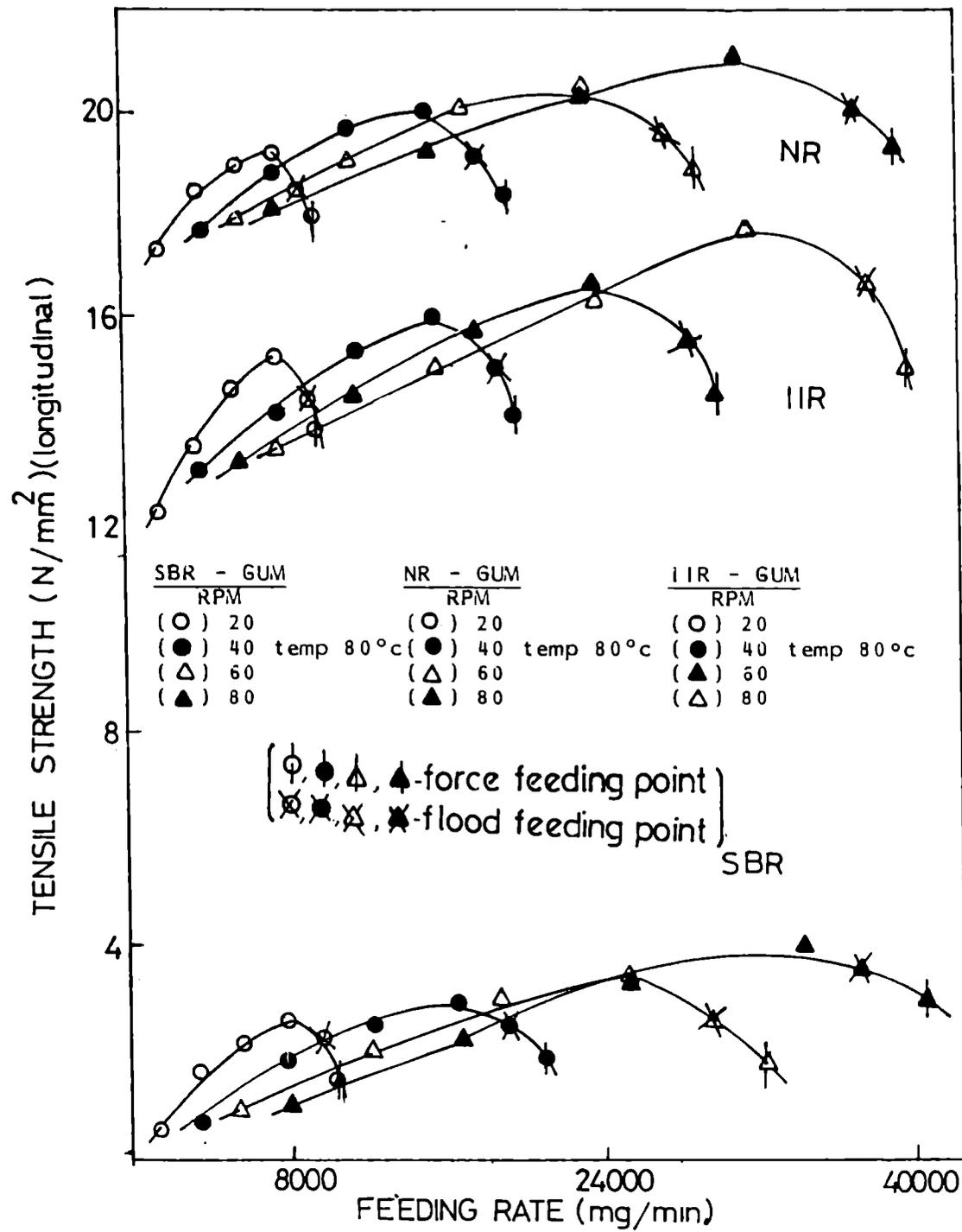
Fig.3.3: Variation of tensile strength of gum NR, SBR and IIR vulcanizates with feeding rate at different rpm in the milling/extrusion direction
