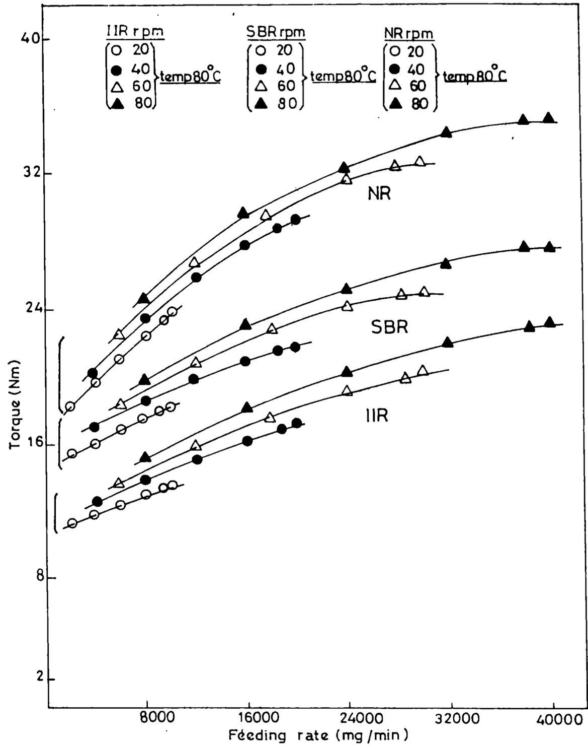
Fig.3.1: Variation of torque in the extrusion of gum NR, SBR and IIR compounds with feeding rate at different rpm.
