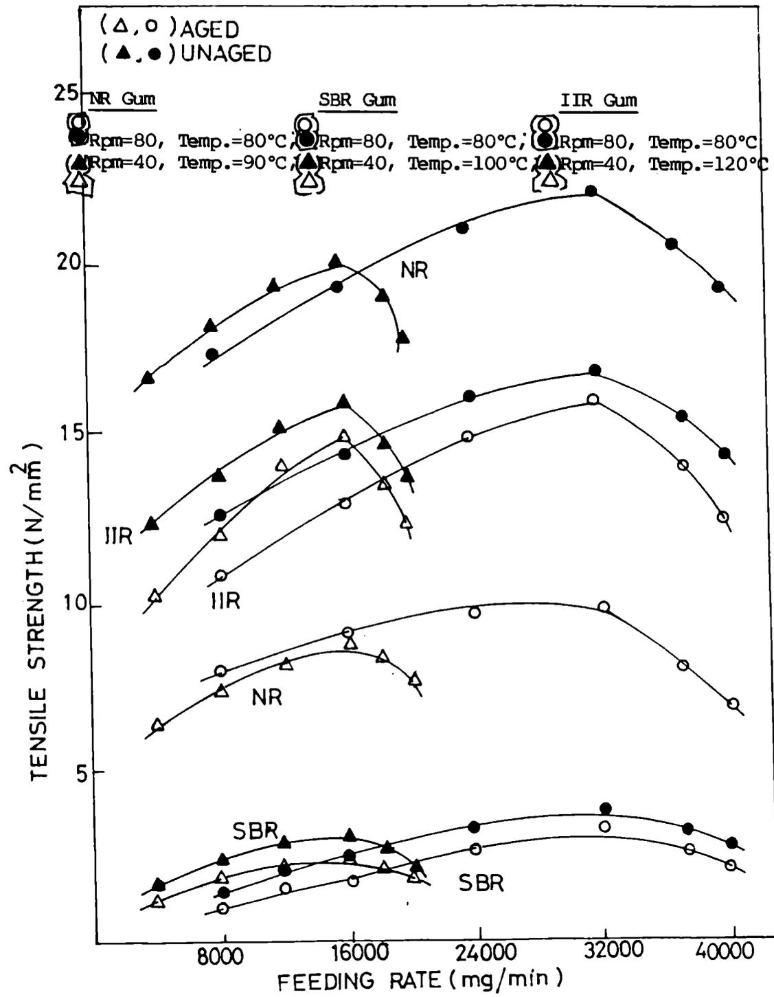
Fig.3.20: Variation of tensile strength of gum NR, SBR and IIR vulcanizates with feeding rate at different rpms and temperatures.
