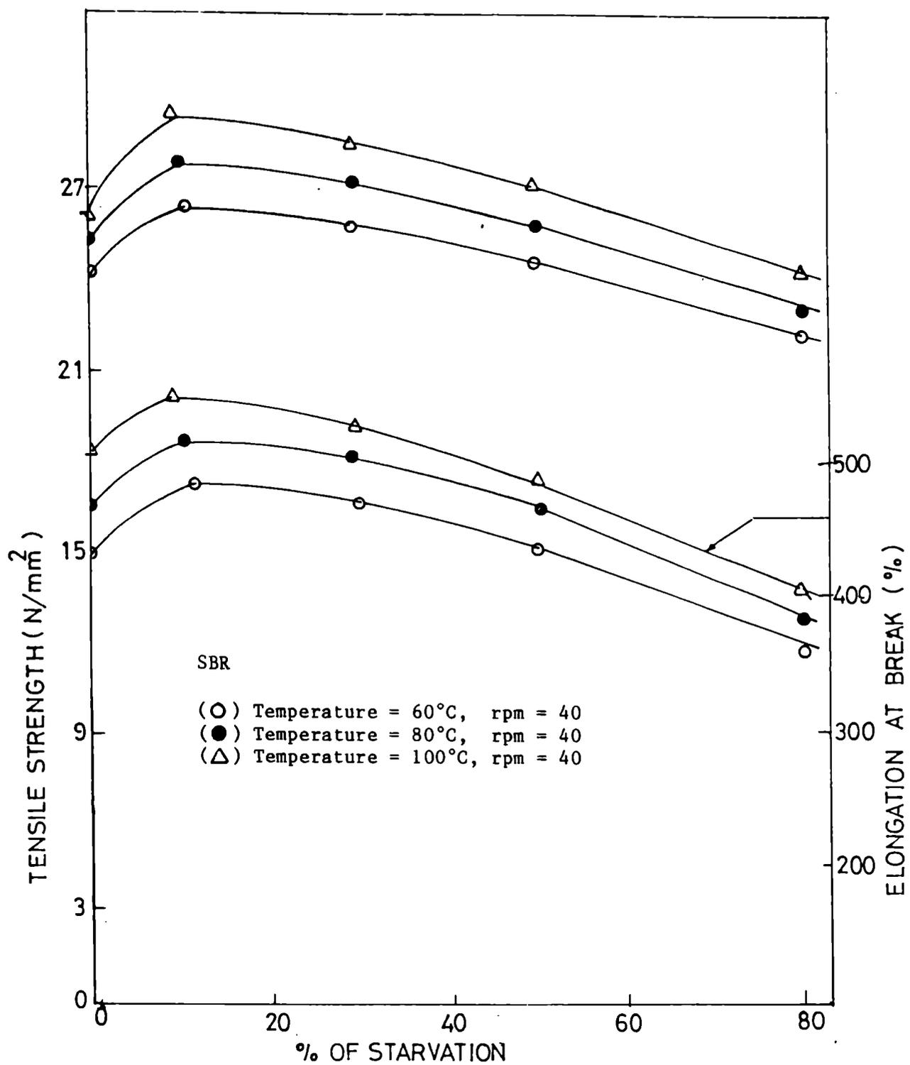
Fig.4.17: Variation of tensile strength and elongation at break of filled SBR vulcanizates with percentage starvation at different temperatures.
