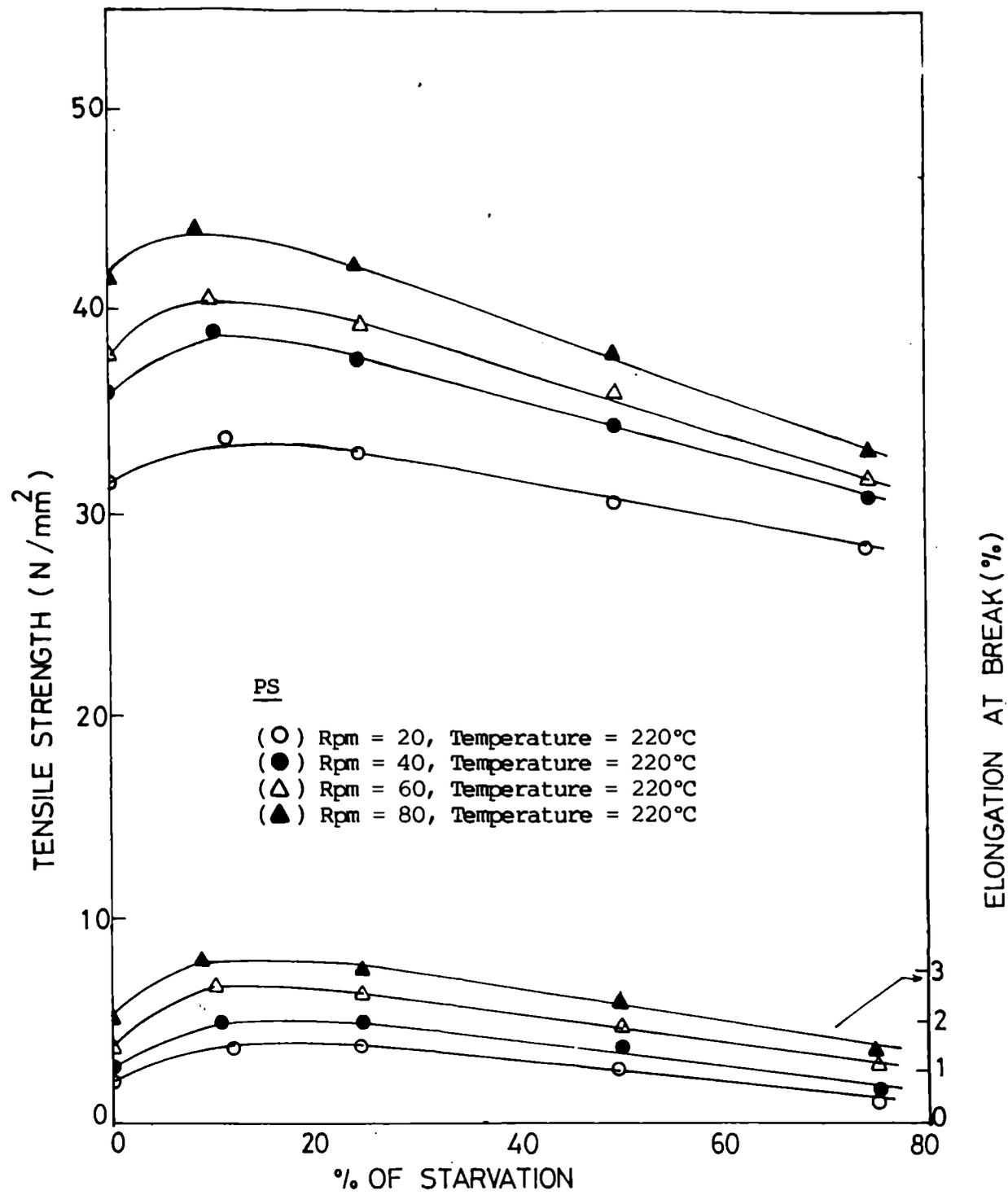
Fig.5.12: Variation of tensile strength and elongation at break of PS with percentage of starvation at different rpm.
