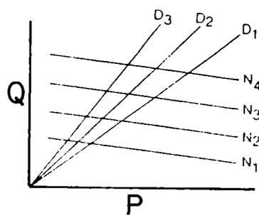
Fig.1.5: Family of screw characteristics with various die intersections
