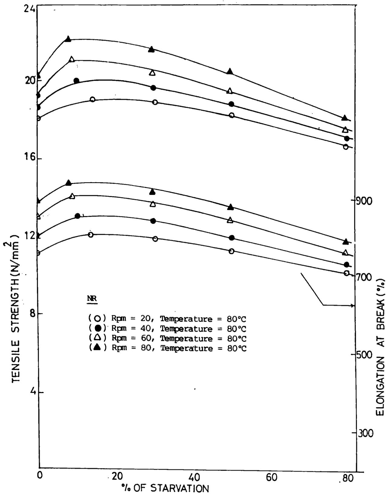
Fig.3.14: Variation of tensile strength and elongation at break of gum NR vulcanizates with percentage starvation at different rpms.
