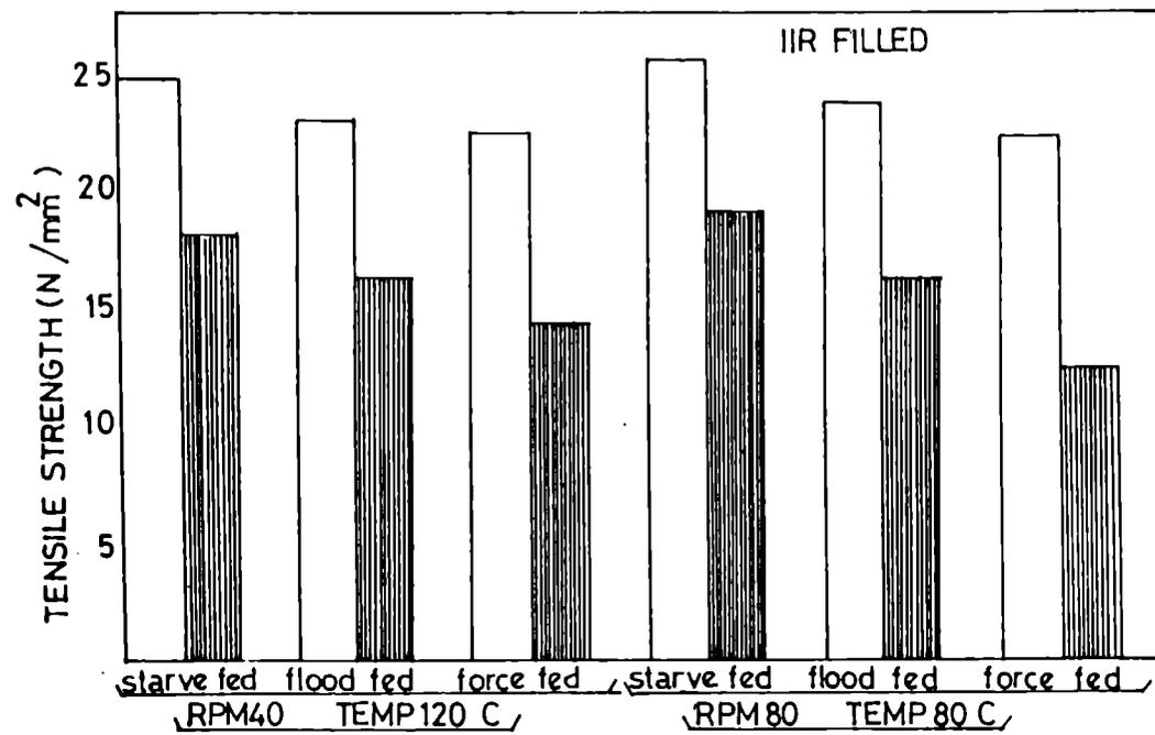
Fig.4.24: Variation of tensile strength and elongation at break of filled IIR vulcanizates with different levels of feeding at different rpms and temperatures.
