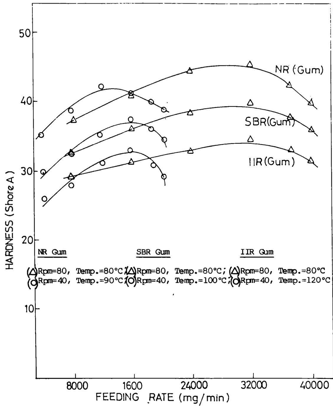
Fig.3.12: Variation of hardness of gum NR, SBR and IIR vulcanizates with feeding rate at different rpms and temperatures.
