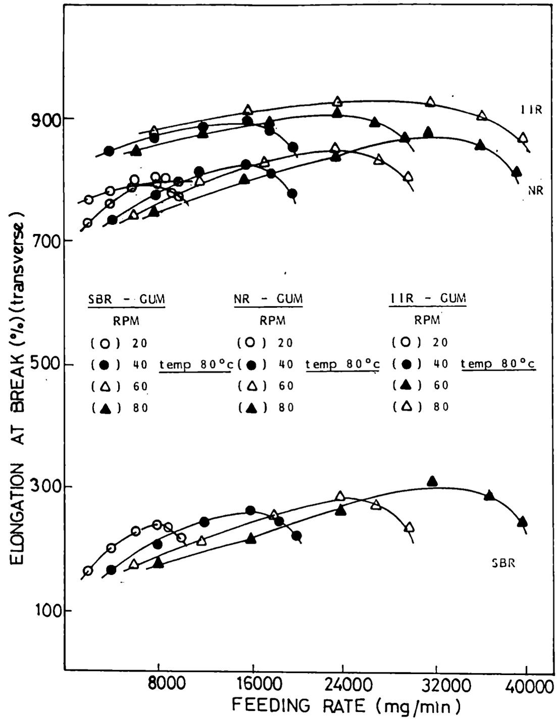
Fig.3.6: Variation of elongation at break of gum NR, SBR and IIR vulcanizates with feeding rate at different rpms in the transverse direction.
