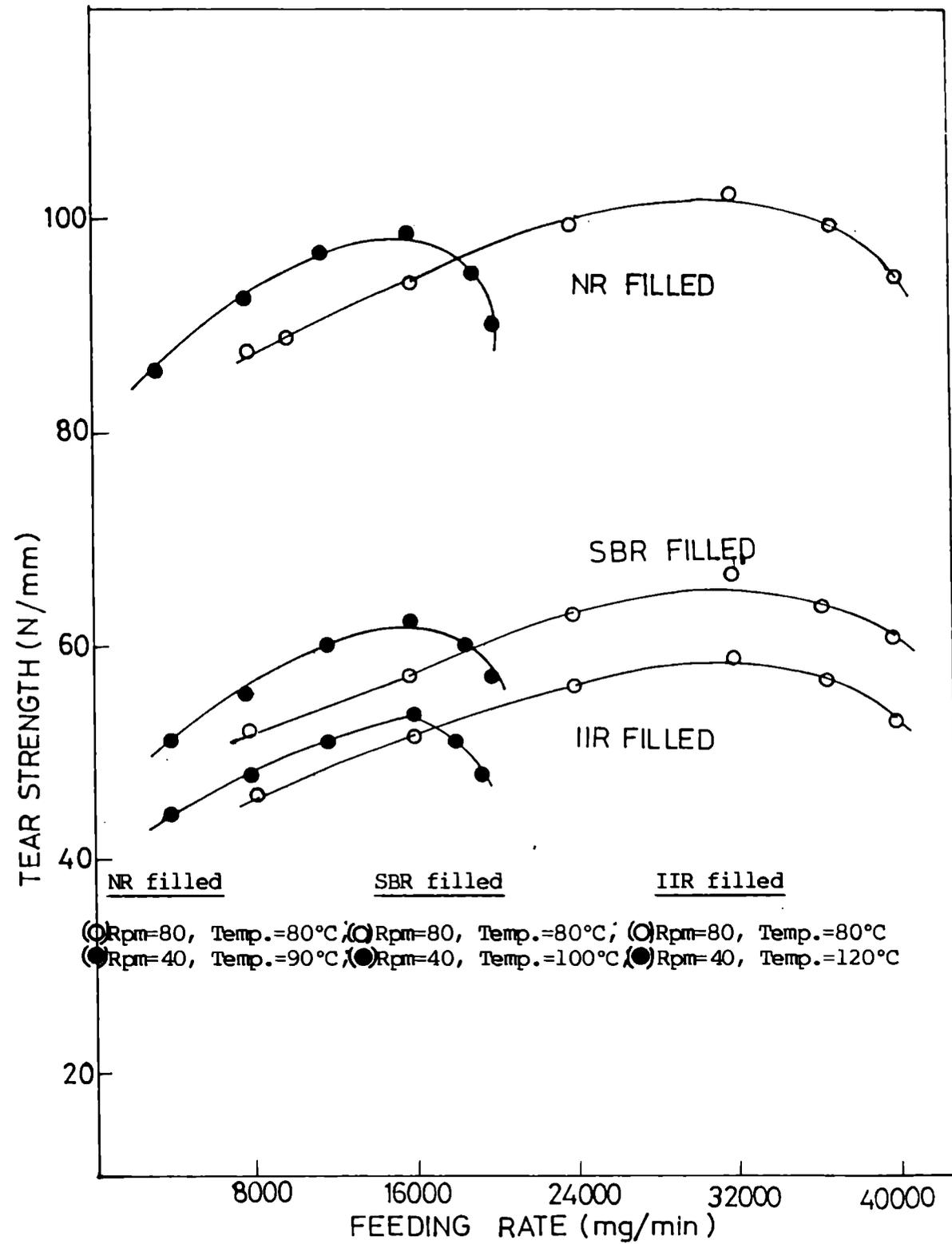
Fig.4.11: Variation of tear strength of filled NR, SBR and IIR vulcanizates with feeding rate at different rpms and temperatures.
