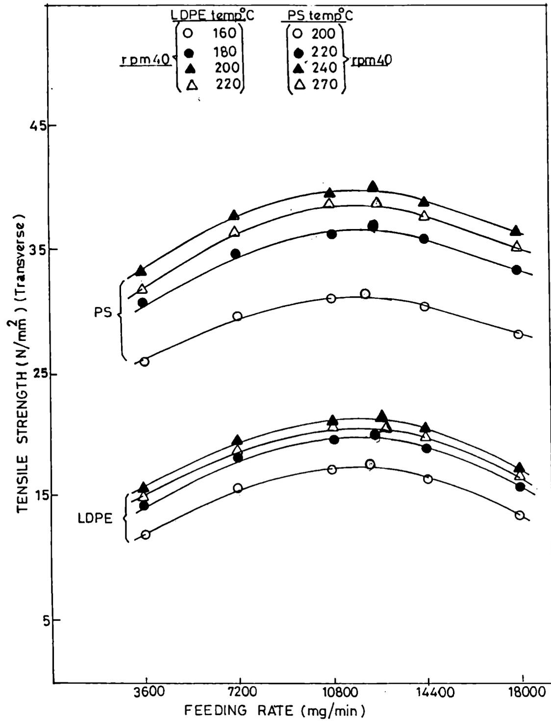
Fig.5.8: Variation of tensile strength of LDPE and PS with feeding rate at different temperatures in the transverse direction.
