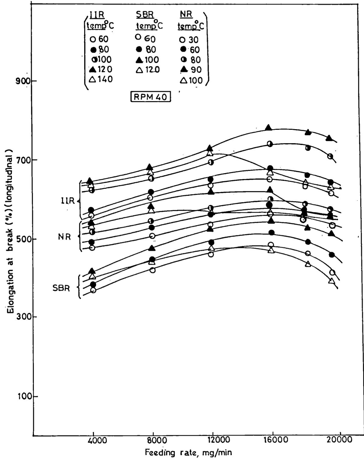
Fig.4.9: Variation of elongation at break of filled NR, SBR and IIR vulcanizates with feeding rate at different temperatures in the milling/extrusion direction.
