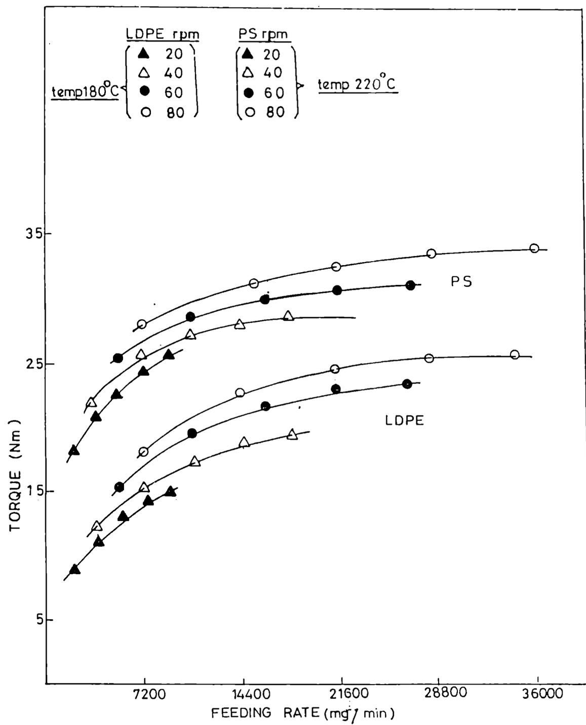
Fig.5.1 Variation of torque in the extrusion of LDPE and PS with feeding rate at different rpm.
