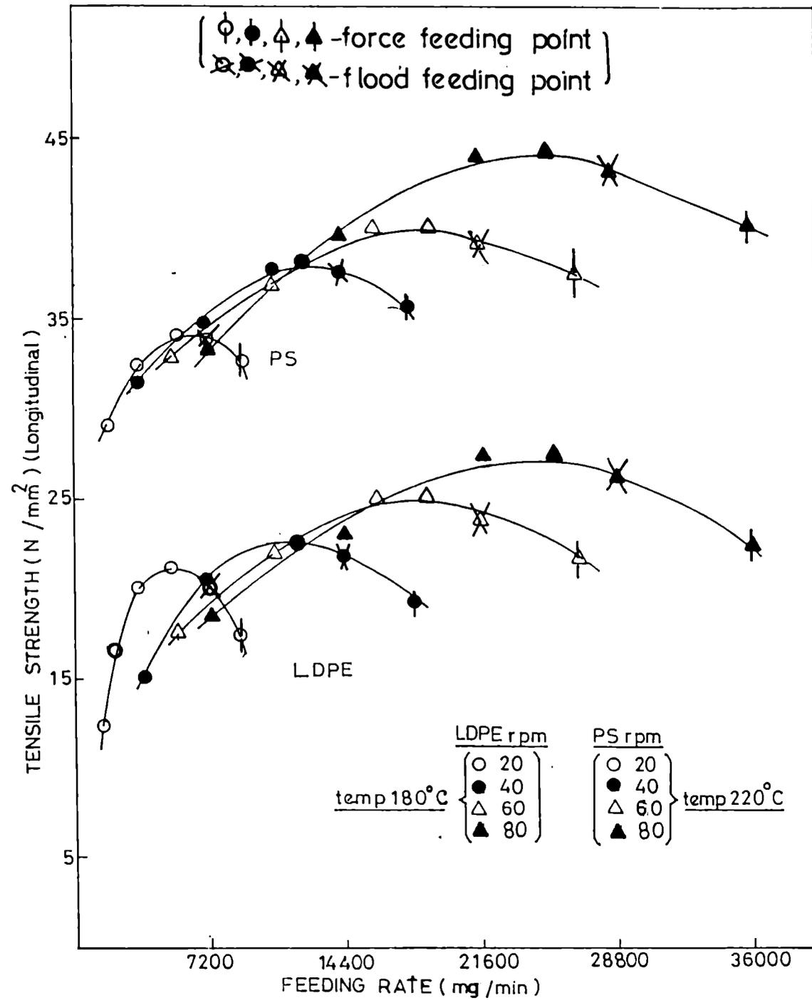
Fig.5.3: Variation of tensile strength of LDPE and PS with feeding rate at different rpm in the extrusion direction.
