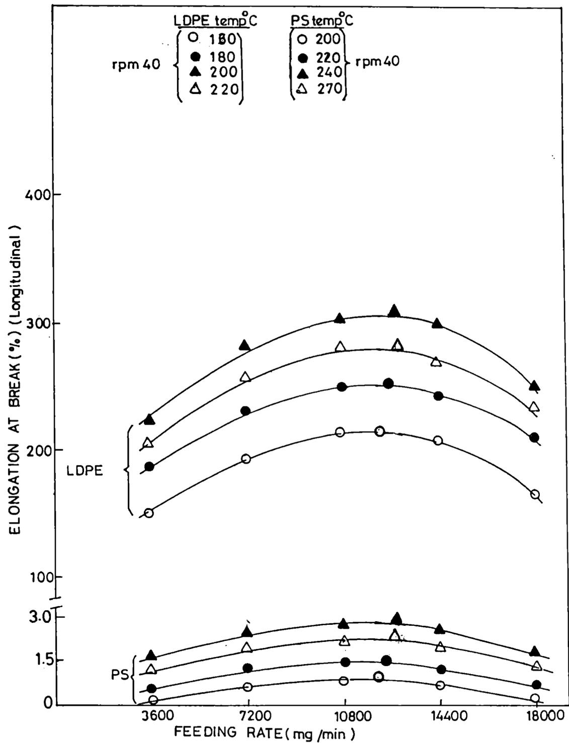
Fig.5.9: Variation of elongation at break of LDPE and PS with feeding rate at different temperatures in the extrusion direction.
