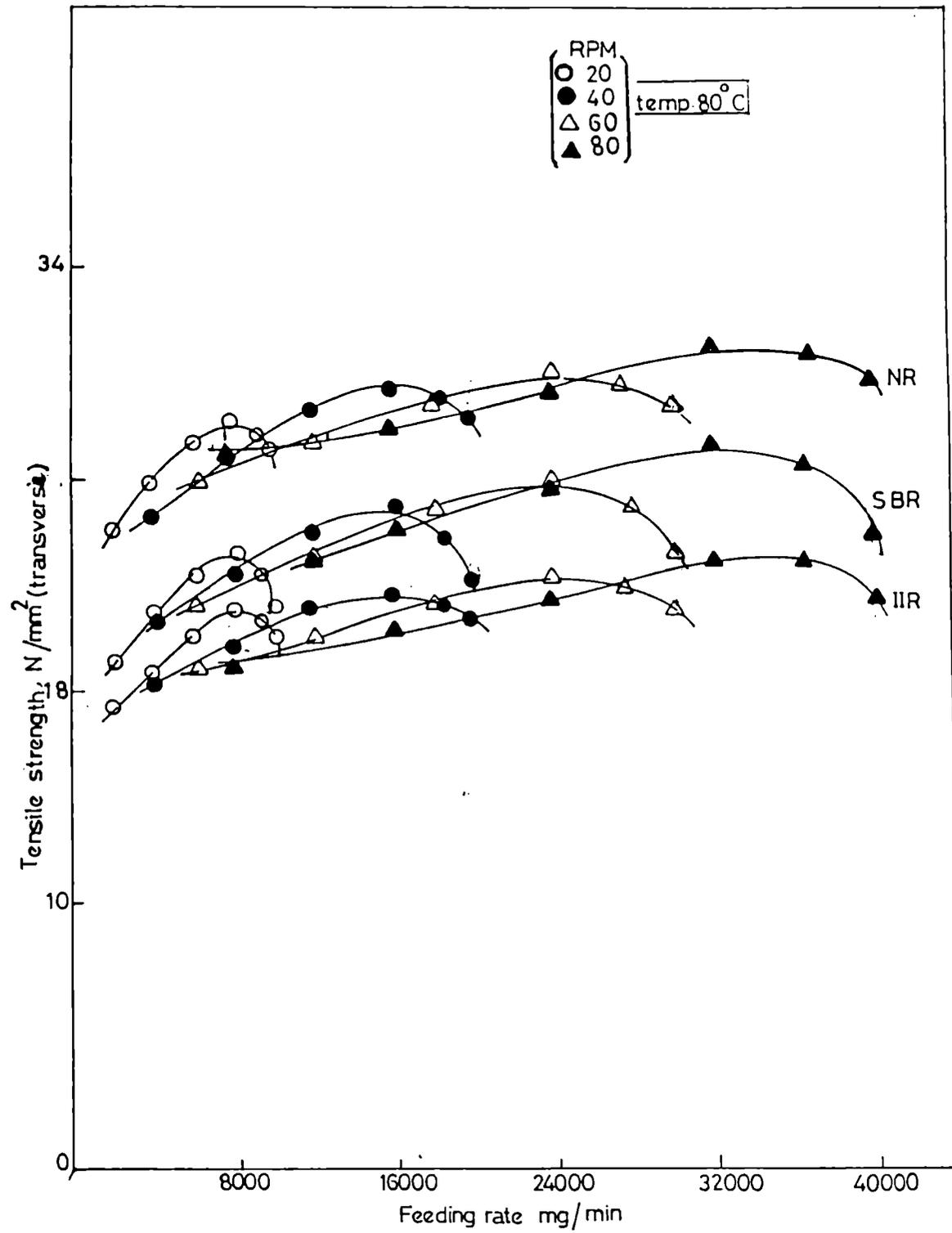
Fig.4.4: Variation of tensile strength of filled NR, SBR and IIR vulcanizates with feeding rate at different rpms in transverse direction.
