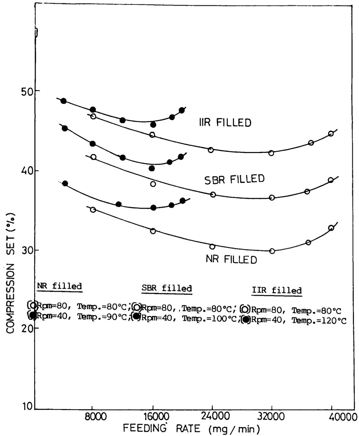
Fig.4.13: Variation of compression set of filled NR, SBR and IIR vulcanizates with feeding rate at different rpm and temperatures.
