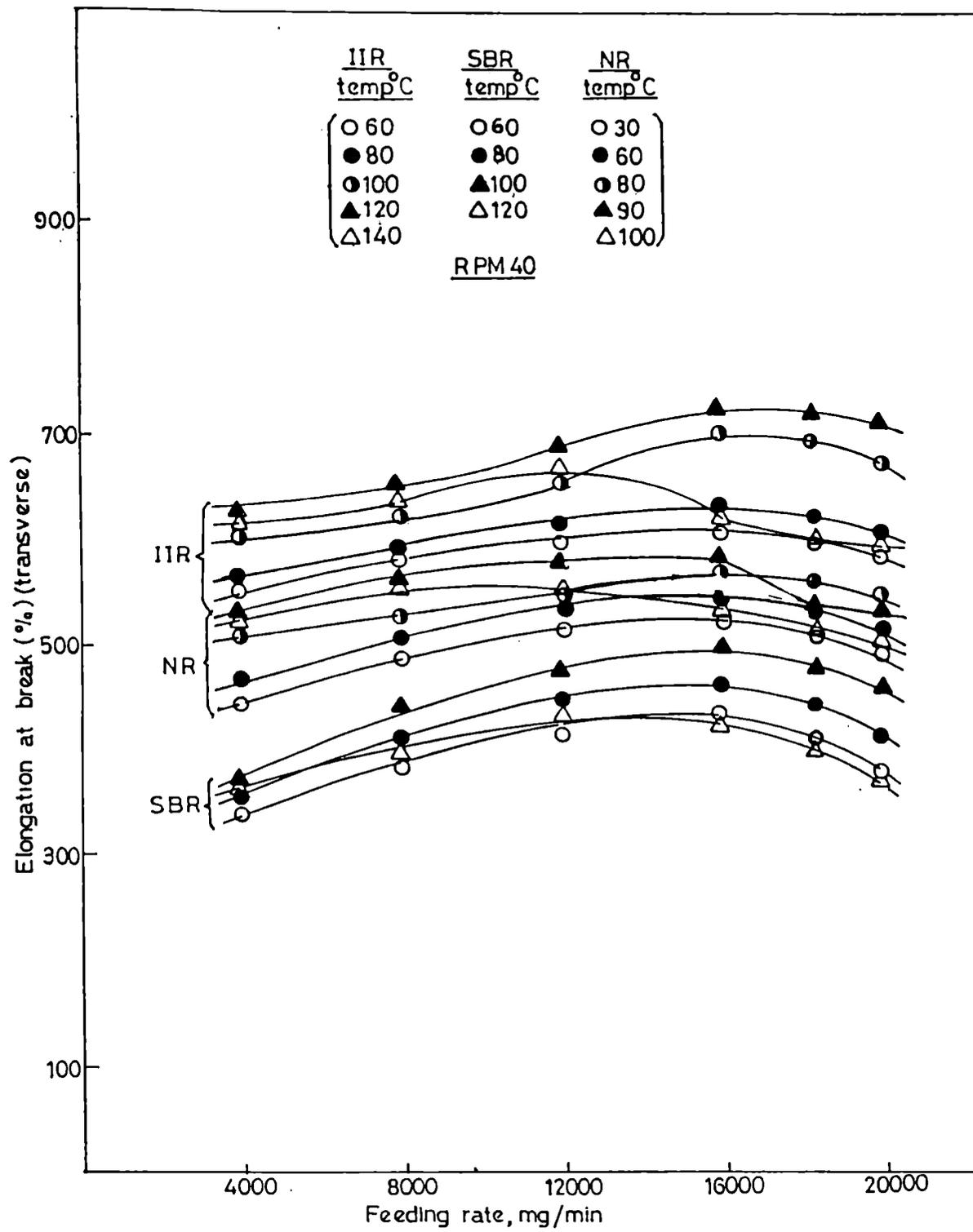
Fig.4.10: Variation of elongation at break of filled NR, SBR and IIR vulcanizates with feeding rate at different temperatures in the transverse direction.
