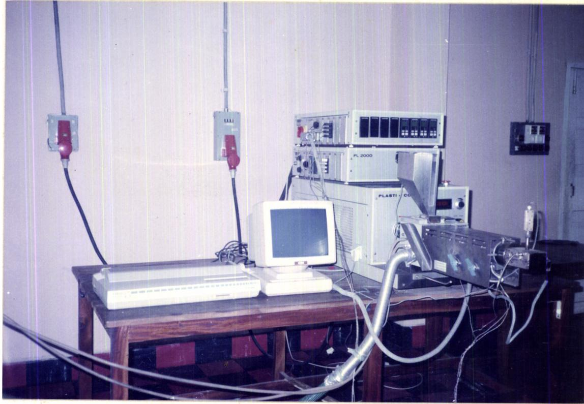
Fig.2.1: Brabender PL 2000 with plastic extruder and die.
