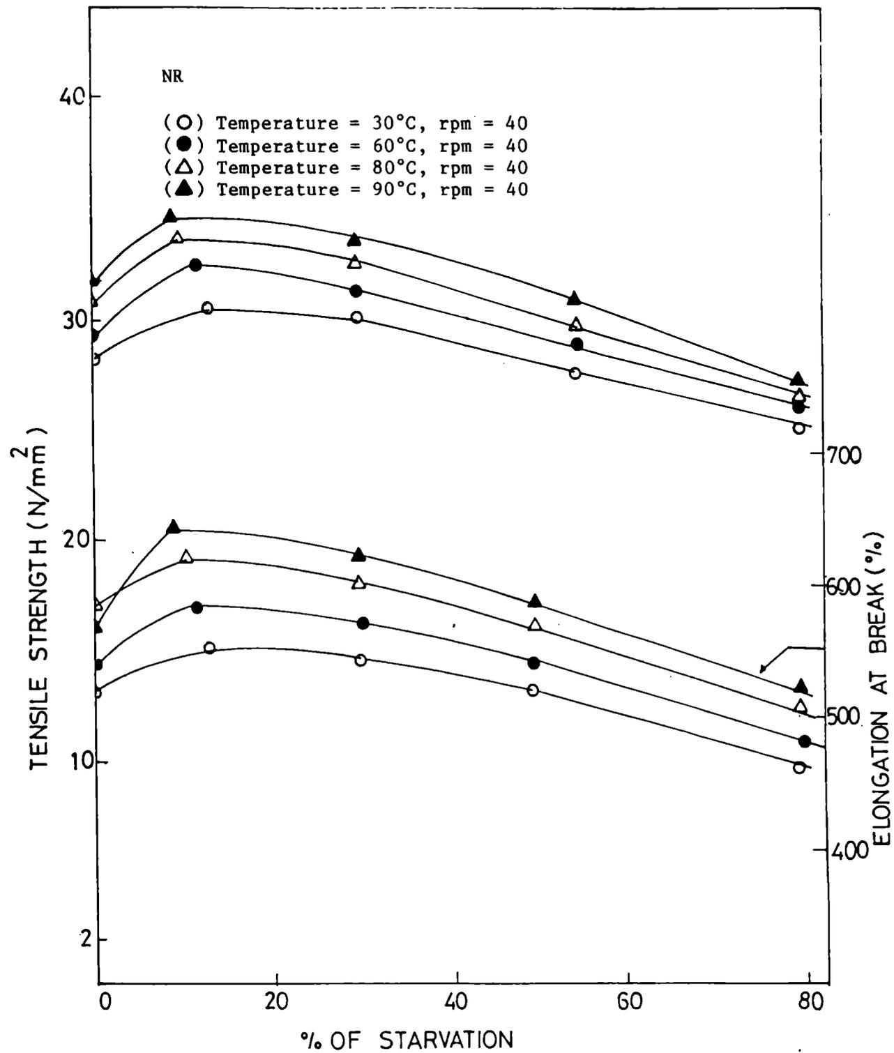
Fig.4.15: Variation of tensile strength and elongation at break of filled NR vulcanizates with percentage starvation at different temperatures.
