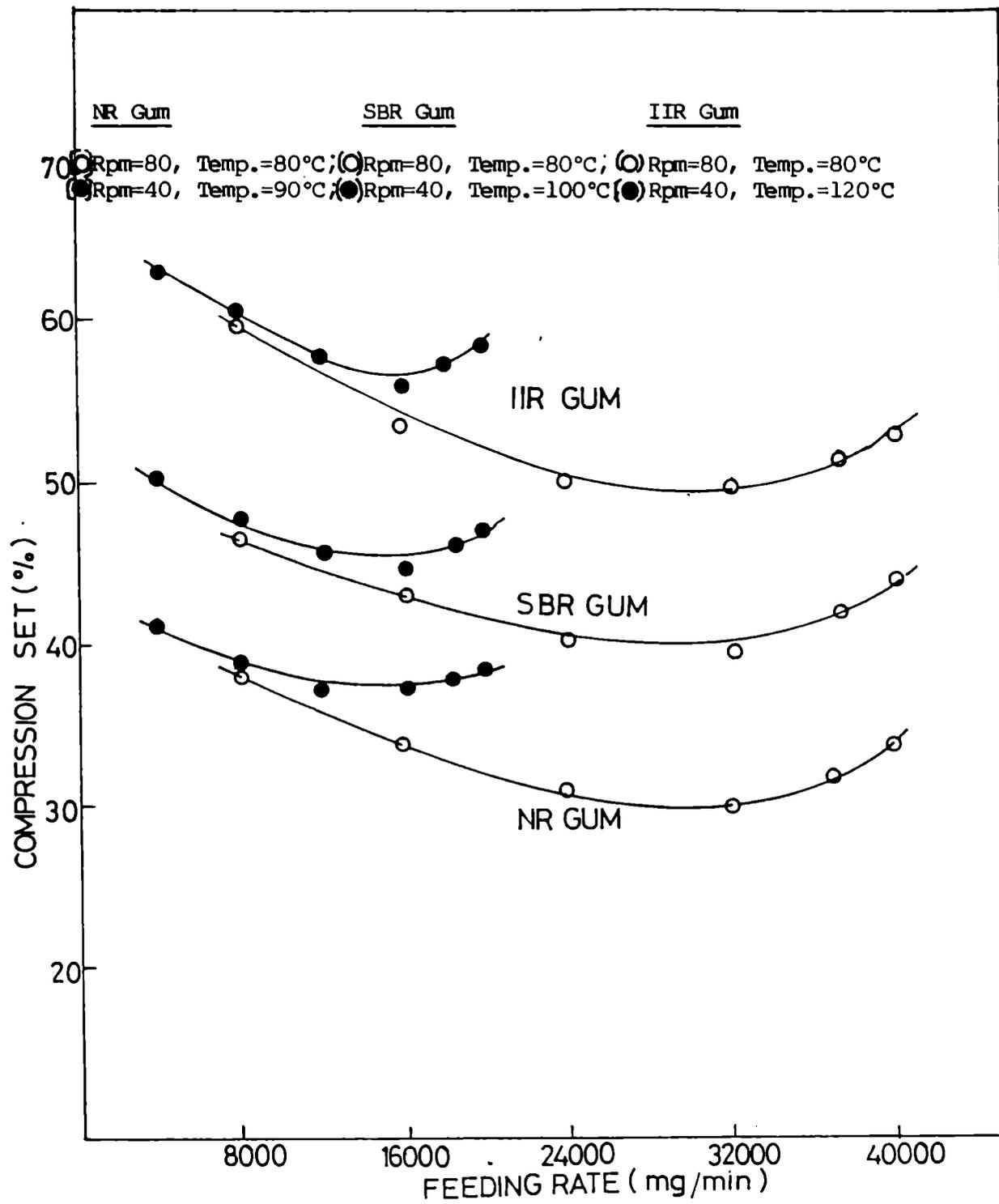
Fig.3.13: Variation of compression set of gum NR, SBR and IIR vulcanizates with feeding rate at different rpms and temperature.
