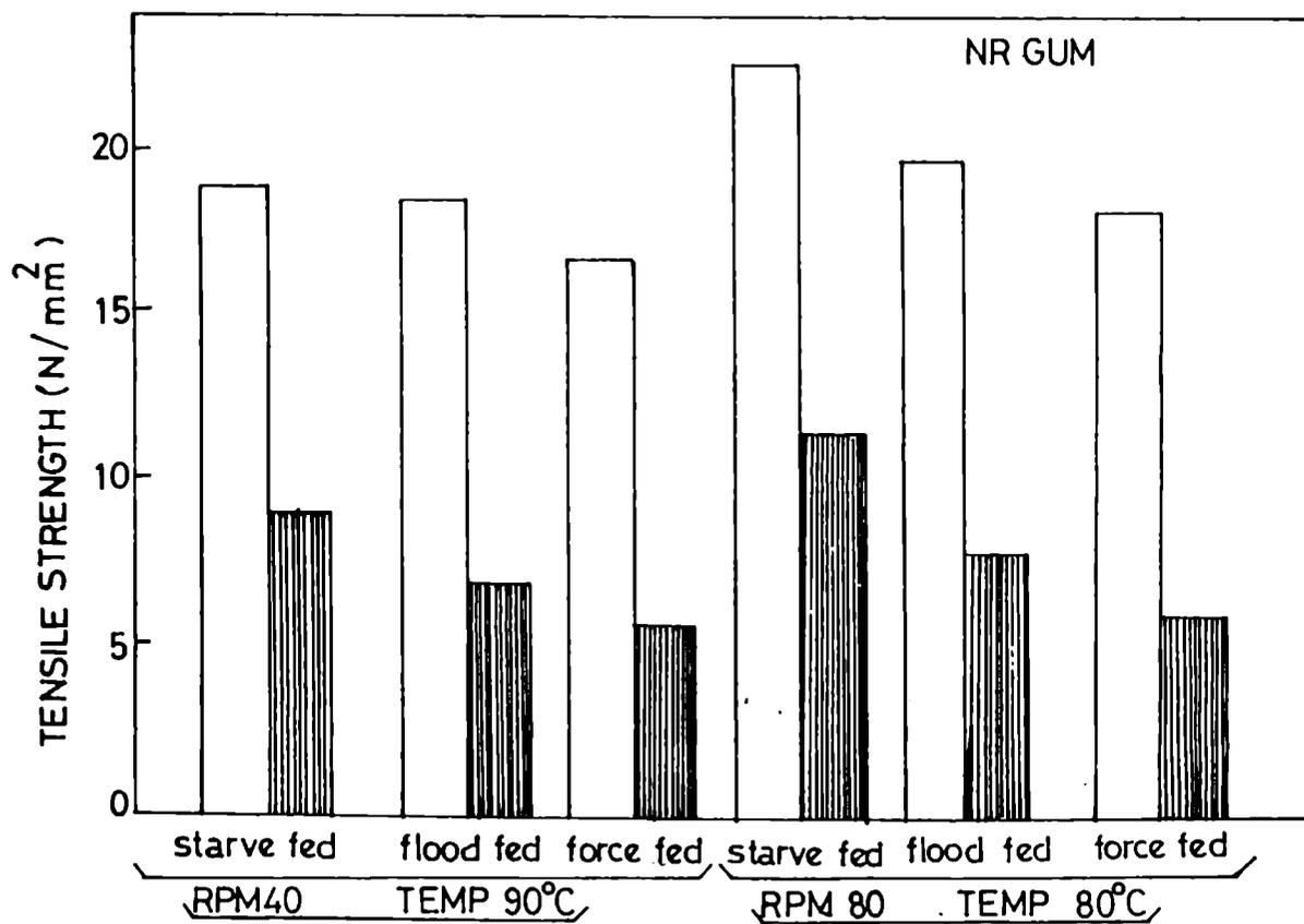
Fig.3.22: Variation of tensile strength and elongation at break of gum NR vulcanizates with different levels of feeding at different rpms and temperatures.
