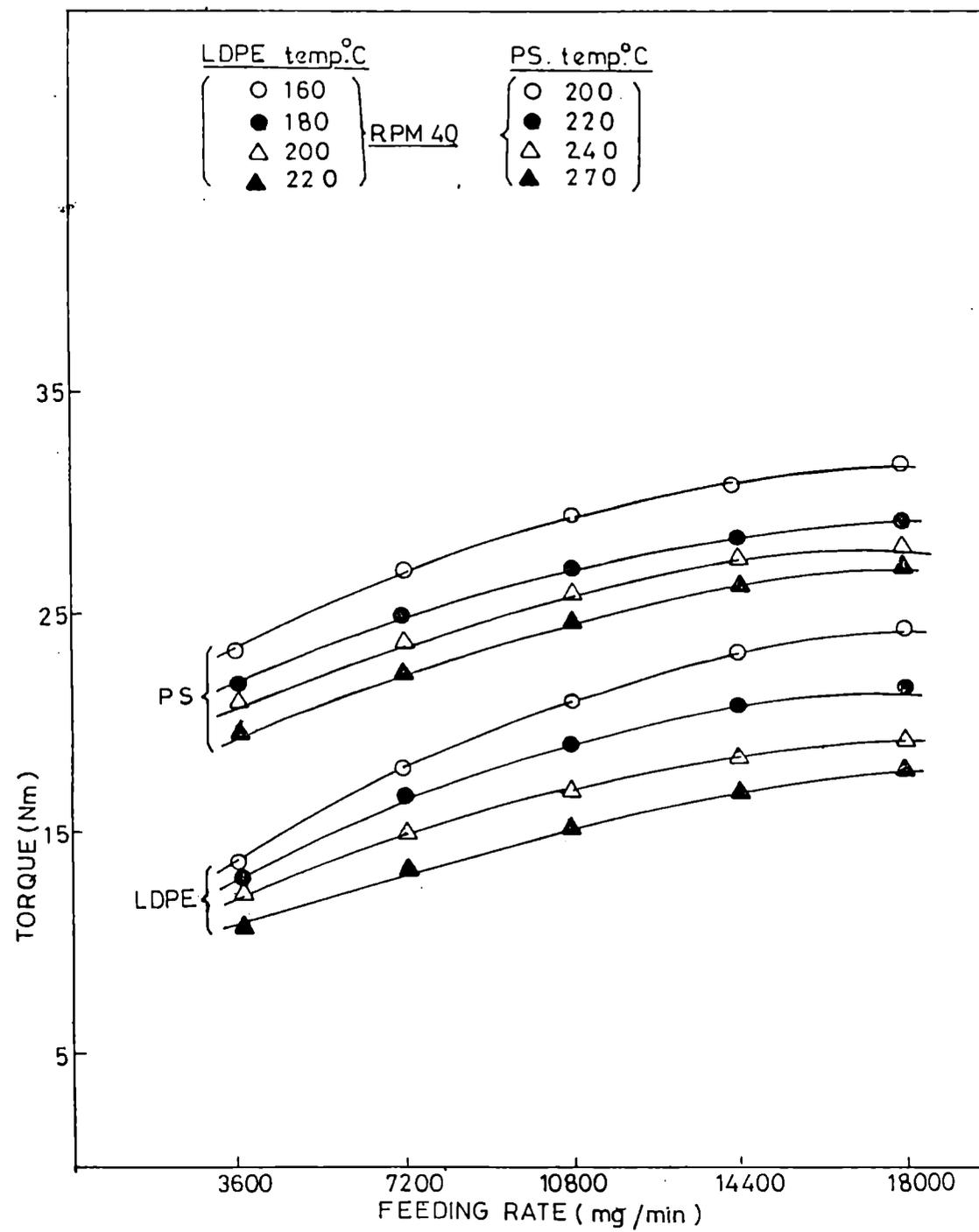
Fig.5.2: Variation of torque in the extrusion of LDPE and PS with feeding rate at different temperatures.
