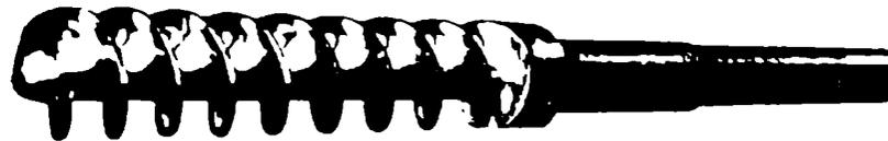
Fig.1.2b Screw of a conventional rubber extruder
