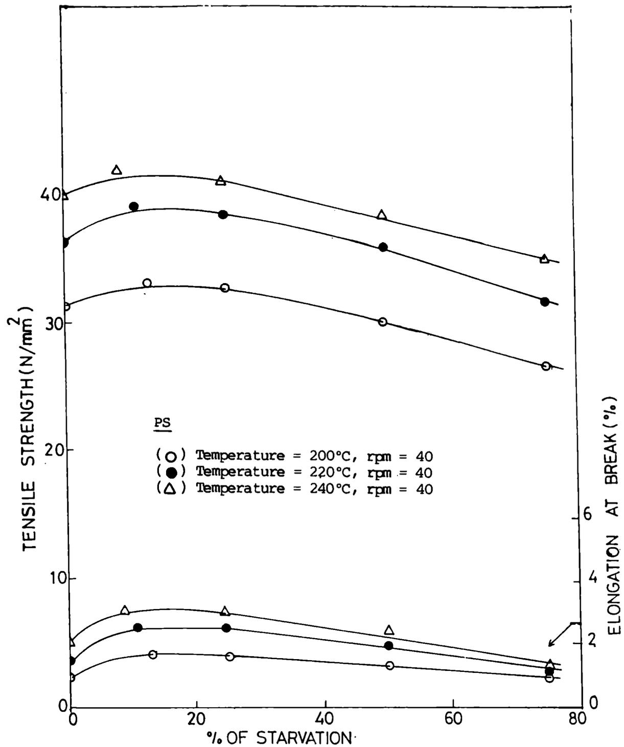
Fig.5.14: Variation of tensile strength and elongation at break of PS with percentage of starvation at different temperatures.
