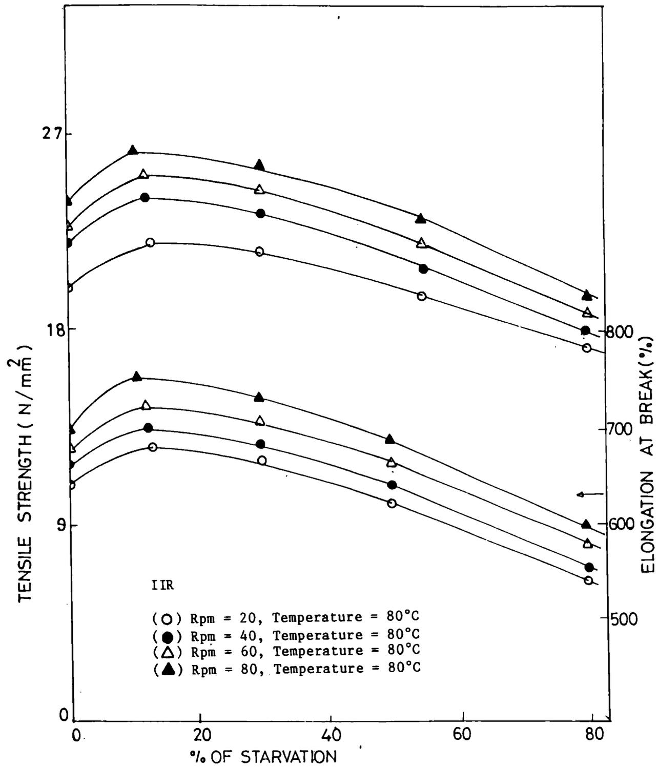
Fig.4.18: Variation of tensile strength and elongation at break of filled IIR vulcanizates with percentage starvation at different rpms.
