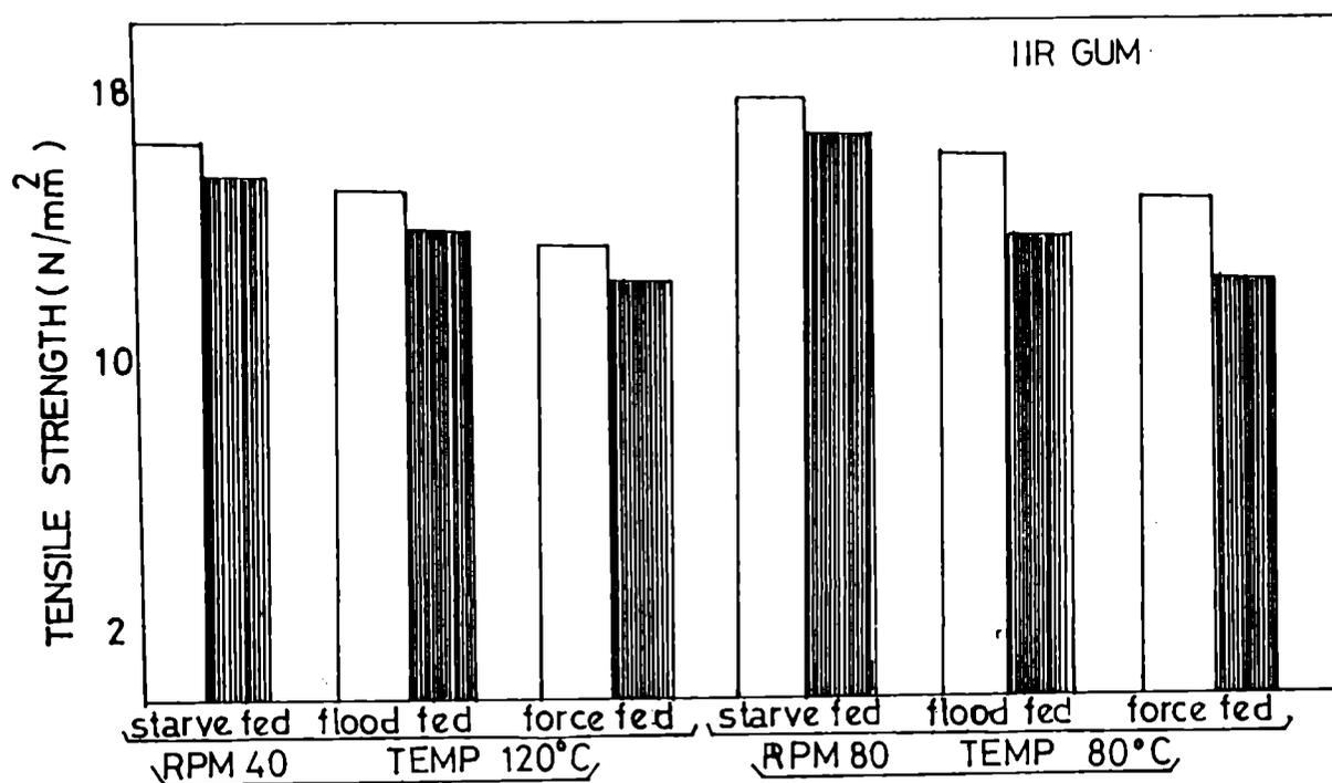
Fig.3.24: Variation of tensile strength and elongation at break of gum IIR vulcanizates with different levels of feeding at different rpms and temperatures.
