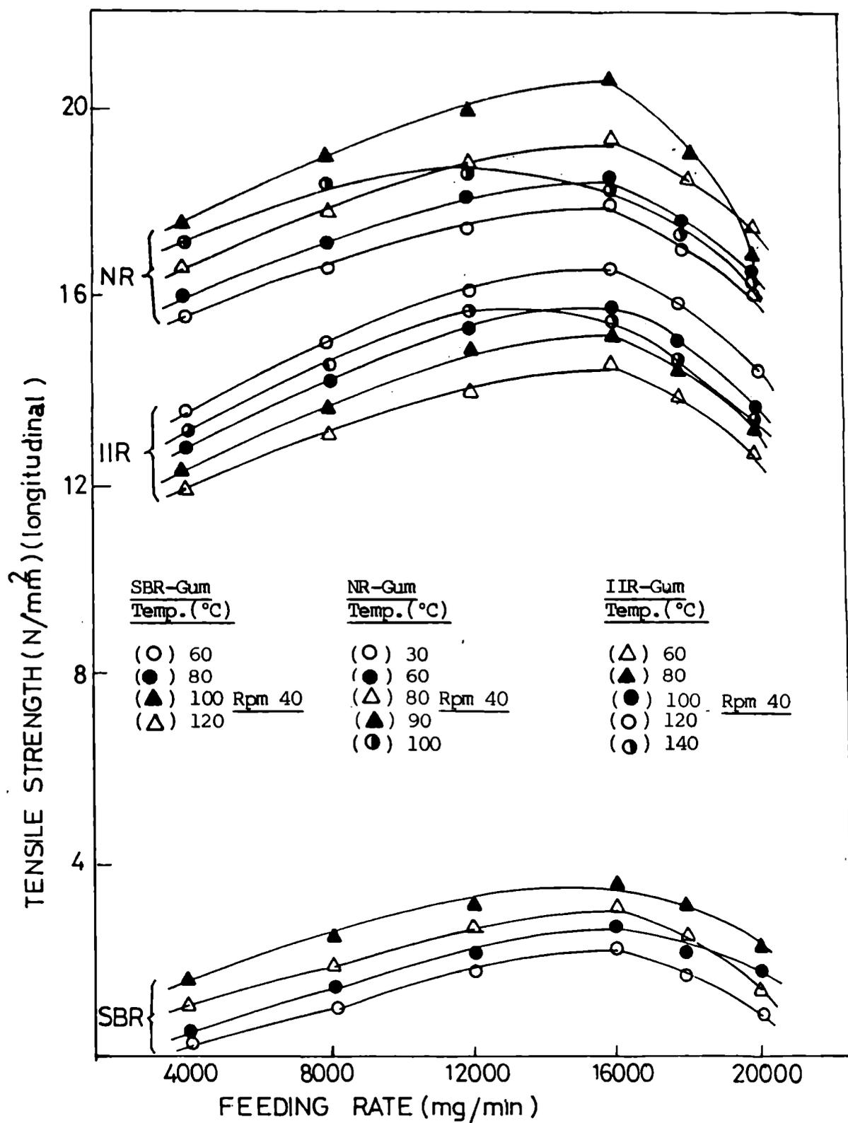
Fig.3.7: Variation of tensile strength of gum NR, SBR and IIR vulcanizates with feeding rate at different temperatures in the milling/extrusion direction.
