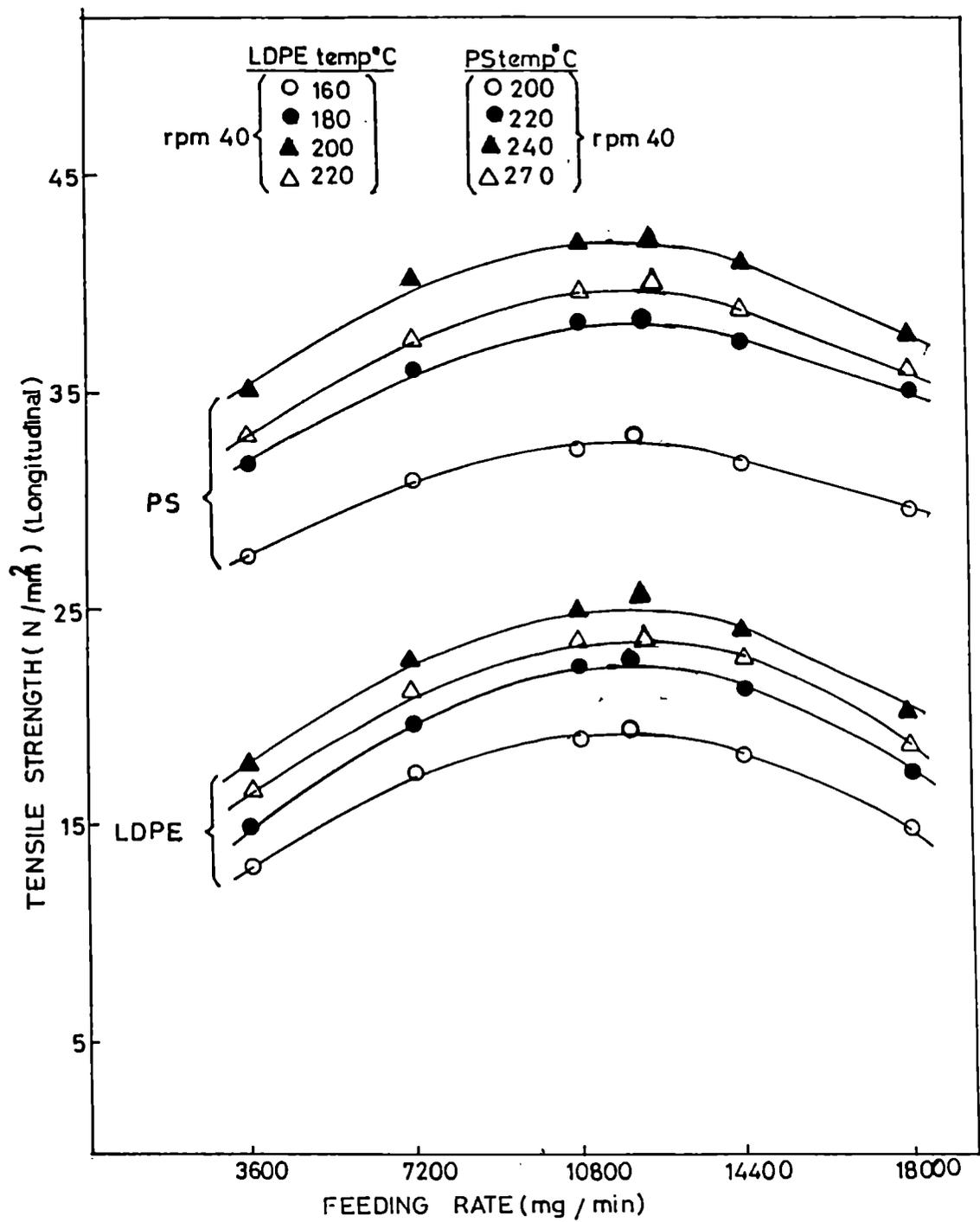
Fig.5.7: Variation of tensile strength of LDPE and PS with feeding rate at different temperatures in the extrusion direction.
