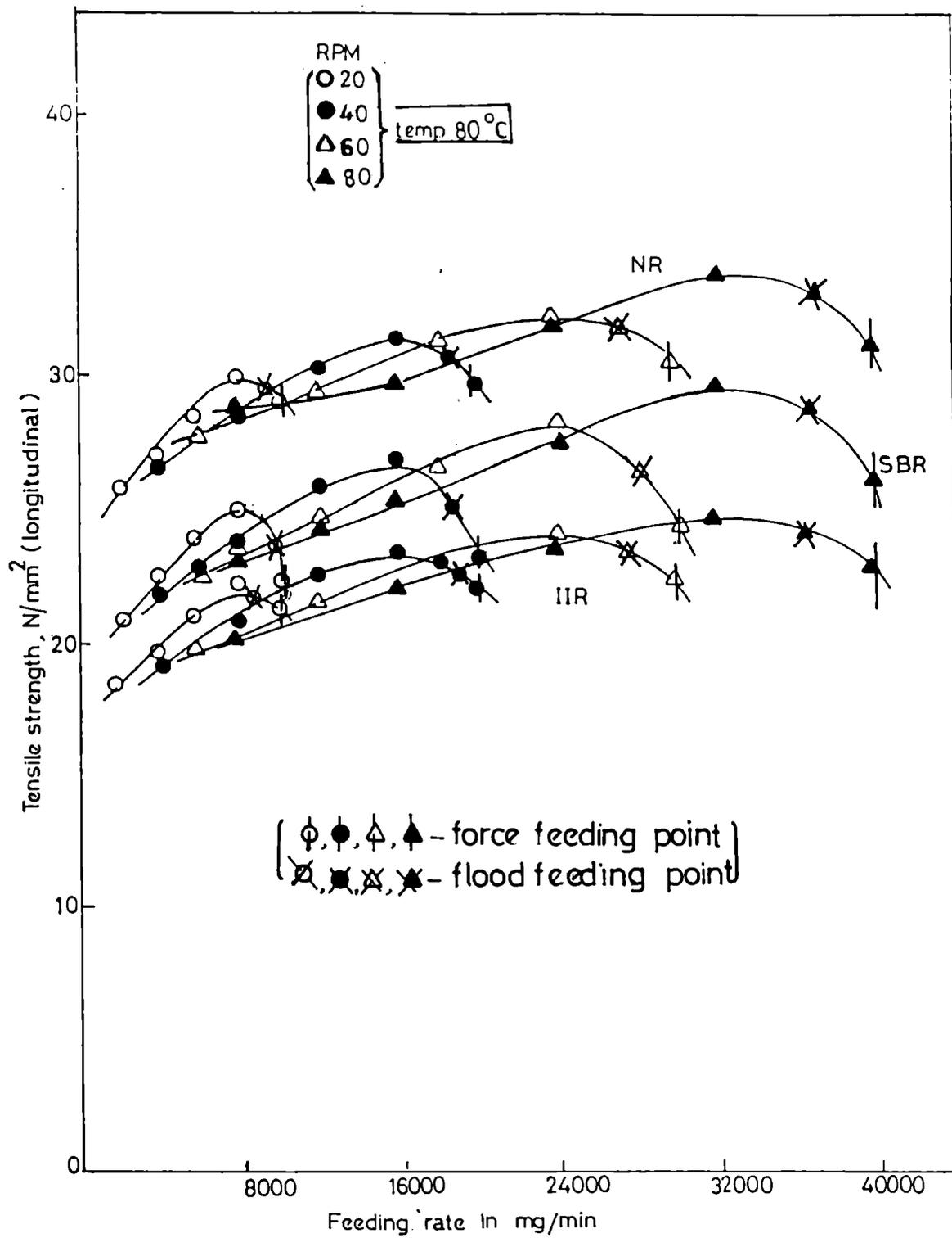
Fig.4.3: Variation of tensile strength of filled NR, SBR and IIR vulcanizates with feeding rate at different rpms in milling/extrusion direction.
