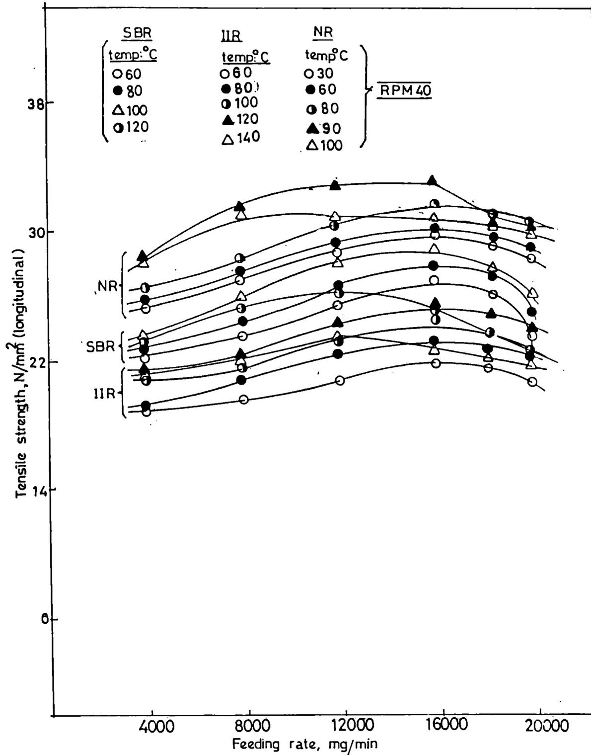
Fig.4.7: Variation of tensile strength of filled NR, SBR and IIR vulcanizates with feeding rate at different temperatures in the milling/extrusion direction.
