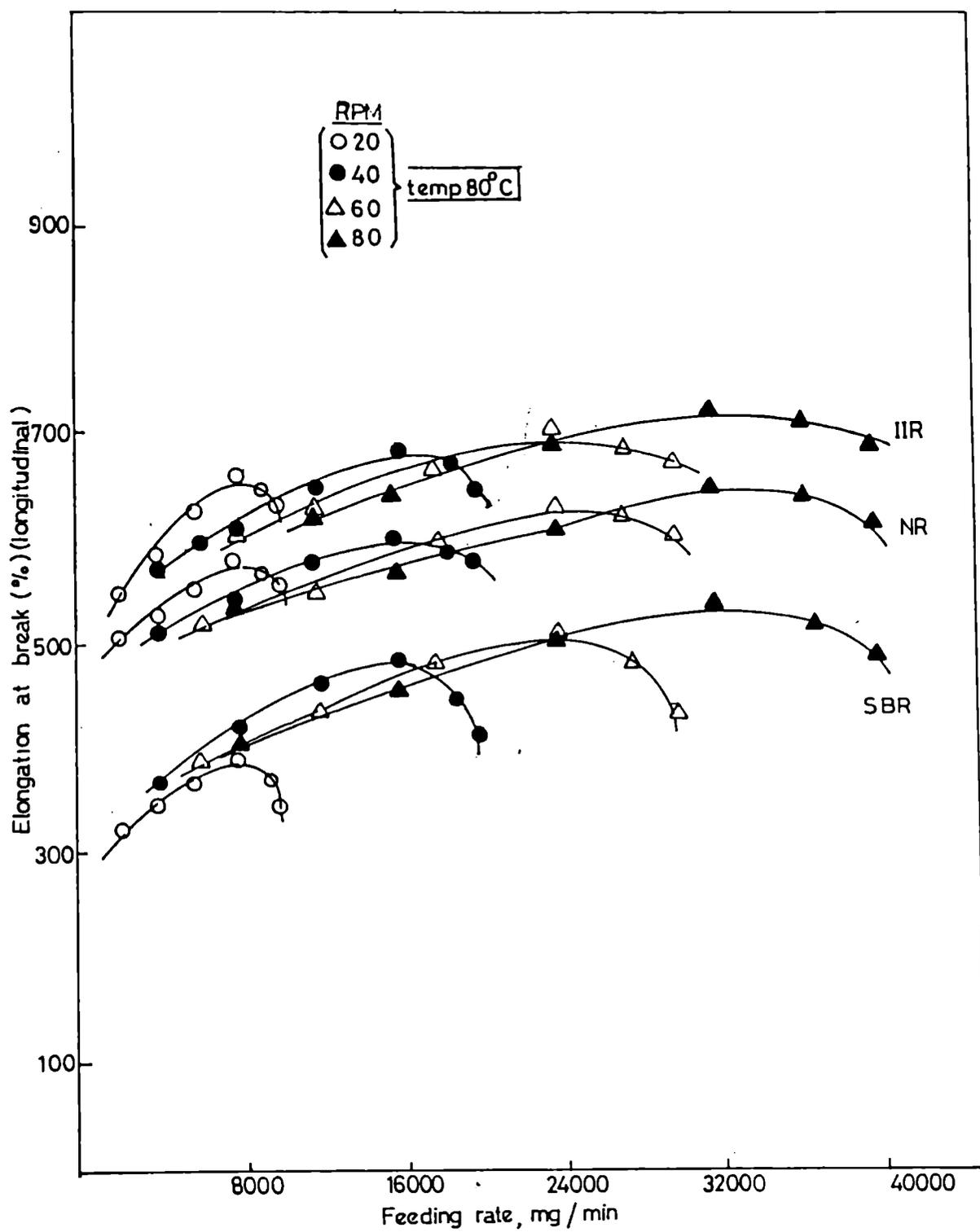
Fig.4.5: Variation of elongation at break of filled NR, SBR and IIR vulcanizates with feeding rate at different rpms in the milling/extrusion direction.
