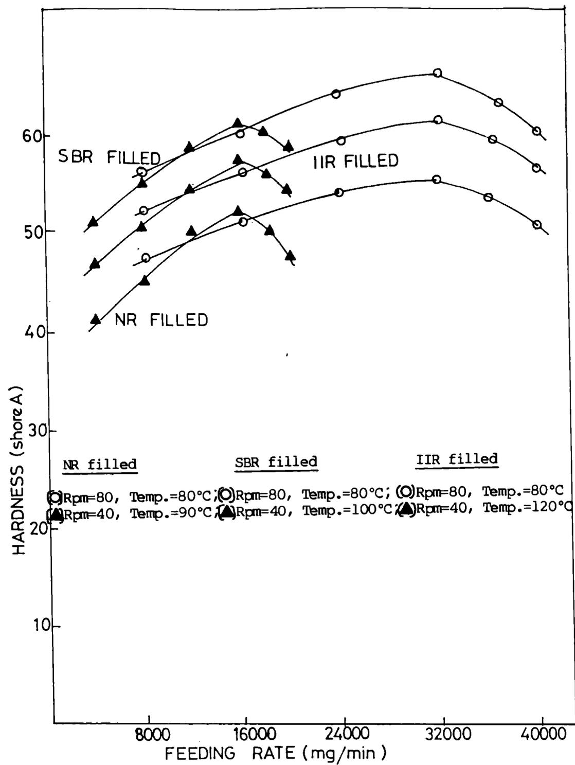
Fig.4.12: Variation of hardness of filled NR, SBR and IIR vulcanizates with feeding rate at different rpms and temperatures.
