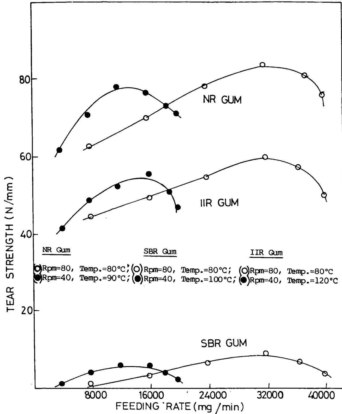
Fig.3.11: Variation of tear strength of gum NR, SBR and IIR vulcanizates with feeding rate at different rpms and temperatures.
