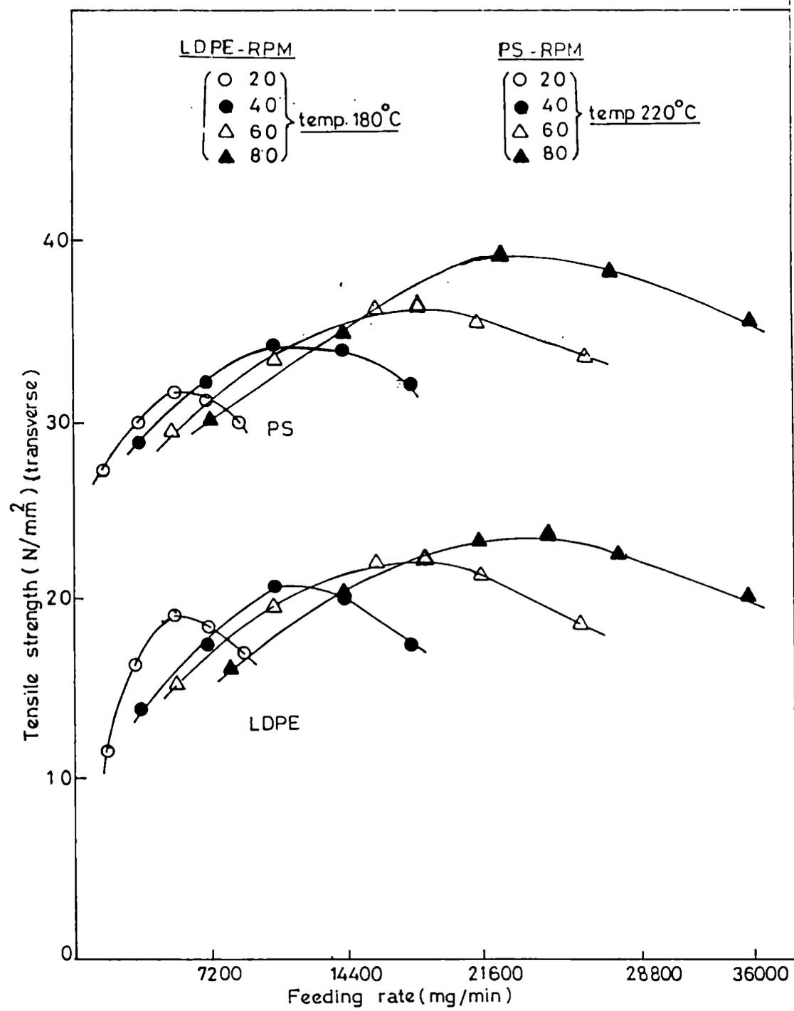
Fig.5.4: Variation of tensile strength of LDPE and PS with feeding rate at different rpm in the transverse direction.
