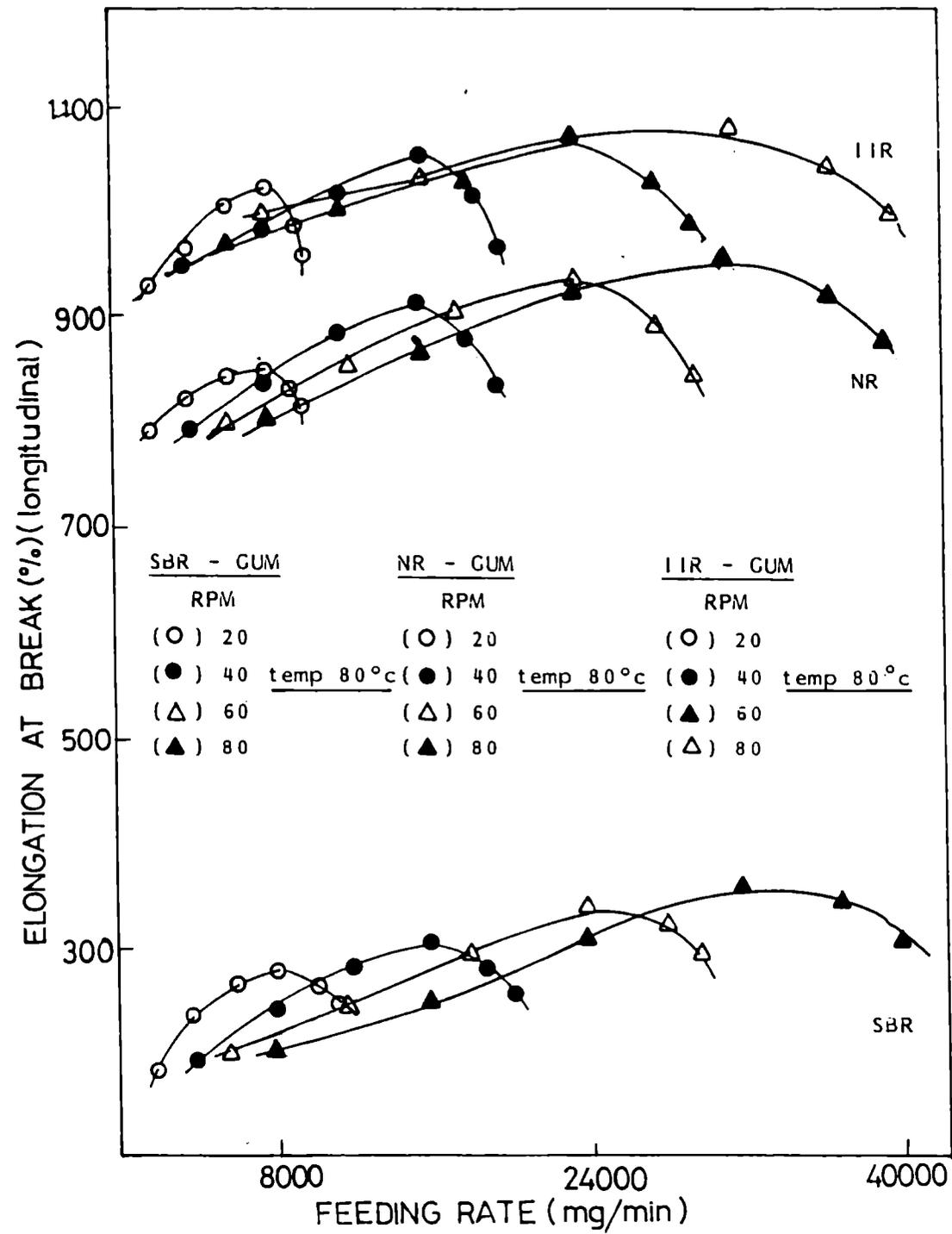
Fig.3.5: Variation of elongation at break of gum NR, SBR and IIR vulcanizates with feeding rate at different rpms in the milling/extrusion direction.
