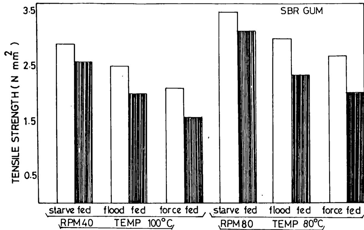
Fig.3.23: Variation of tensile strength and elongation at break of gum SBR vulcanizates with different levels of feeding at different rpms and temperatures.
