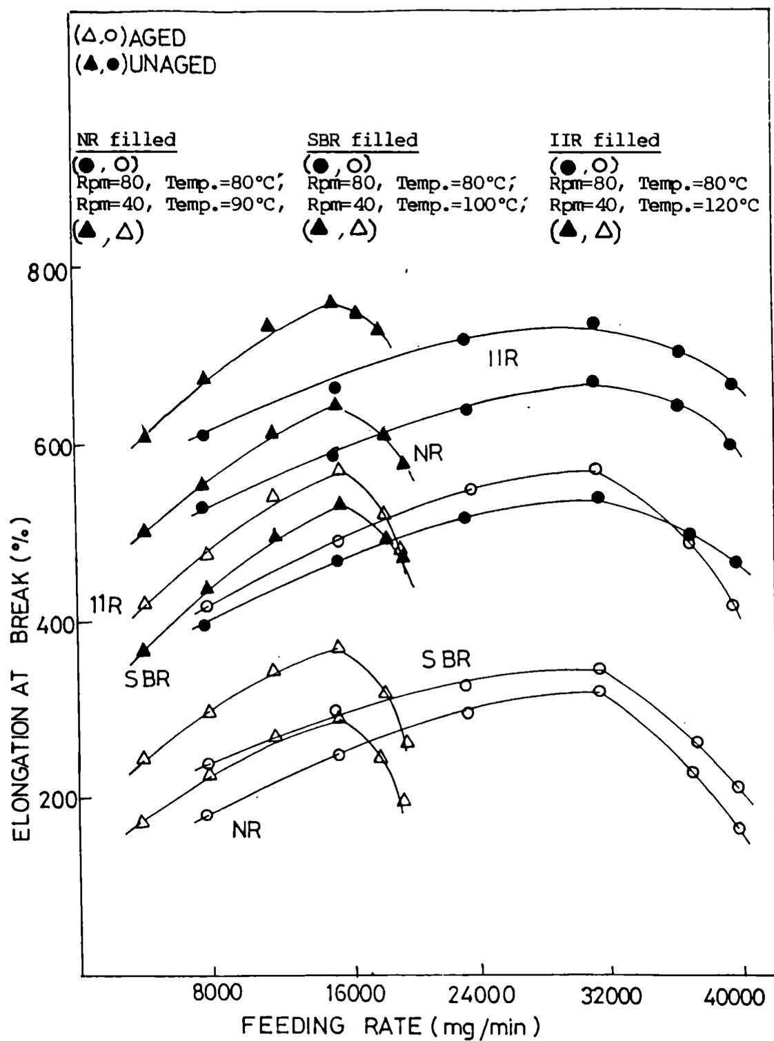
Fig.4.21: Variation of elongation at break of filled NR, SBR and IIR vulcanizates with feeding rate at different rpms and temperatures.
