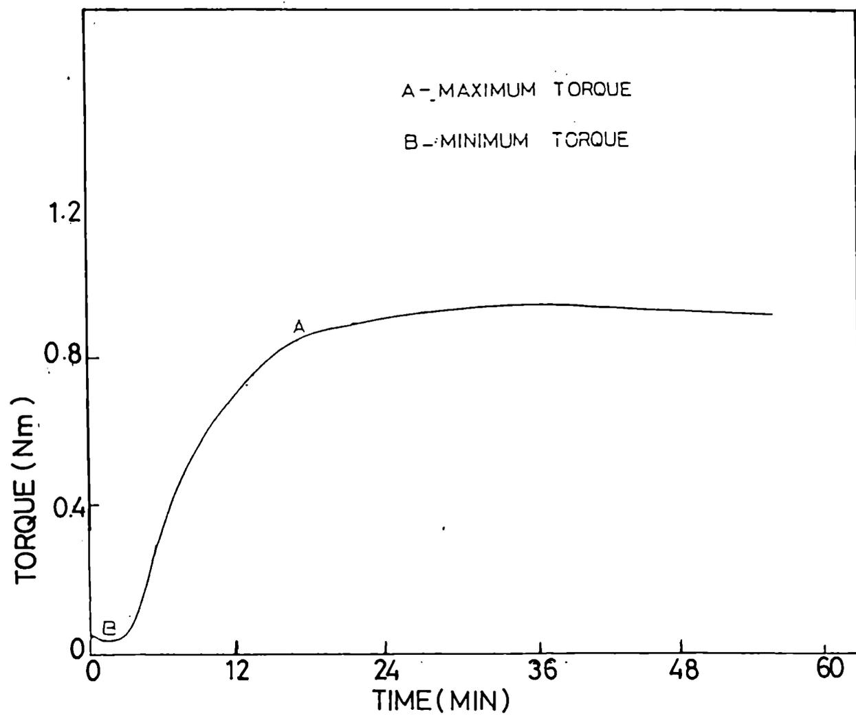
Fig.2.2: A typical cure curve of a rubber compound from elastograph.
