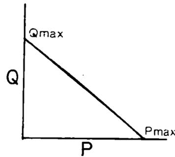
Fig.1.3 The extruder or screw characteristic
