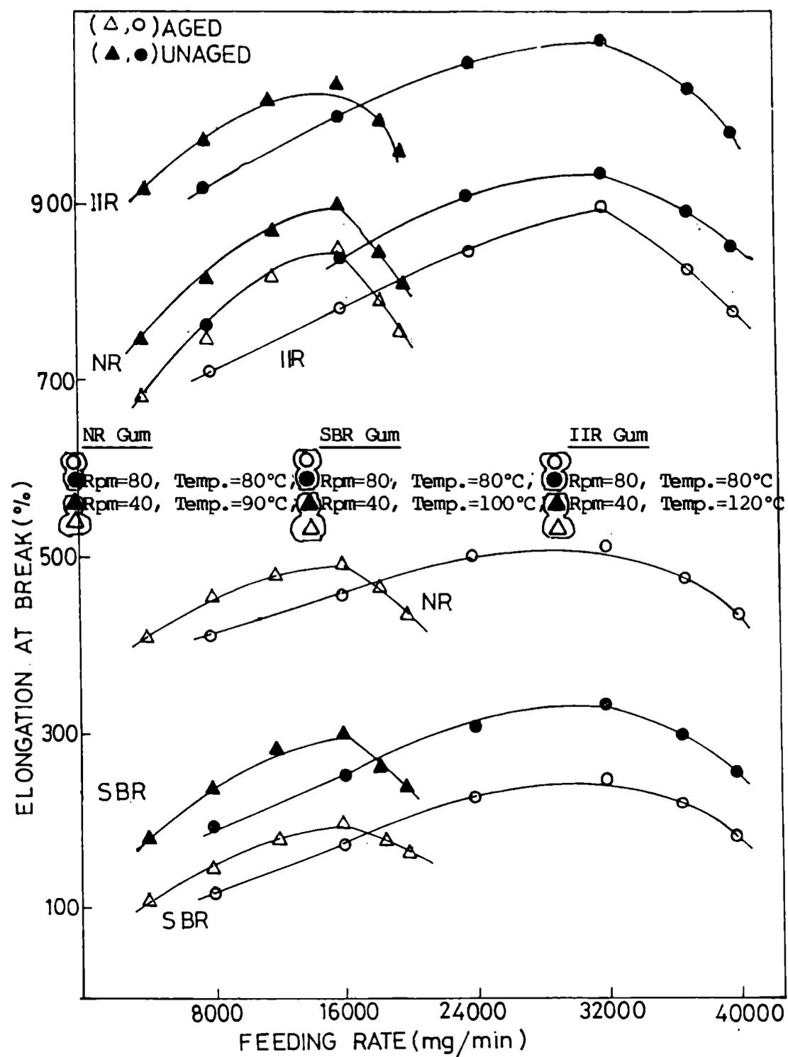
Fig.3.21: Variation of elongation at break of gum NR, SBR and IIR vulcanizates with feeding rate at different rpms and temperatures.
