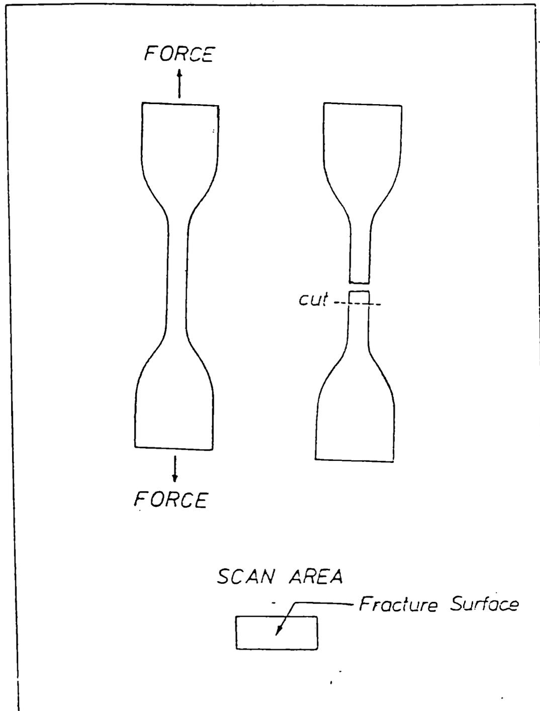
Fig.2.3: SEM scan area of the tensile fracture surface.
