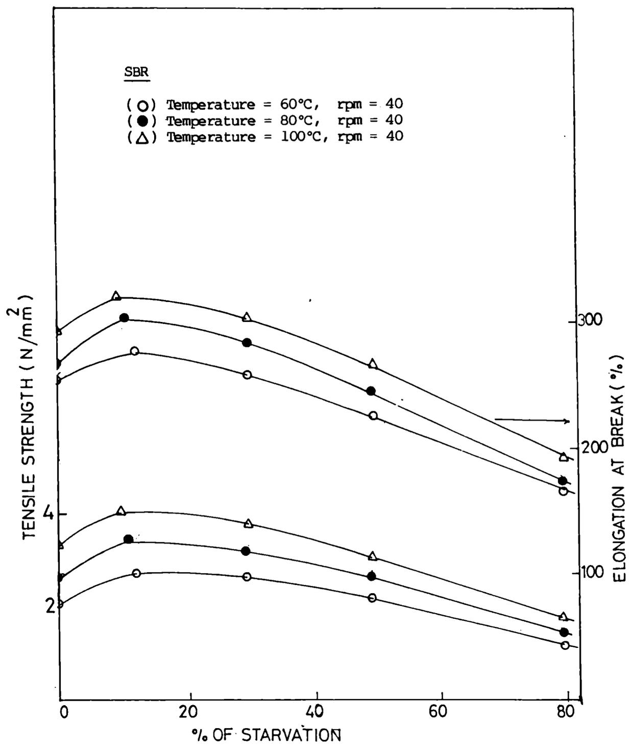
Fig.3.17: Variation of tensile strength and elongation at break of gum SBR vulcanizates with percentage starvation at different temperatures.
