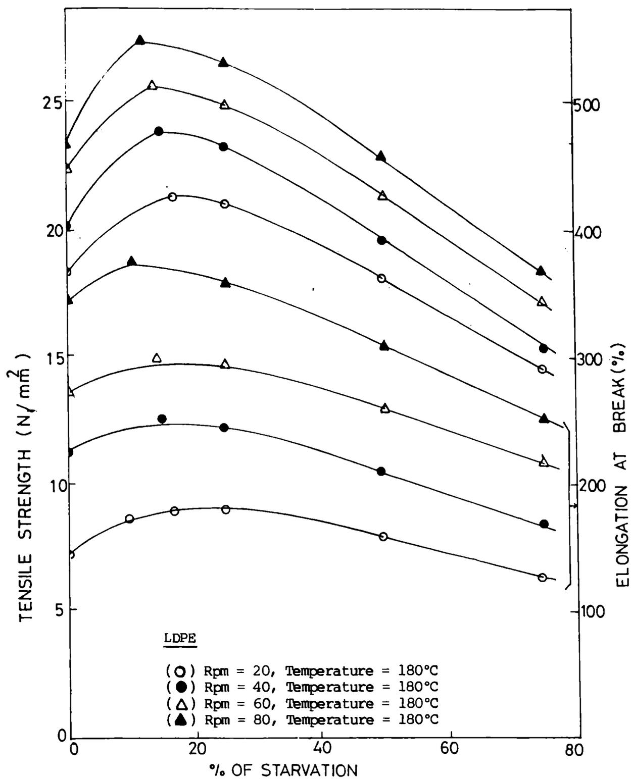
Fig.5.11: Variation of tensile strength and elongation at break of LDPE with percentage starvation at different rpm.
