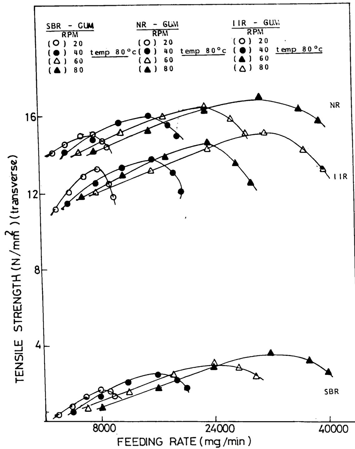
Fig.3.4: Variation of tensile strength of gum NR, SBR and IIR vulcanizates with feeding rate at different rpms in transverse direction.
