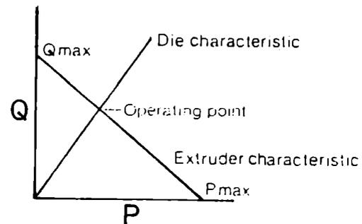
Fig.1.4: Interaction of screw and die characteristics
