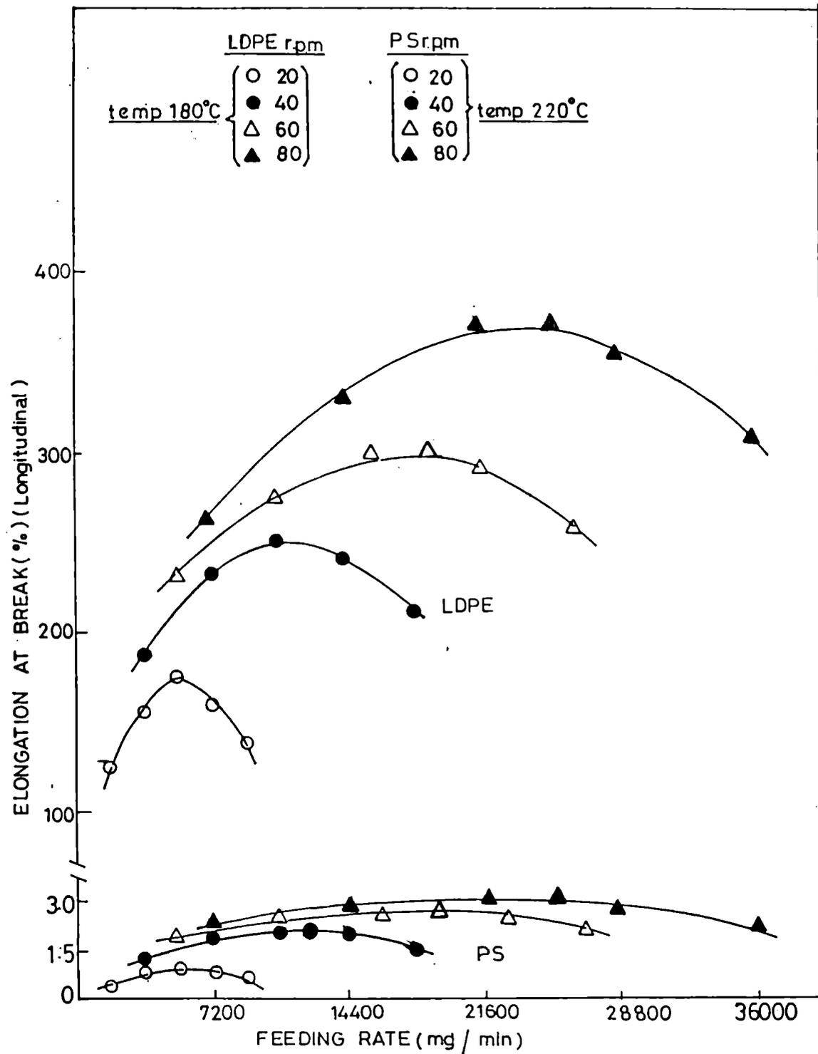
Fig.5.5: Variation of elongation at break of LDPE and PS with feeding rate at different rpm in the extrusion direction.
