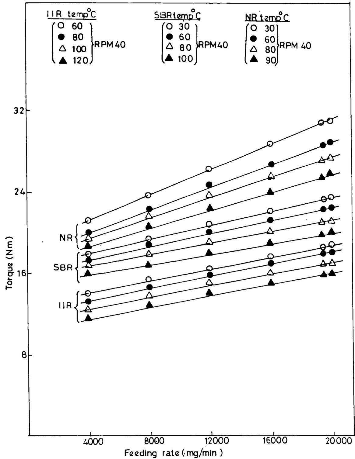
Fig.3.2: Variation of torque in the extrusion of gum NR, SBR and IIR compounds with feeding rate at different temperatures.
