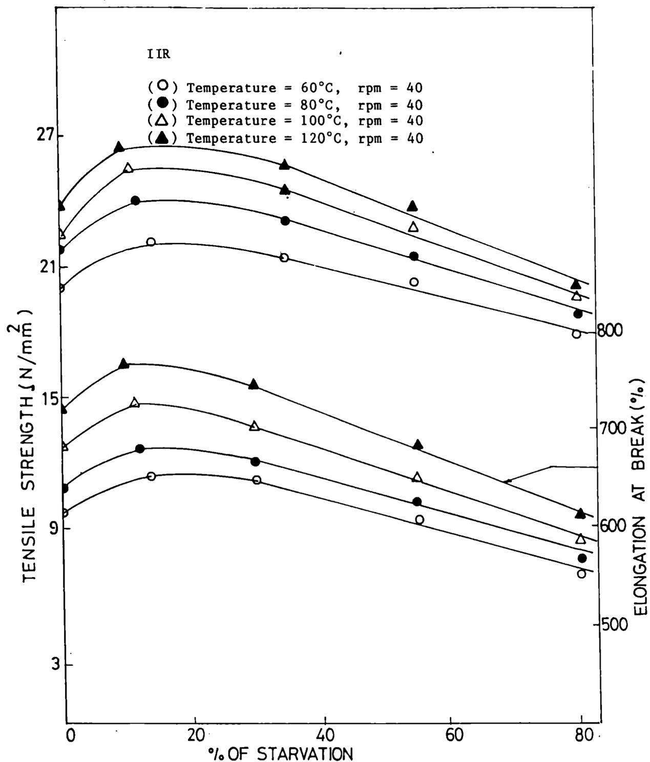
Fig.4.19: Variation of tensile strength and elongation at break of filled IIR vulcanizates with percentage starvation at different temperatures.
