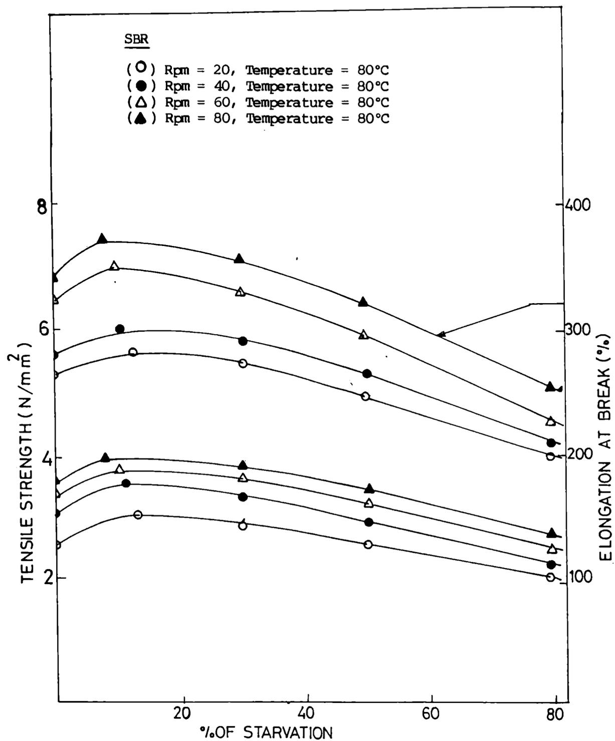
Fig.3.16: Variation of tensile strength and elongation at break of gum SBR vulcanizates with percentage starvation at different rpms.
