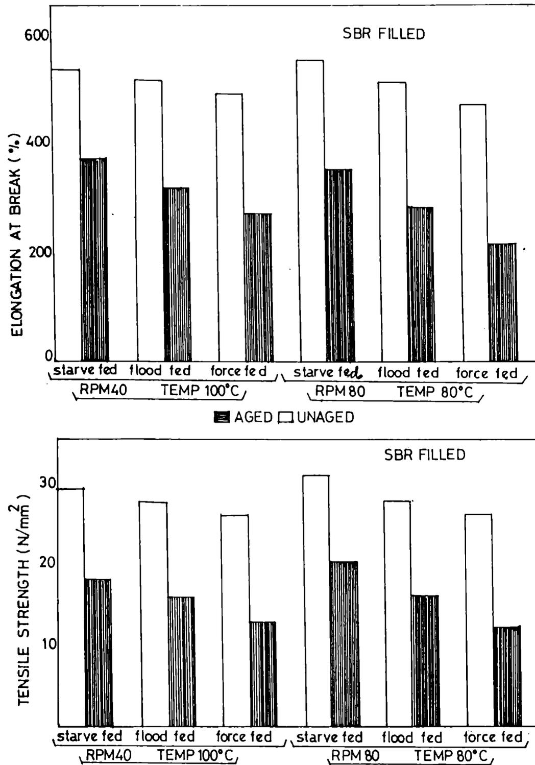
Fig.4.23: Variation of tensile strength and elongation at break of filled SBR vulcanizates with different levels of feeding at different rpms and temperatures.
