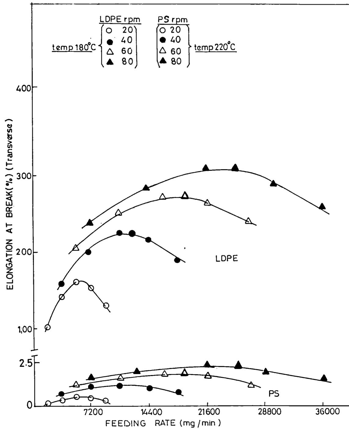
Fig.5.6: Variation of elongation at break of LDPE and PS with feeding rate at different rpm in the transverse direction.
