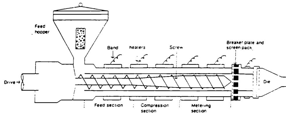
Fig.1.1 A screw extruder
