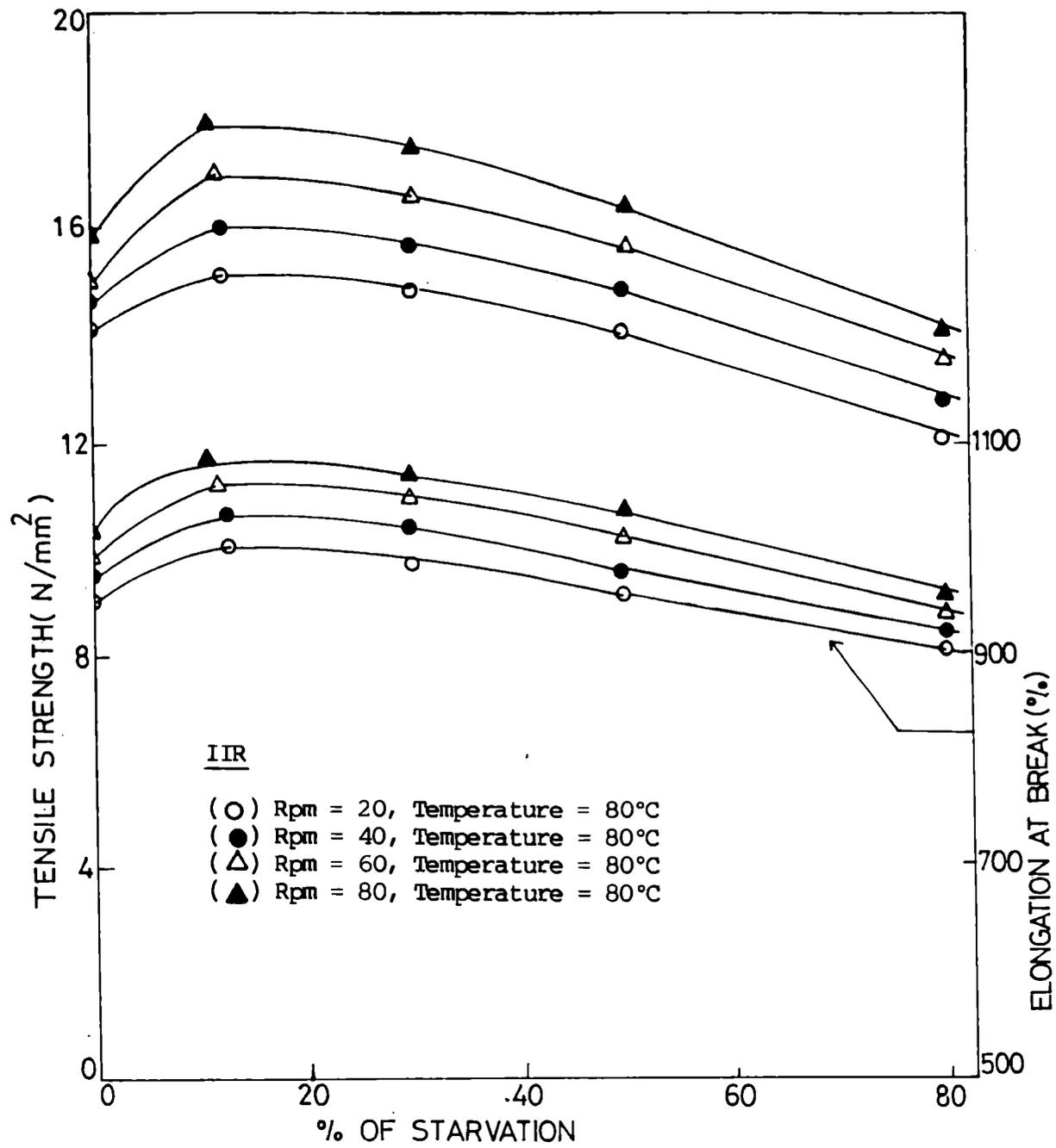
Fig.3.18: Variation of tensile strength and elongation at break of gum IIR vulcanizates with percentage starvation at different rpms.
