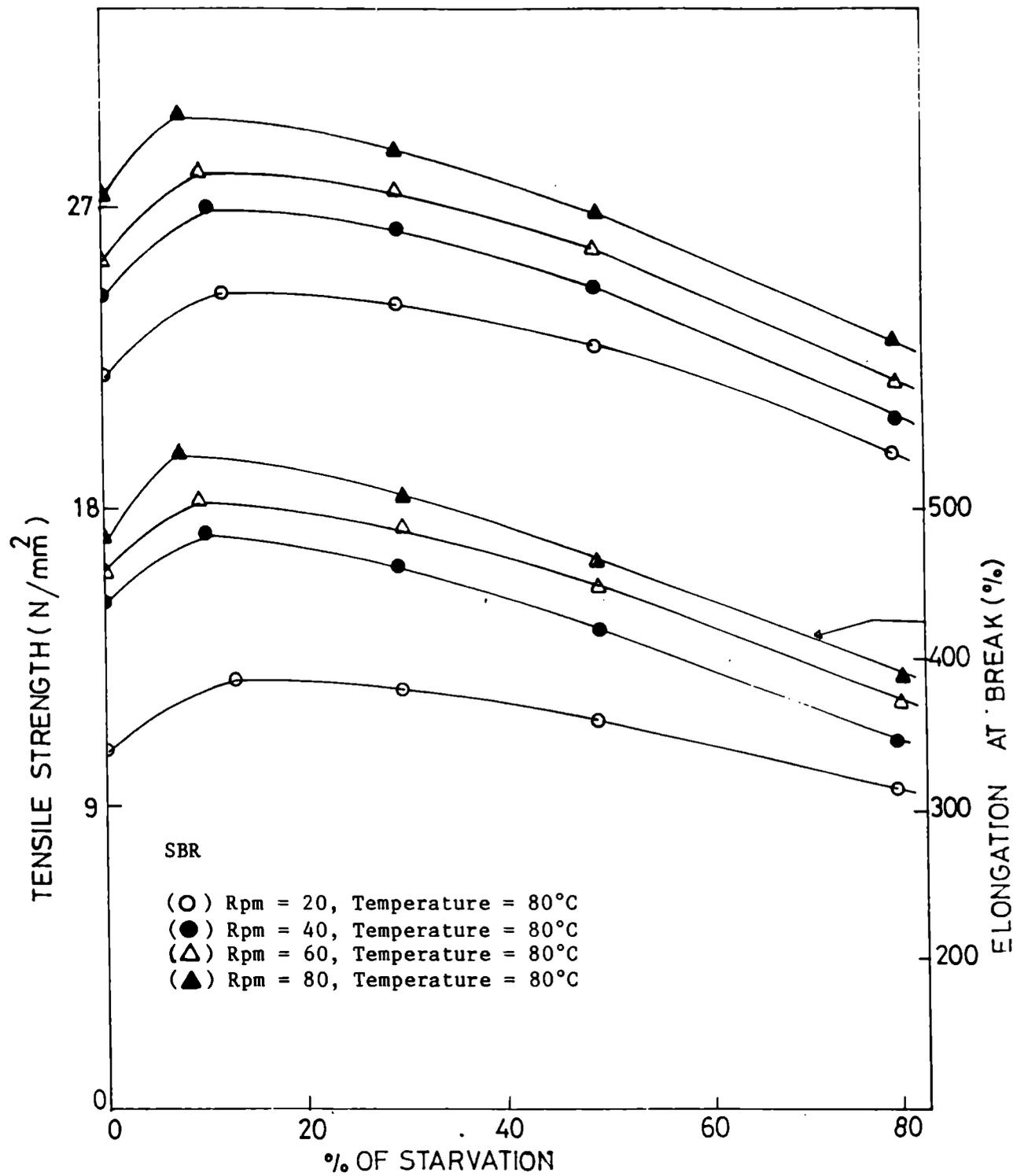
Fig.4.16: Variation of tensile strength and elongation at break of filled SBR vulcanizates with percentage starvation at different rpms.
