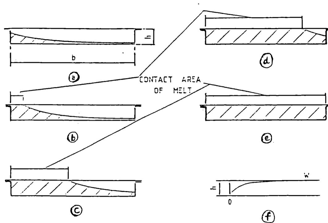
Fig. 1.6 Melt cross-section of partially filled channels
