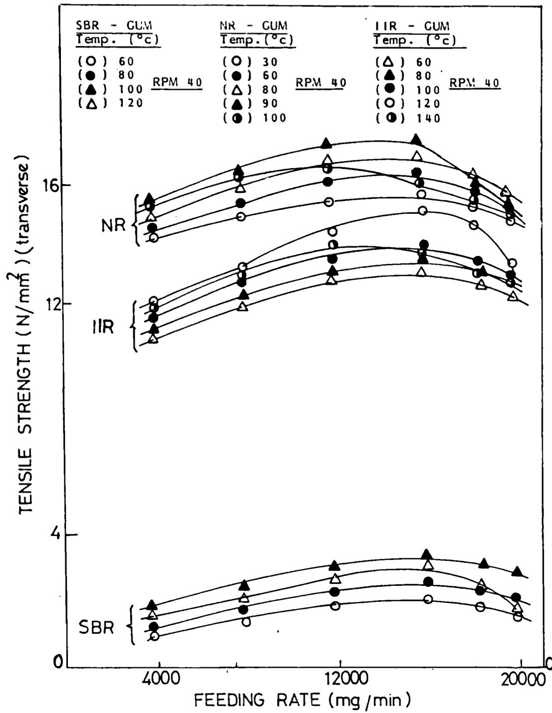
Fig.3.8: Variation of tensile strength of gum NR, SBR and IIR vulcanizates with feeding rate at different temperatures in the transverse direction.
