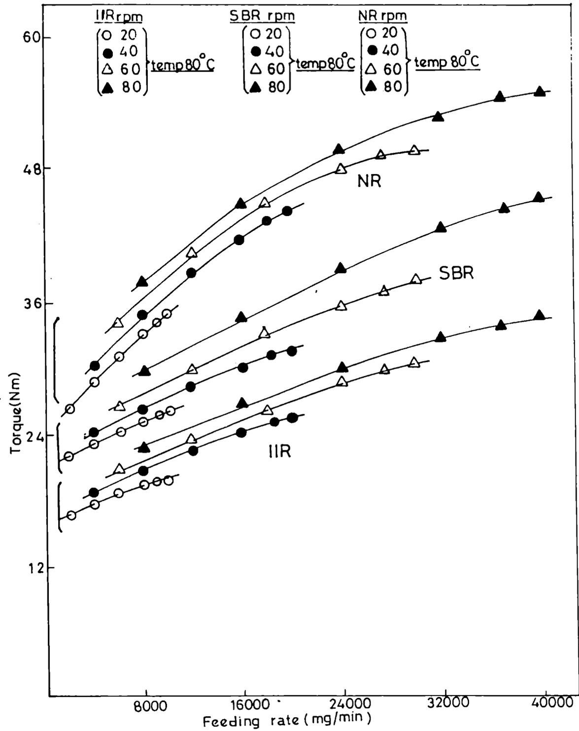
Fig.4.1: Variation of torque in the extrusion of filled NR, SBR and IIR compounds with feeding rate at different rpms.
