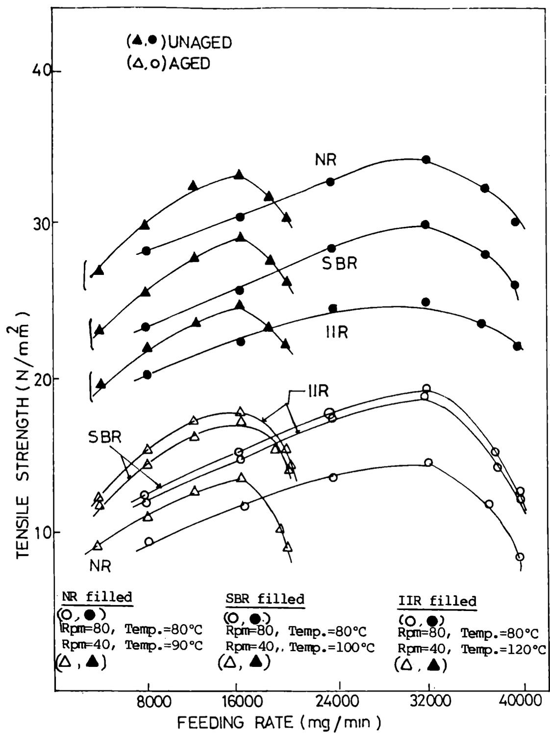
Fig.4.20: Variation of tensile strength of filled NR, SBR and IIR vulcanizates with feeding rate at different rpms and temperatures.
