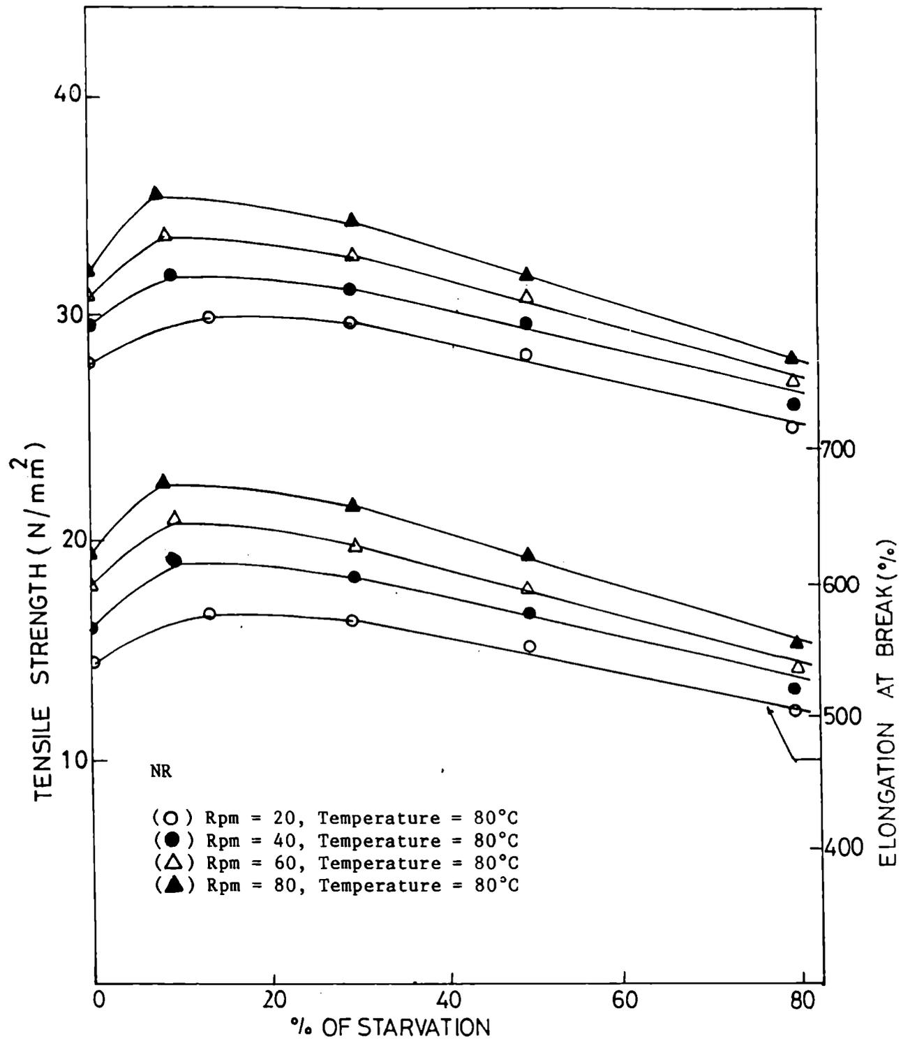
Fig.4.14: Variation of tensile strength and elongation at break of filled NR vulcanizates with percentage starvation at different rpms.
