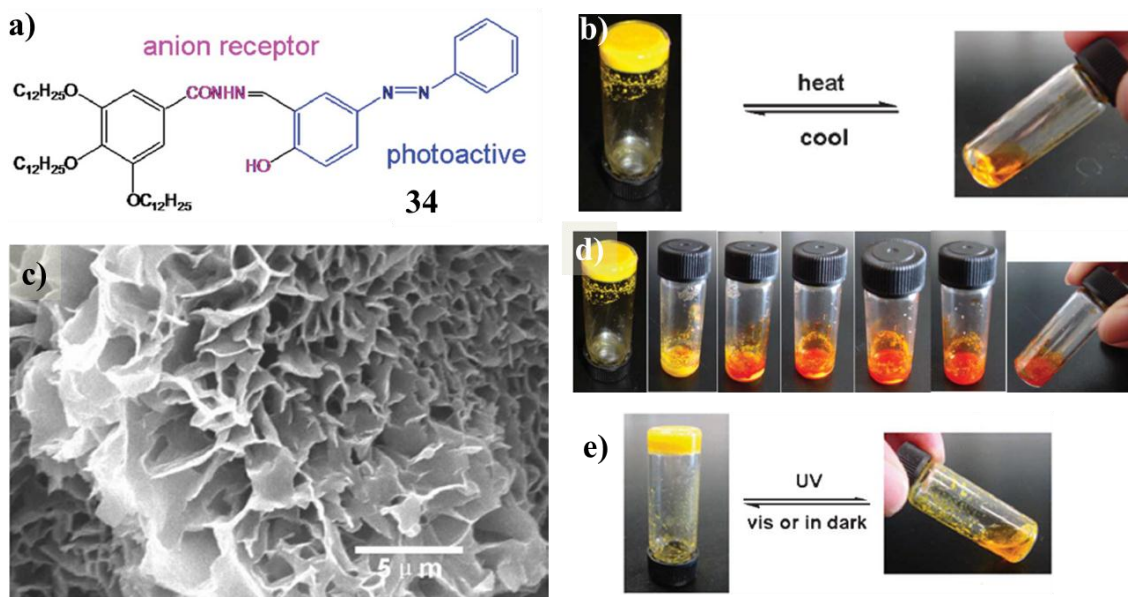
Figure 1.17. (a) Chemical structure of 34 . (b) Organogel formed by heating-cooling of 34 in DMF. (c) SEM image of the xerogel 34 . (d) Organogels formed from a solution of 34 in DMF after addition of solid tetrabutylammonium phosphate salt (1 eqv.) at different time intervals from 0 to 10 min. (e) Organogel formed from a solution of 1% 34 with \alpha -CD in DMF in the dark or vis irradiation.
