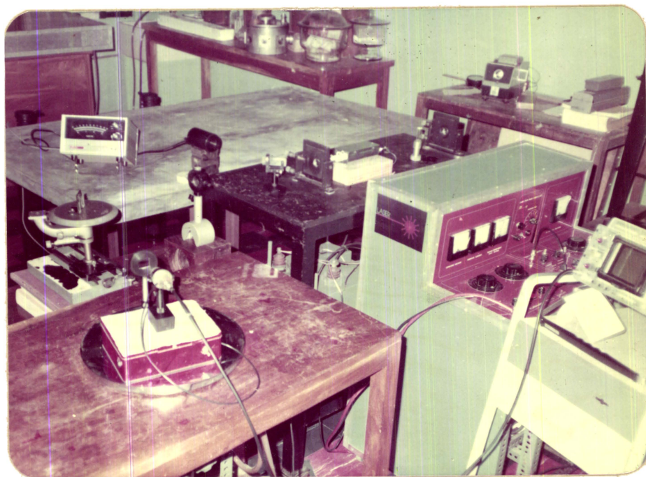
Fig.3.1B Laser-induced damage threshold measurement set-up.
