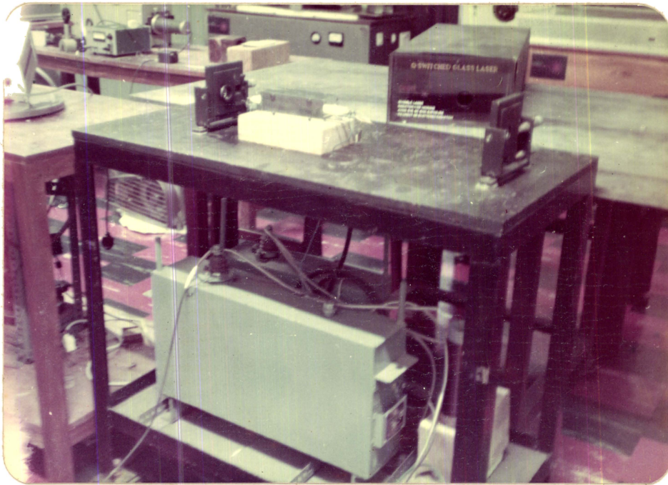
Fig.1.2B Conventional mode glass laser resonator.
