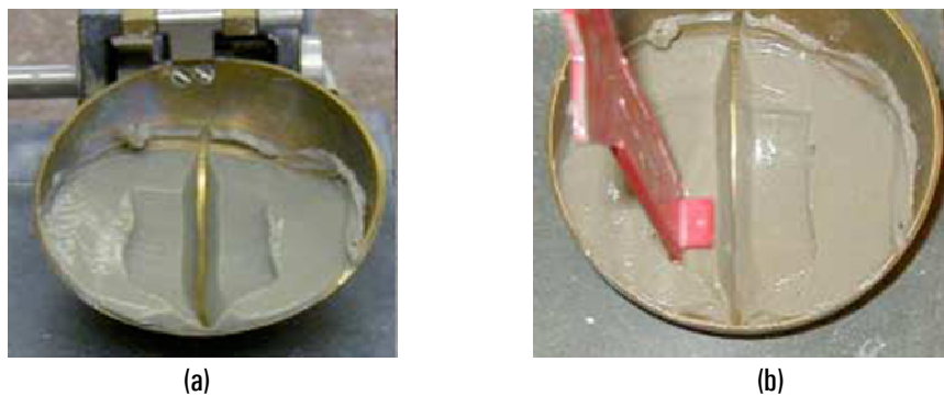
Figure 3.4 – (a) Groove separating two halves of the soil pat, (b) blow counts stopped after the groove closes by about 12mm size.
