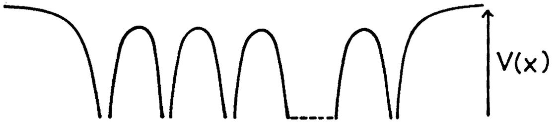
Fig.1.2 : Periodic potential due to the atomic core in a crystalline solid.
