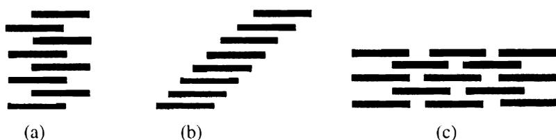
*Figure 2.2:* Schematic representation of the different arrangement of dyes in the solid surface and in solution. (a) ladder type, (b) staircase type and (c) brickwork type.
