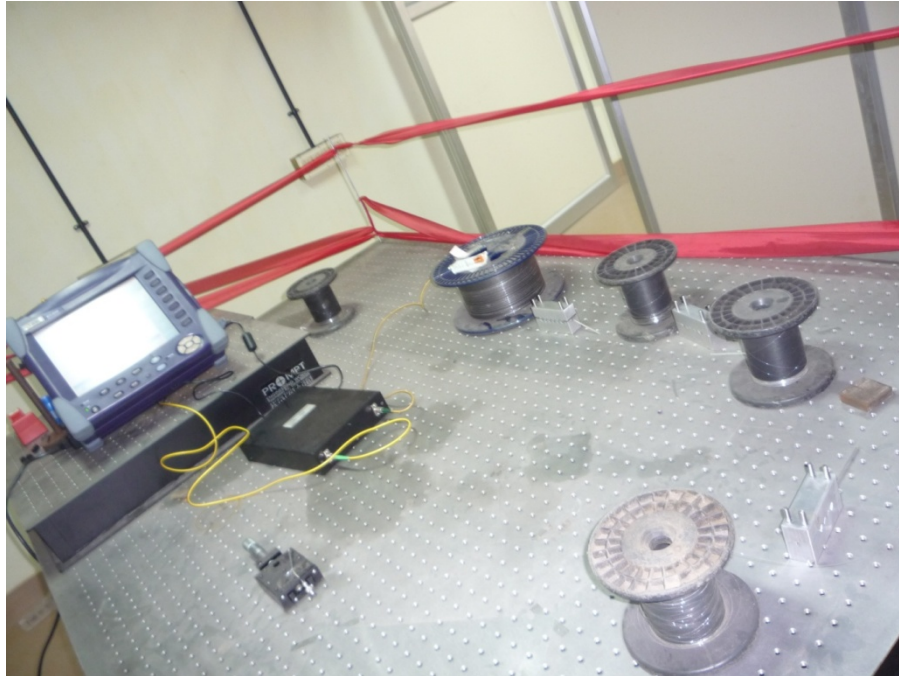
Figure 6.4 Photograph of the experimental set up for the distributed sensing
