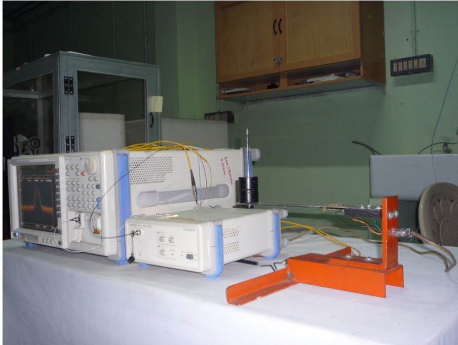
Figure 4.17 Photograph of the experimental set up for characterising FBG sensors
