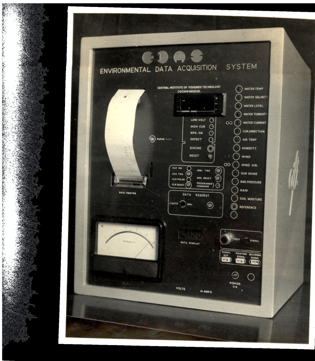
Fig 47 PHOTOGRAPH OF THE DATA PROCESSING/DISPLAY UNIT OF ENVIRONMENTAL DATA ACQUISITION SYSTEM
