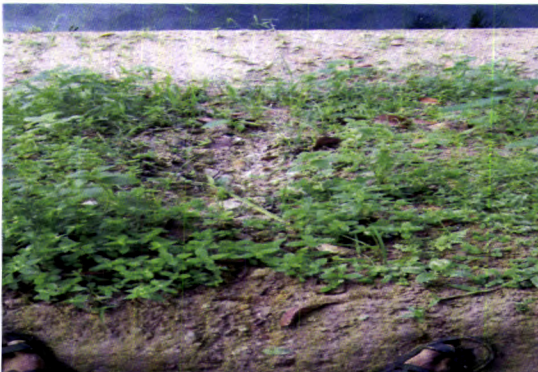
Figure 6.17. CP, less density, non uniform vegetation with soil erosion, after 7 months
