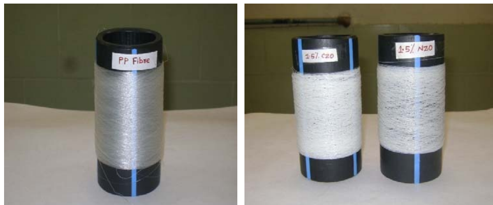
Figure 4.3: Photographs of neat PP and PP/ZnO composite fibers
