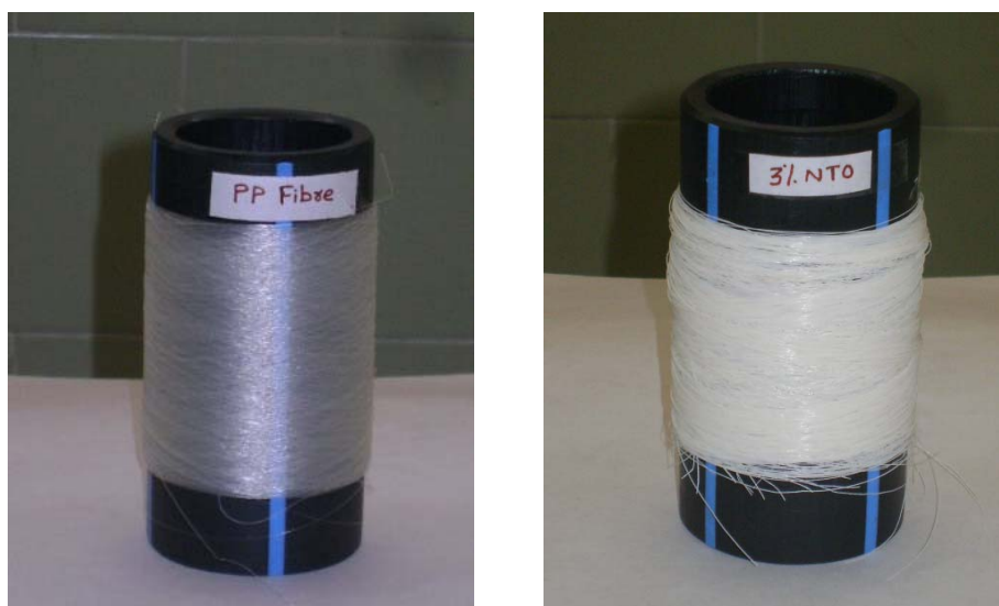
Figure 7.1: Photographs of neat PP fiber and \text{PP/TiO}_2 composite fibers
