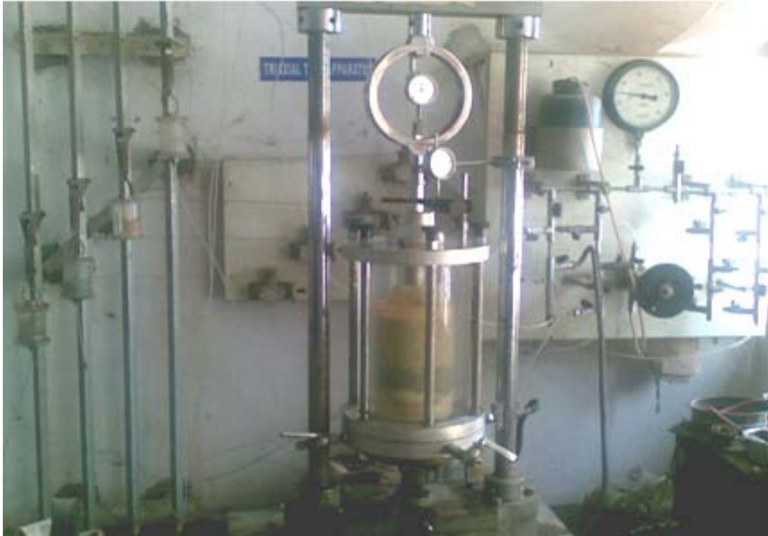
Fig. 7.4 Triaxial test set up
