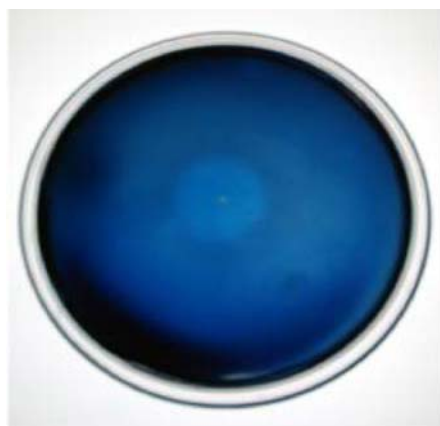
Fig. 2.7 PVA degrading isolate ( V.neries , strain BTKB4); Zone of clearance surrounding the colony in PVA agar plates after flooding with iodine -boric acid solution indicates PVA degradation
