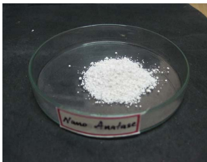
Fig. 3.3 TiO 2 nano particles obtained after calcinations at 400 0 C
