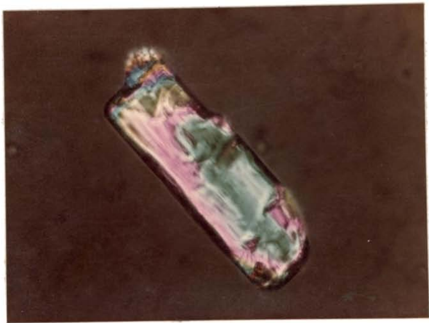
Plate32. Elongate prismatic grain of sillimanite
