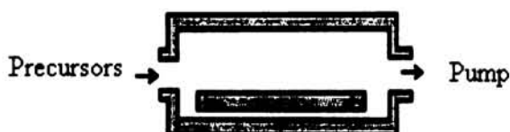
Figure 3.2: Thermal ALD reactor using cross flow concept.
