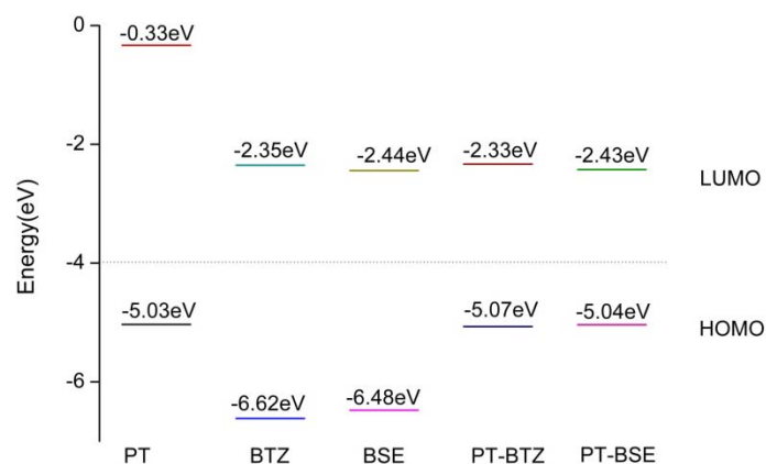
Figure 2: Energy levels of PT, BTZ, BSE, PT-BTZ and PT-BSE
