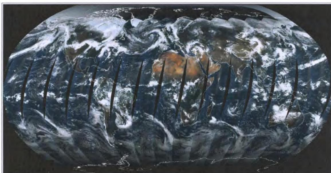
*Fig.2.1. True colour RGB image from MODIS sensor onboard Terra on April 19, 2000 showing its near daily global coverage capability.*
