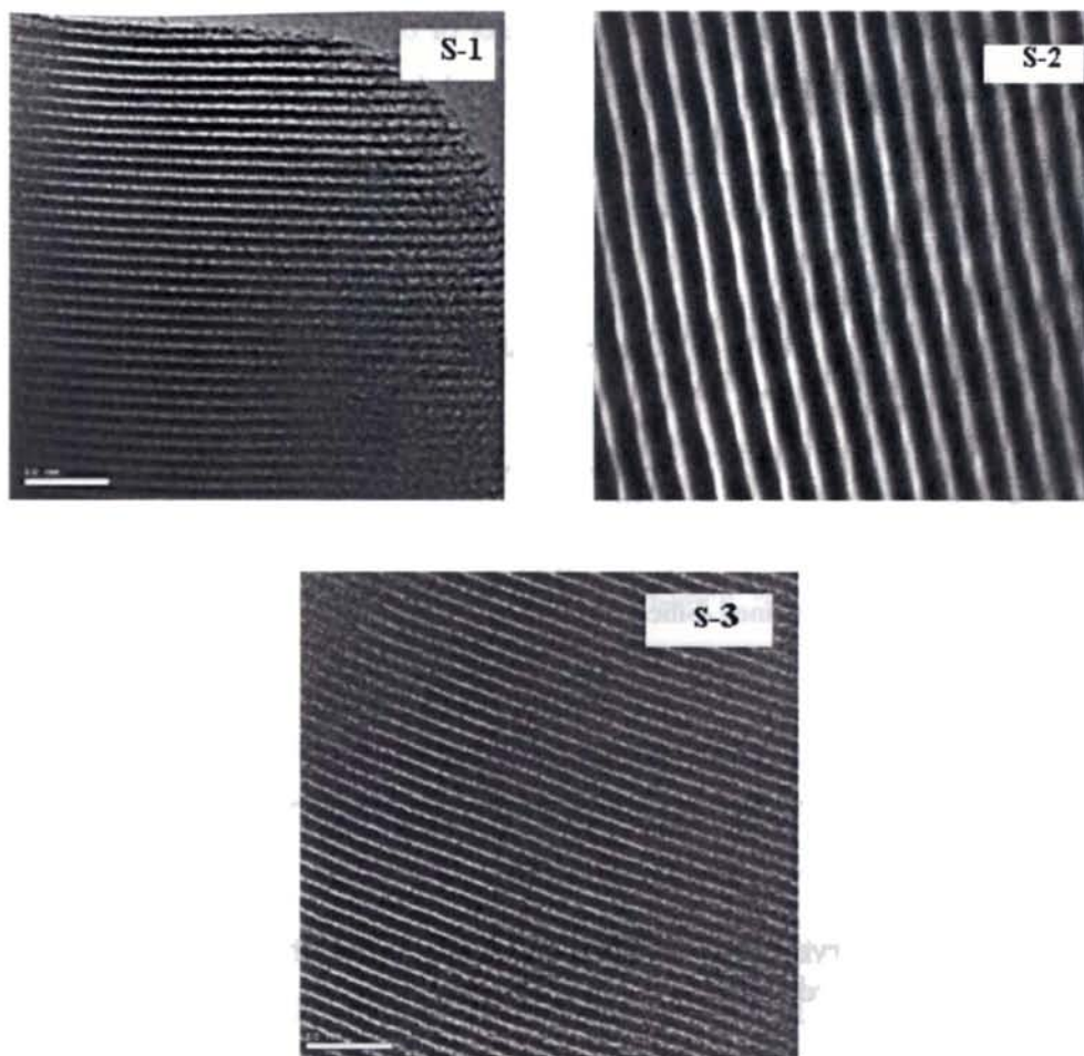
Fig 4.15 HRTEM of samples of various pore sizes taken vertical to the parallel channels
